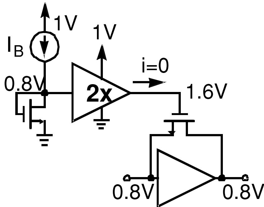
✓ Charge pump supplies no current, minimizing ripple
