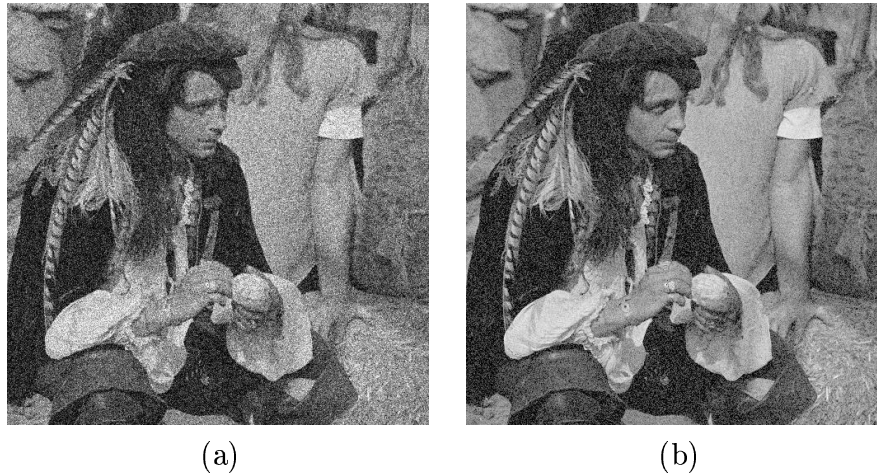
Figure 4.5: (a) Gaussian noise in light space is transformed to Gaussian noise in image space, if the CRF is linear. The second image (b) is the resultant noisy image corresponding to a nonlinear CRF. Light regions in (b) are less affected by noise due to the nonlinearity.
