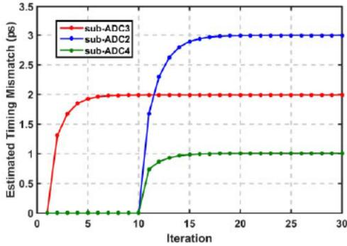
Fig. 5. Convergence of the estimated timing mismatch for a single-tone input at  $0.41f_s$  when  $\Delta T_{1-4}$  are set at [1, 4, 3, and 2 ps]. SNDR after calibration versus different  $N$  for 12-bit resolution.
