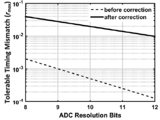
Fig. 2. Maximum tolerable timing mismatch versus resolution for 3-dB SNDR penalty in a four-channel TI-ADC before and after derivative-based digital correction ( $f_{in} = f_s/2$ ).
