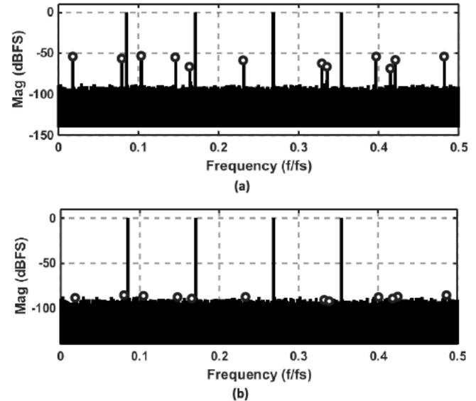
Fig. 10. Spectra of TI-ADC output for a multitone input. (a) Without and (b) with the proposed all-digital timing mismatch calibration.
