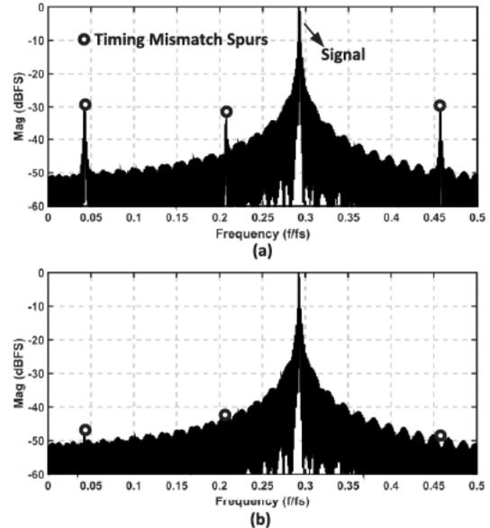
Fig. 9. Spectra of four-channel TI-ADC output for QPSK signal with a carrier frequency of  $0.29f_s$  and a symbol rate of 10 MHz. (a) Without and (b) with the proposed all-digital timing mismatch calibration.
