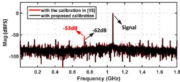
Fig. 16. Measured spectra of two-channel TI-ADC output for a single-tone input at 1065 MHz with the all-digital timing mismatch calibration in [17] and the proposed calibration. On-chip analog timing skew adjustment code is  $7b'0$ .
