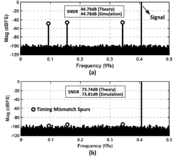
Fig. 6. Spectra of TI-ADC output for a single-tone input at  $0.41f_s$ . (a) Without and (b) with the proposed all-digital timing mismatch calibration. Theoretical results are computed from (9) and (13).
