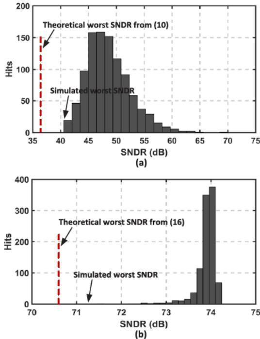
Fig. 8. Thousand times Monte-Carlo simulation of four-channel TI-ADC for Gaussian-distributed timing mismatch  $\Delta T_{1-4}$  ( $\sigma = 1$  ps). (a) Without and (b) with the proposed all-digital timing mismatch calibration. Theoretical worst SNDRs are calculated assuming  $r_{\max} = 6\sigma/T_s$ .
