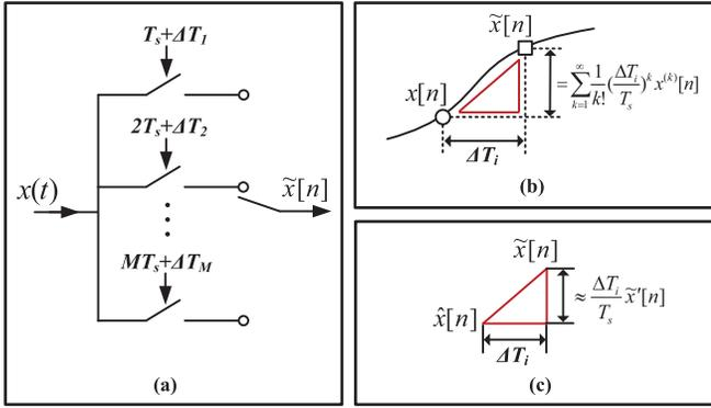
Fig. 1. Sampling diagram of a TI-ADC with timing mismatch. The number of sub-ADC channels is  $M$  and  $i = 1, 2, \dots, M$ . The sampling period of the TI-ADC is  $T_s$ , and the timing skew of the  $i$ th sub-ADC is  $\Delta T_i$ .  $x'[n]$  and  $x^{(k)}[n]$  represent the first-order derivative of  $\tilde{x}[n]$  and the  $k$ -order derivative of  $x[n]$ . (a)  $M$ -channel TI-ADC with timing mismatch. (b) Sampling in the  $i$ th sub-ADC. (c) Derivative-based correction.
