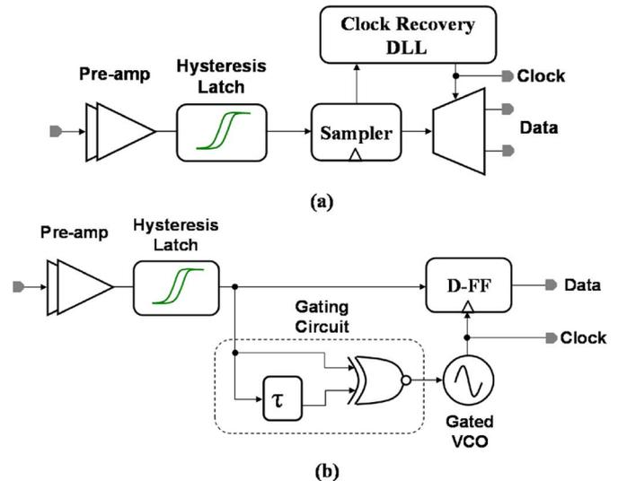
Fig. 11. AC coupled pulse receivers: (a) as in [1]; (b) as in [8].
