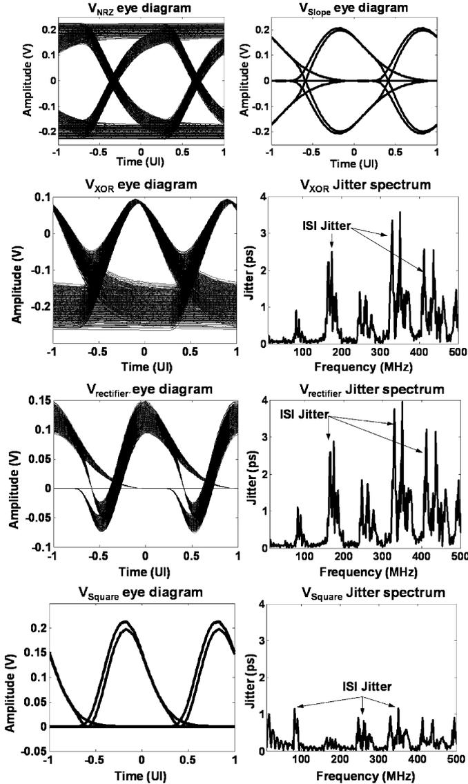
Fig. 14. Simulation results comparing different timing recovery schemes in both time and frequency domain at 10 Gb/s.
