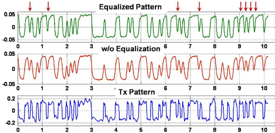
Fig. 10. Transmitted and recovered  $2^7 - 1$  sequence at 12 Gb/s with and without equalization captured by a pattern-locked oscilloscope. Arrows on the top indicate errors in the unequaled pattern which are corrected by equalization with the linear path.
