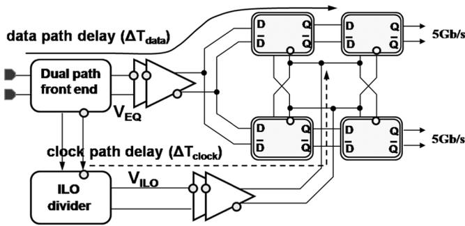
Fig. 20. Block diagram of the demux.
