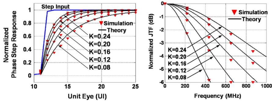
Fig. 22. Transient phase response and corresponding jitter transfer function for different injection strengths with  $n = 4$  stages, an oscillation frequency of 5 GHz and an injection frequency of 10 GHz.
