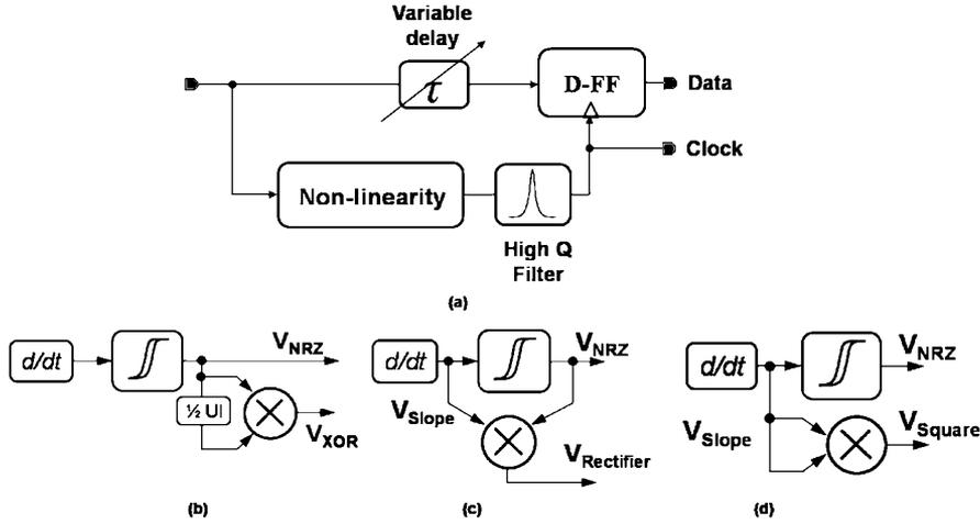
Fig. 13. Clock recovery with nonlinear spectral line method: (a) general block diagram; (b) as in [10]; (c) as in [17]; (d) this work.
