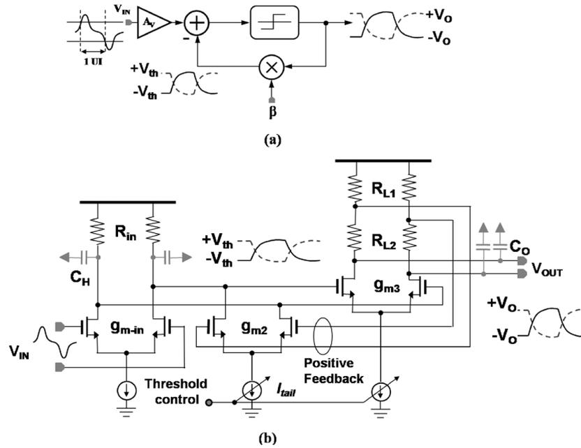
Fig. 4. Hysteresis latch topology for NRZ recovery: (a) NRZ recovery with DFE; (b) proposed Implementation.
