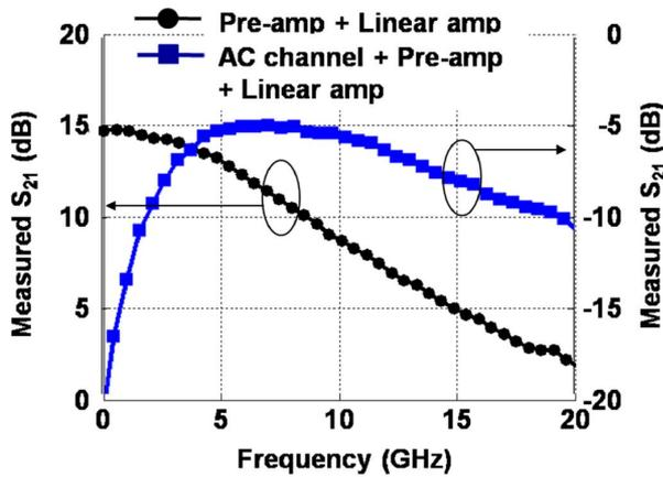
Fig. 7. Measured linear path response including and without the AC coupled channel.
