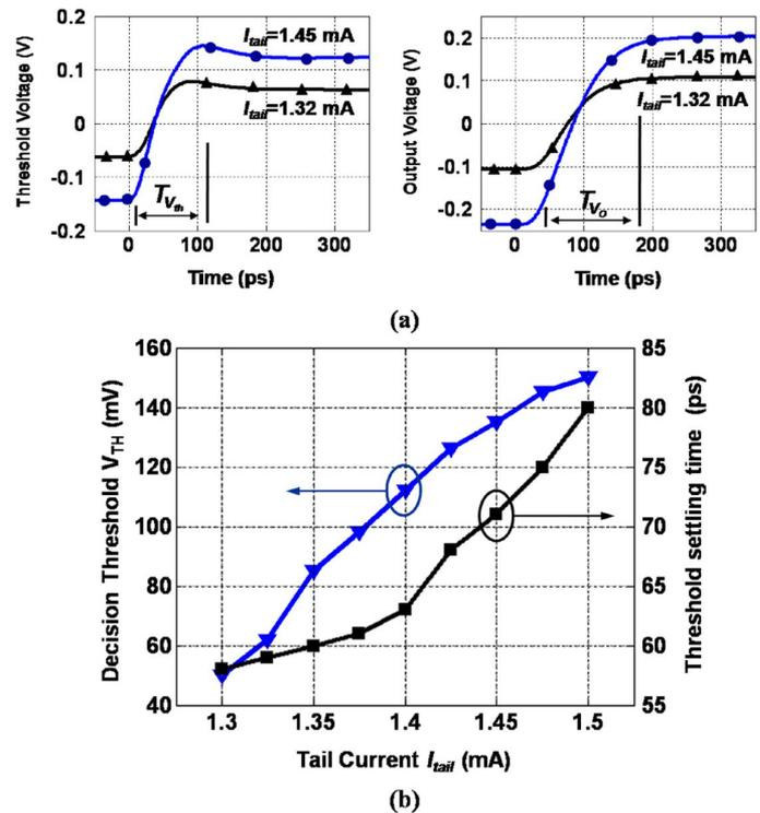
Fig. 5. Threshold adjustment with  $I_{tail}$  in the proposed hysteresis latch: (a) settling time of the decision threshold and output voltage; (b) variation of threshold voltage and settling time as a function of tail current.
