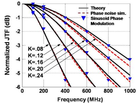
Fig. 21. Normalized jitter transfer function for different injection strengths with  $n = 4$  stages, an oscillation frequency of 5 GHz and an injection frequency of 10 GHz.
