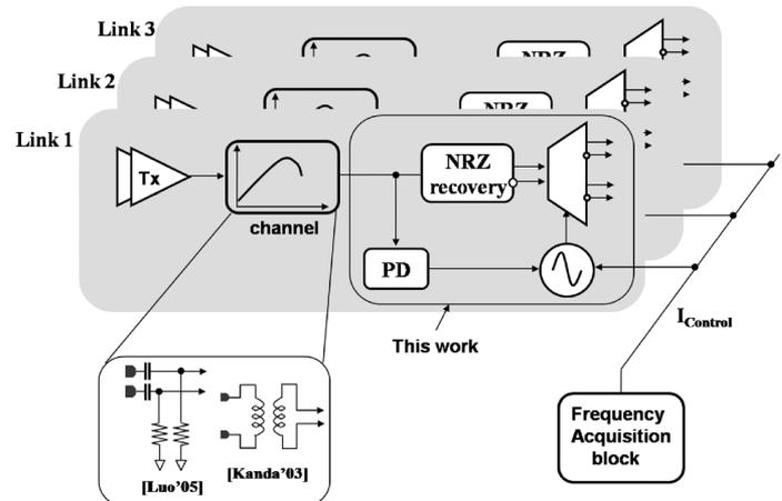
Fig. 1. AC coupled pulse transceivers for high density I/Os.
