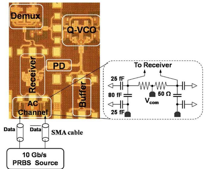
Fig. 23. Implemented complete receiver in 90 nm CMOS.
