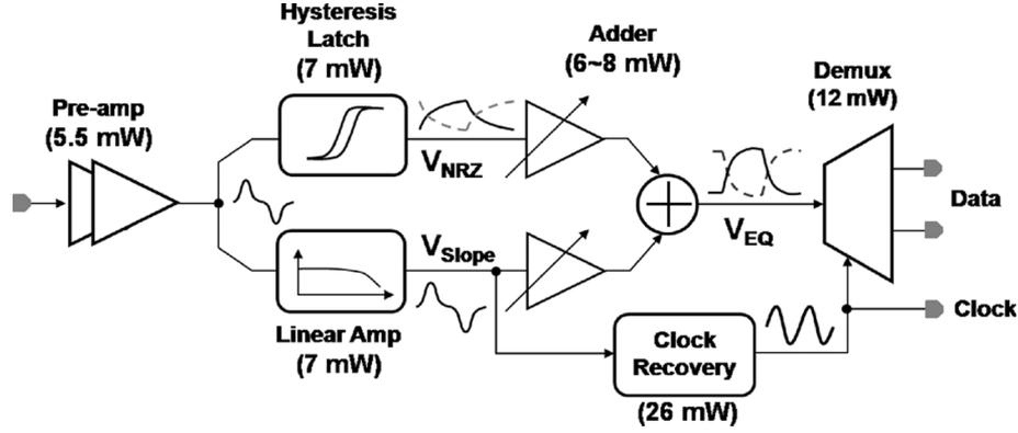
Fig. 12. Proposed dual path AC coupled pulse receiver with clock recovery using linear path.
