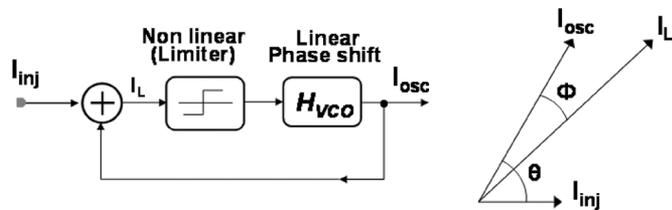
Fig. 17. Injection locked oscillator model and corresponding phasor diagram.
