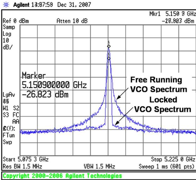
Fig. 25. Spectrum of the free running and recovered clock.
