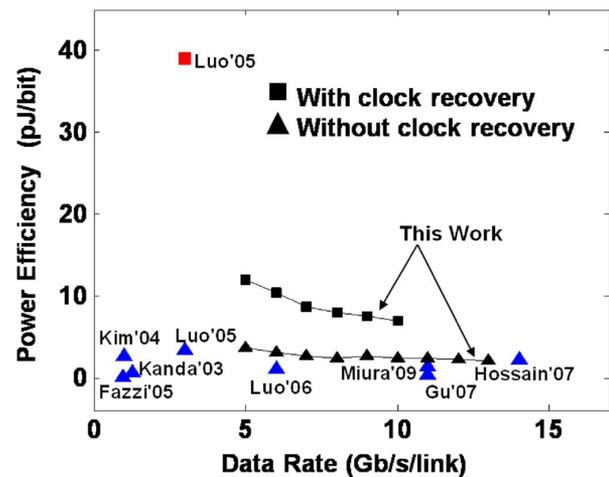
Fig. 2. Summary of existing AC coupled pulse receivers.
