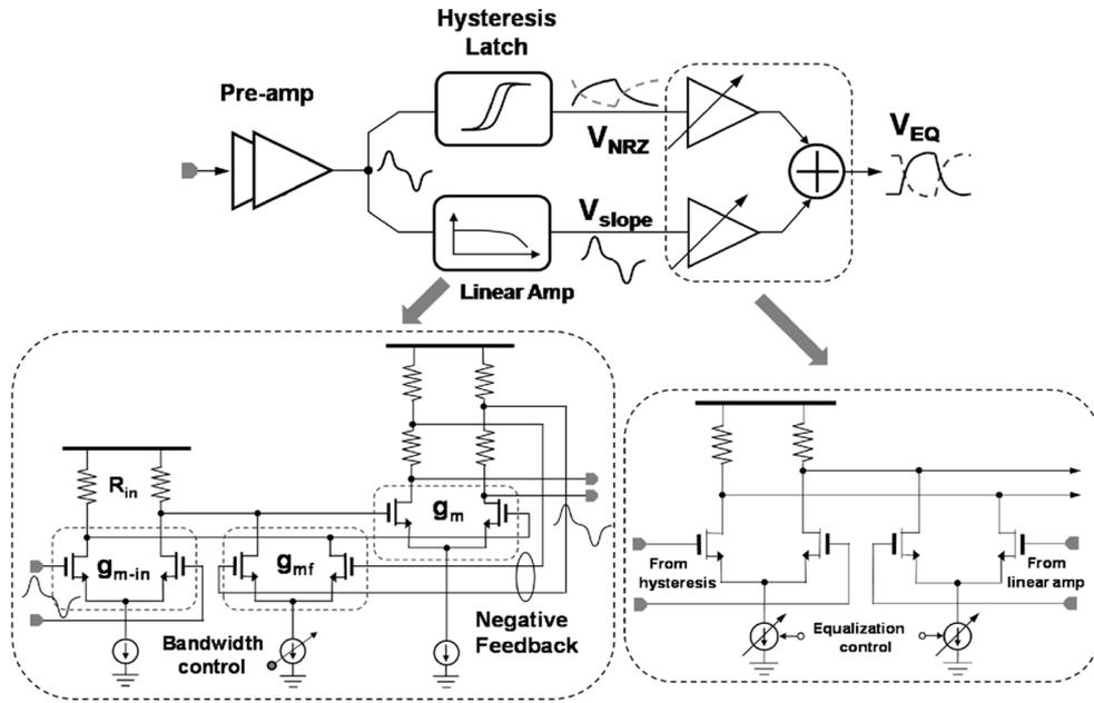
Fig. 6. Dual path receiver architecture with linear amplifier and analog adder.
