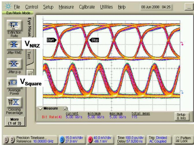
Fig. 16. Recovered NRZ signal and corresponding extracted clock tone at 5 Gb/s.
