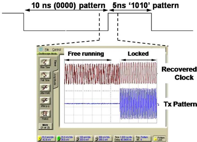
Fig. 28. Experimental verification of lock time.
