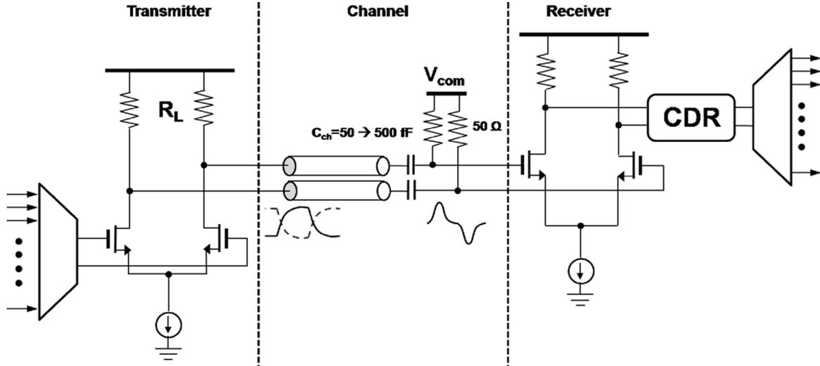
Fig. 3. Equivalent circuit of an AC coupled link including transmitter, channel and receiver.
