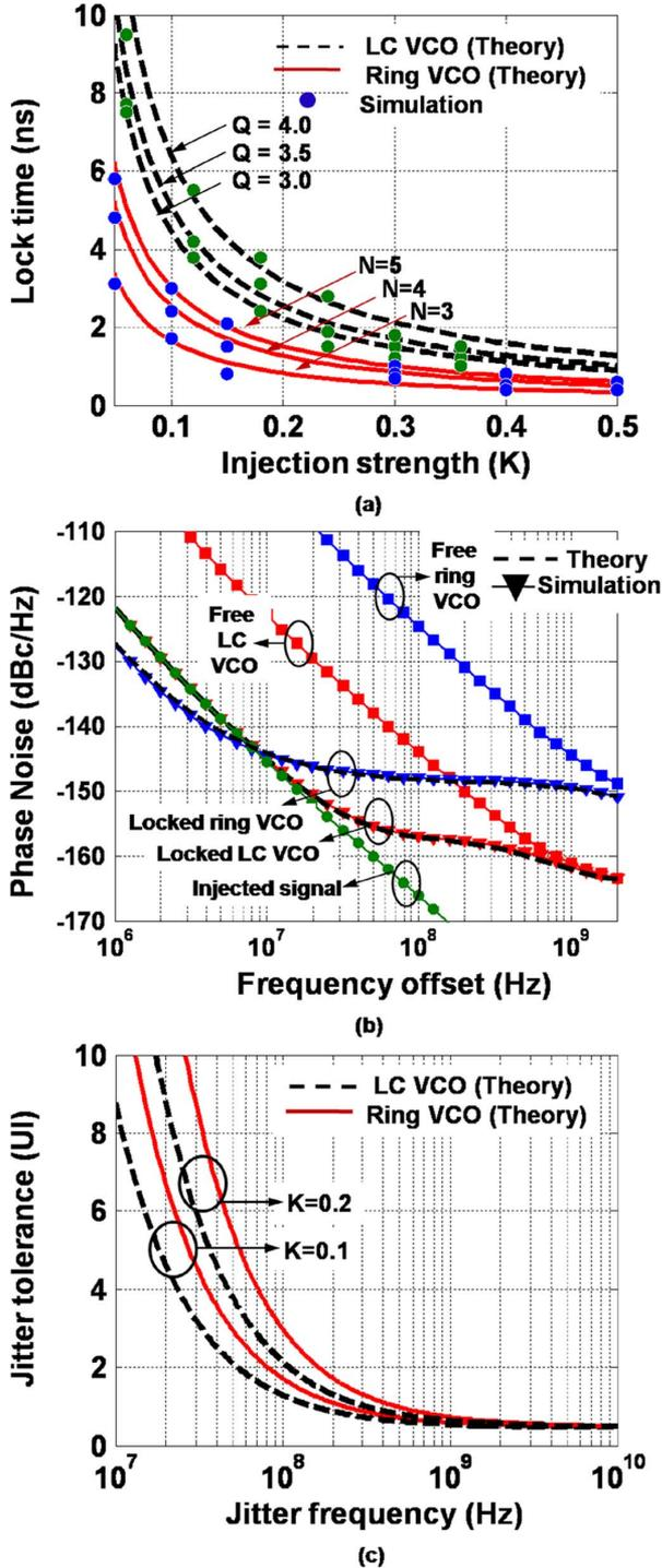
Fig. 18. Comparison of ILO performance for LC vs ring VCO. The LC VCO is operating at 10 GHz,  $Q = 3.5$ . The ring oscillator is operating at 5 GHz with  $n = 4$  stages: (a) lock time as a function of injection strength; (b) phase noise of the free running VCO and corresponding recovered clock; (c) jitter tolerance with a frequency offset,  $\Delta\omega = 2\pi \times 10^6$ .
