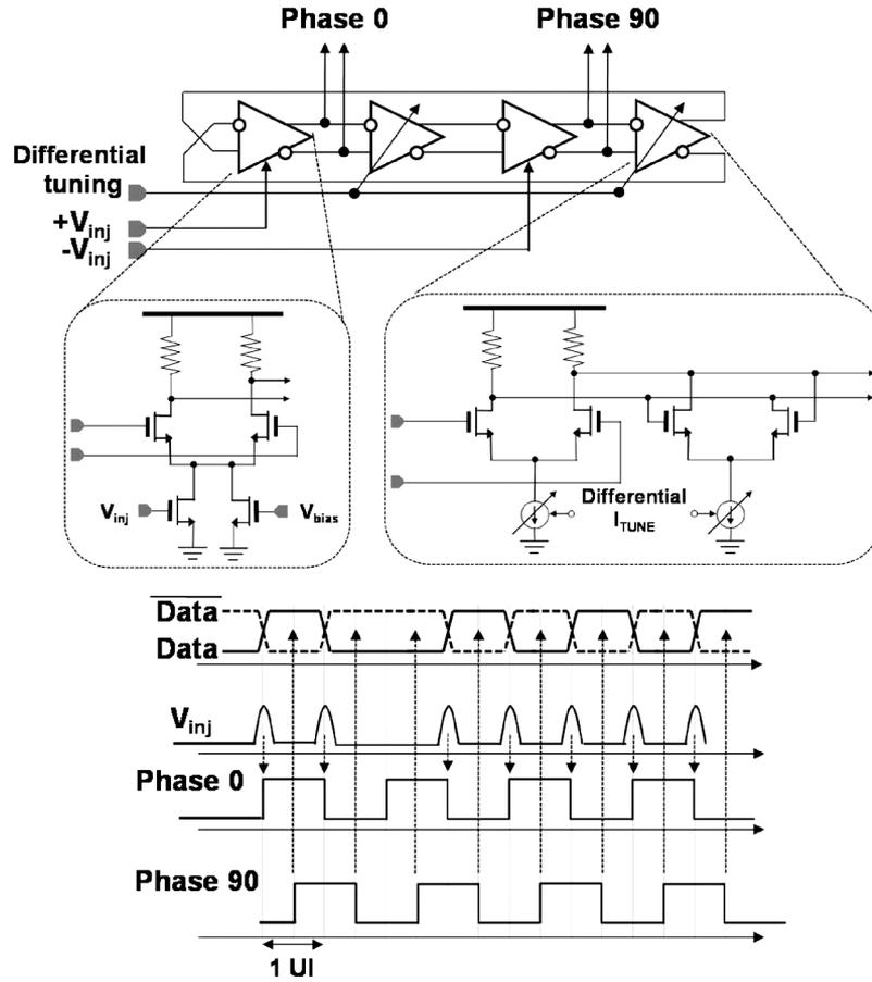
Fig. 19. Schematic of the ring oscillator based ILO and corresponding timing diagram.
