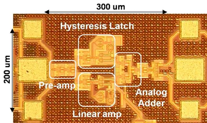
Fig. 8. Die photo of the dual path receiver in 90 nm CMOS.
