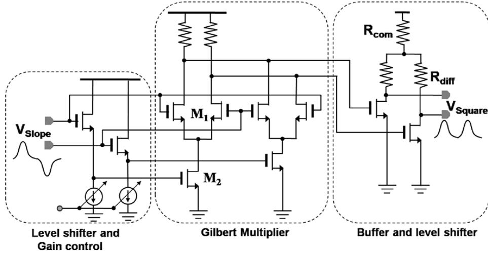
Fig. 15. Schematic of the Gilbert multiplier used for clock extraction.
