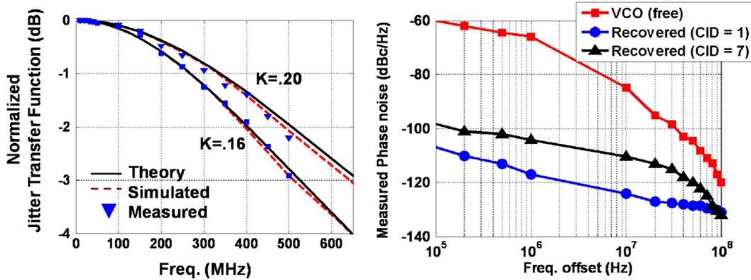
Fig. 27. Normalized jitter transfer function and phase noise of the recovered clock.
