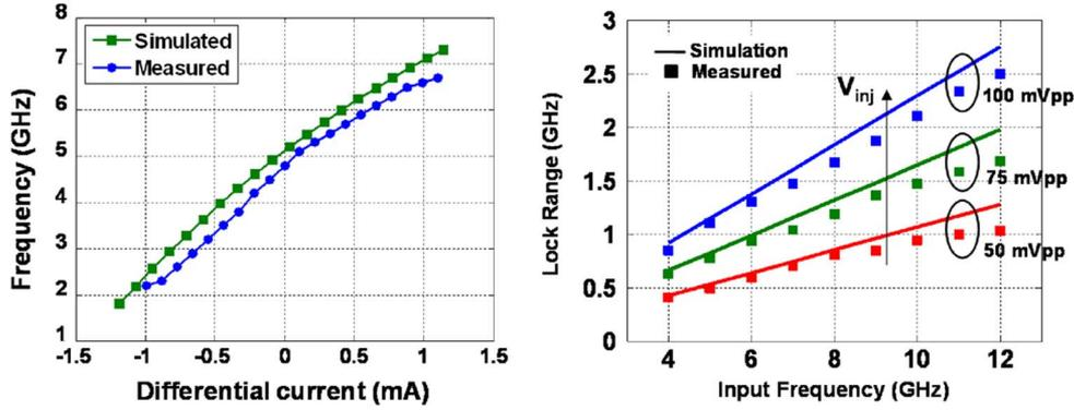
Fig. 24. Measured tuning range and lock range of the implemented 5 GHz 4 stage ring ILO.
