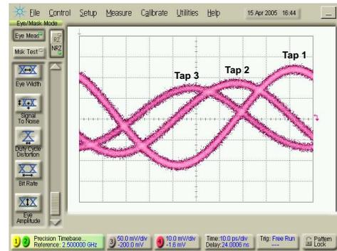
Fig. 6. Measured tap delays with a 200 mV peak-to-peak 10 GHz sinusoidal input.
