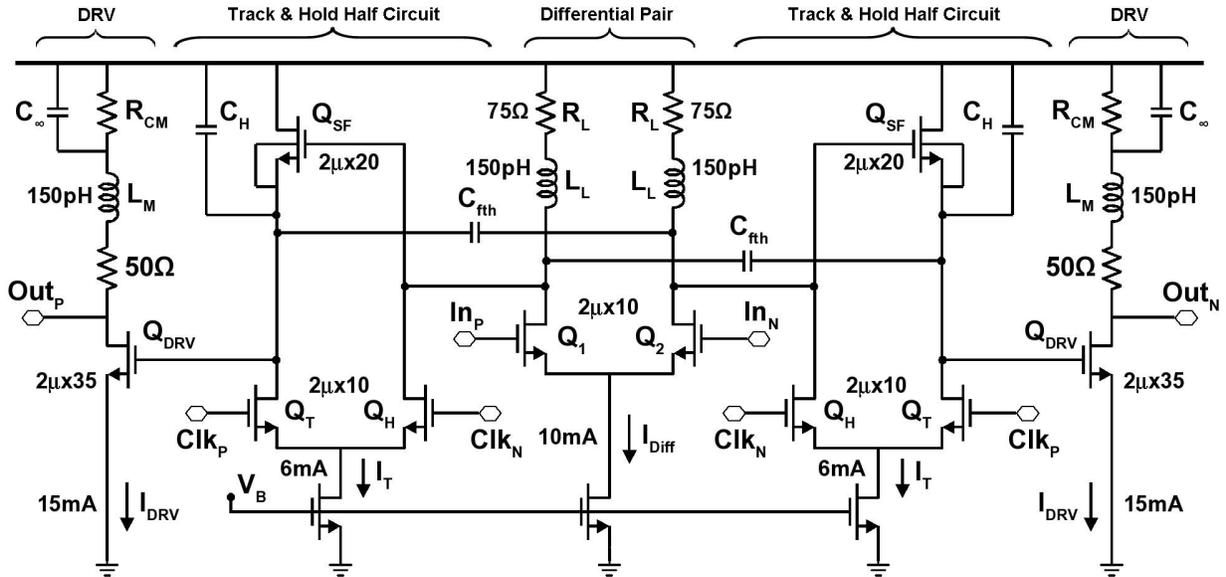
Fig. 3. Circuit diagram of the differential pair, T/H and output driver blocks. All MOSFETs have a drawn gate length of  $0.13\mu\text{m}$ .
