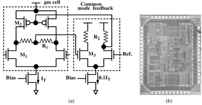
Fig. 5. Dual-function analog filter. (a) Schematic of transconductance cell. (b) Die photo.
