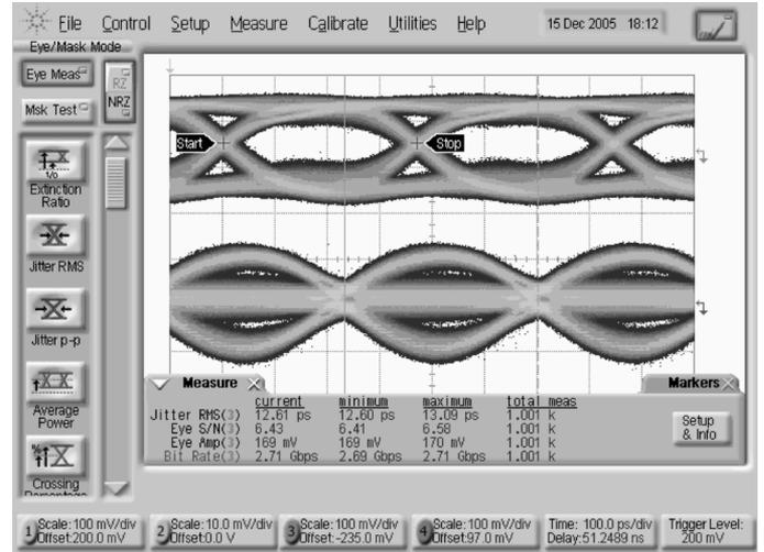
Fig. 7. Data (top eye) and slope (bottom eye) outputs of dual-function analog filter at 2.7-Gb/s (Vertical scale = 100 mv/div ; Horizontal scale = 200 ps/div).
