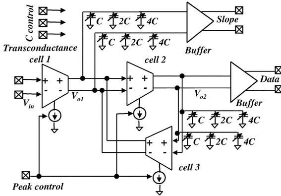
Fig. 4. Dual-function analog filter topology.
