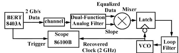
Fig. 8. Test set up for external TR loop using the dual-function analog filter.
