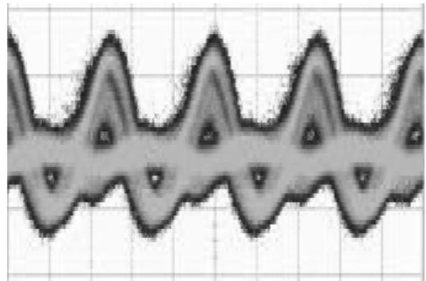
Fig. 9. Mixer output corresponding to a 2-Gb/s random data sequence ( Vertical scale = 20 mv/div ; Horizontal scale = 200 ps/div).
