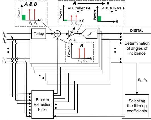
Fig. 1: Detection of the angles of incidence and the cancellation of the blockers.
