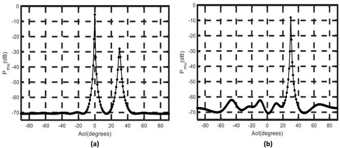
Fig. 10: MUSIC spectrum ( $P_{mu}$ ) (MUSIC algorithm output) (a) in the presence of the blocker and (b) after the blocker has been cancelled. Blocker is present at  $0^\circ$  and the desired signal at  $30^\circ$  AoI.
