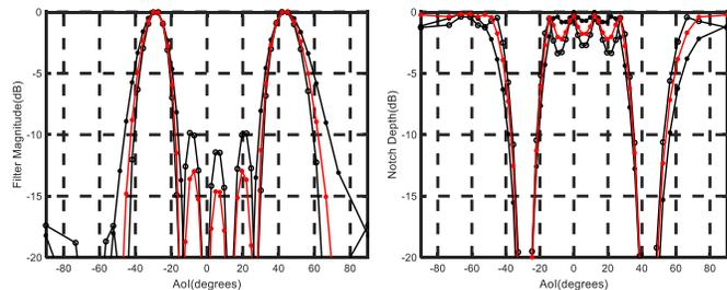
Fig. 7: Simulated blocker extraction filter and the resultant notch filter for blockers present at  $-30^\circ$  and  $45^\circ$  angle of incidences.
