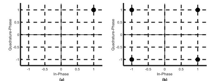
Fig. 11: Constellation diagram of the received QPSK signal (a) in the presence of the CW blocker (b) after the blocker is cancelled.
