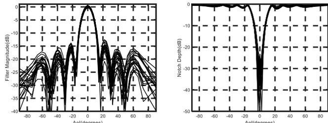
Fig. 8: Blocker extraction and notch filter for 5 percent mismatch in the gains of the amplifiers in the blocker cancellation filter.
