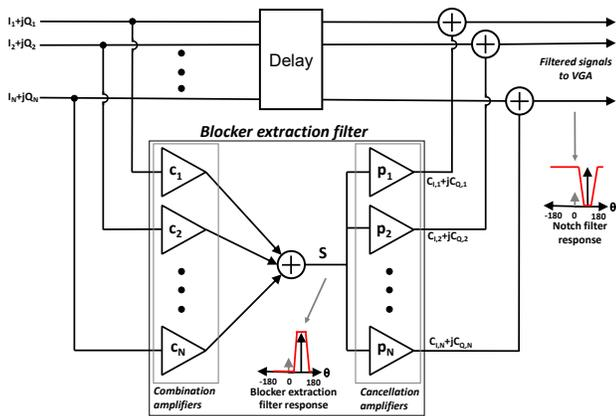
Fig. 2: Proposed filtering to extract and cancel the blocker signals.
