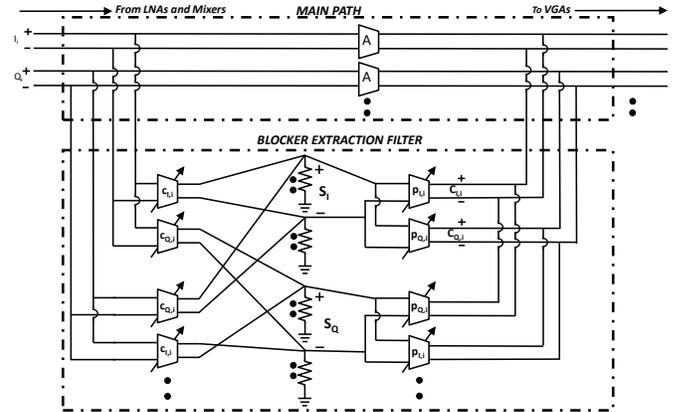
Fig. 5: Circuit level filter implementation.
