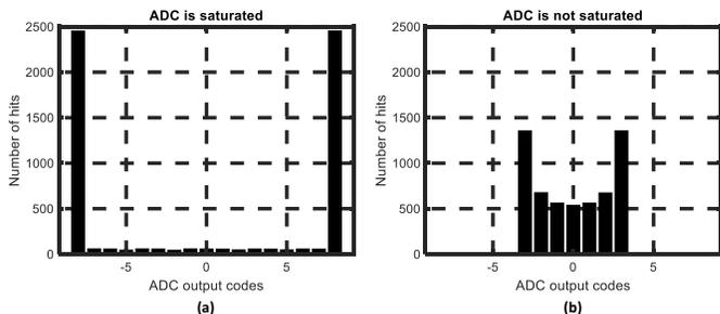
Fig. 9: Output codes of the ADC when (a) the ADC is saturated and (b) when the ADC comes out of saturation after the gain of the ADC is lowered.
