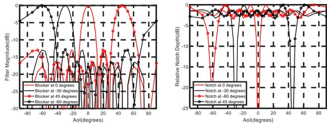
Fig. 6: Simulated blocker extraction filters and the resultant notch filters for different angles of incidences of the blockers.
