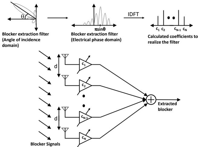
Fig. 3: Determination of filter coefficients for blocker extraction.
