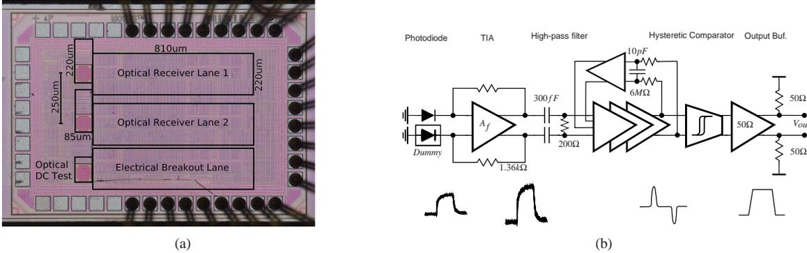
Fig. 1. (a) Photo of the die. (b) Receiver block diagram.
