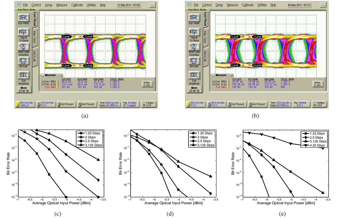
Fig. 2. Measurement results (a) Eye diagrams of an optical input with an average input power of -3.7dBm and an extinction ratio of 9dB and a supply of 1.2V and PRBS31 pattern at 2Gbps (b) PRBS7 pattern at 3.125Gbps. BER vs. average optical input for a constant 9dBm extinction ratio (c) 1.2V supply and PRBS31 input (d) 1.3V supply and PRBS31 input (e) 1.2V supply and PRBS7 input.
