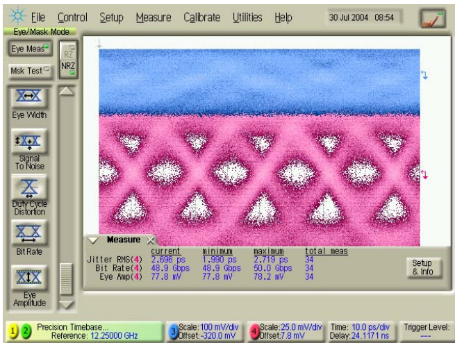
Figure 10. Measured 49 Gb/s (top) input after 9-ft SMA-cable and (bottom) equalized output eye diagram.
