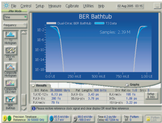
Fig. 14. Single-ended bathtub curve for single-ended output eye through 9-ft SMA cable at 39.5Gbps
