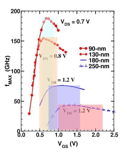
•Linearity depends on  $f_{MAX}(V_{GS})$  flatness at peak
