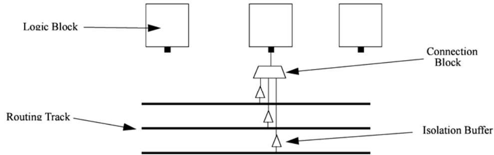
**Figure 8:** Routing track to logic block connection structure.
