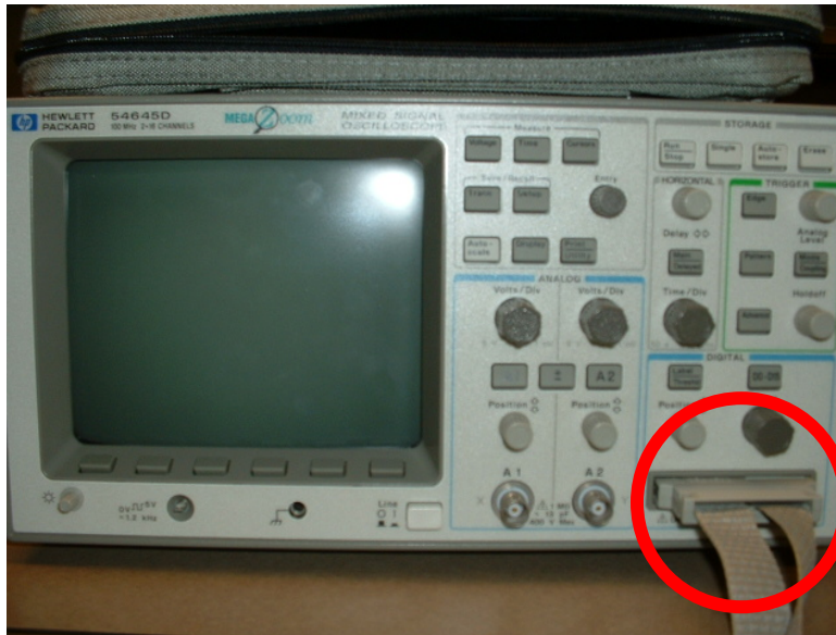
Figure 3 Illustration of the logic scope digital probe attachment.
