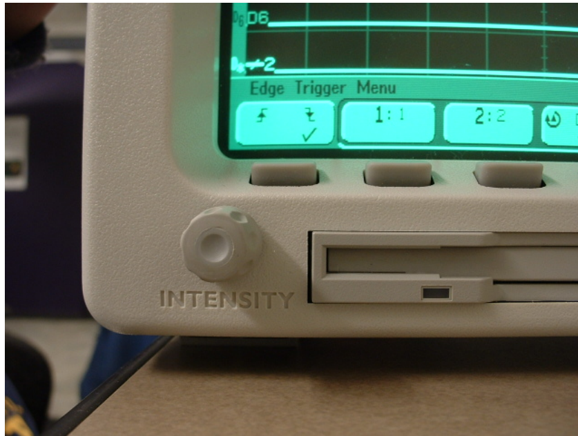
Figure 34 Falling edge selected as trigger pattern.
