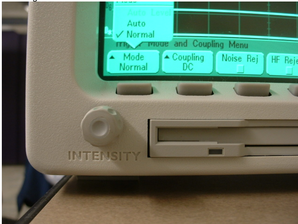
Figure 31 Setting the Agilent scope to "Normal" mode
