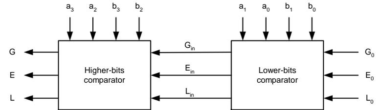
(a) [2] For what values of the inputs  $A$  and  $B$  will the result of the lower-bits comparator ( $G_{in}$ ,  $E_{in}$  and  $L_{in}$ ) influence the overall outputs  $G$ ,  $E$  and  $L$ ? Explain. Your answer *should not* give every possible input combination – you must express your answer by stating relationships between the input values of the  $a_i$ ,  $b_i$ ,  $G_{in}$ ,  $E_{in}$  and  $L_{in}$ .
