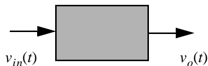
Figure 5.1: A single-input single-output system.
