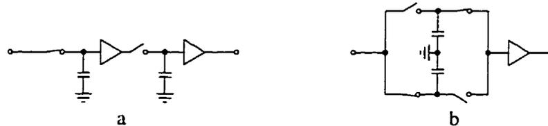
Figure 5.4: Two-stage S/H, a. master-slave, b. ping-pong.
