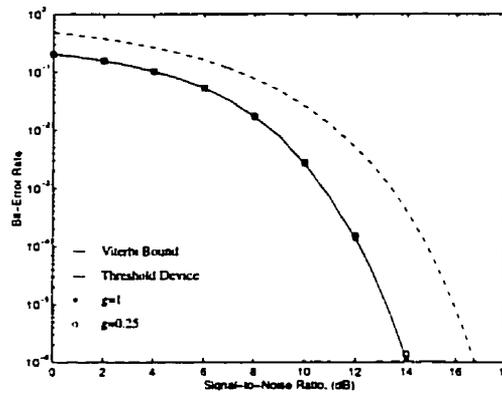
Figure 5.15: Effect of the non-ideal  $i - v$  characteristics of the diodes on the performance of the dicode decoder for two branch gains.
