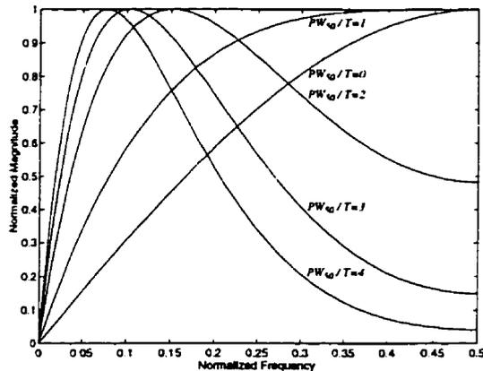
Figure 2.15: Pulse-response spectra of a Lorentzian magnetic channel.
