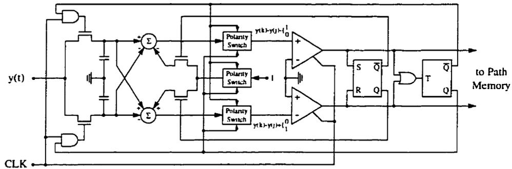
Figure 4.6: Block-diagram realization of the input-interleaved Viterbi detector (the input-interleaved architecture).
