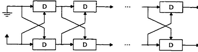
Figure 4.4: The decoder path memory based on the register-exchange method.
