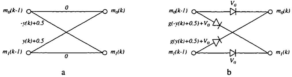
Figure 5.12: A dicode trellis diagram (a), and its corresponding diode network (b).
