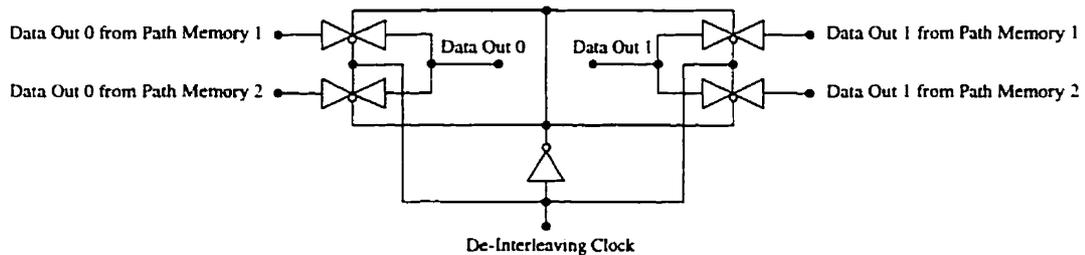
Figure 4.24: The de-interleaving multiplexers.
