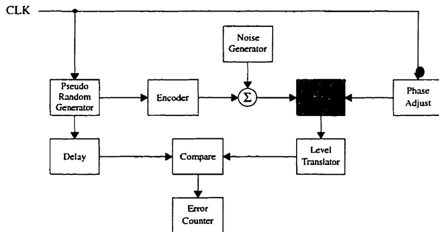
Figure 4.30: The experimental setup used to measure the BER of the decoder. The decoder is shown as the device under test (DUT).
