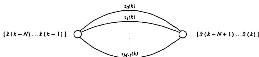
Figure 6.1: The trellis diagram of a one-state sequence detector. The branch labels are the inputs leading to the corresponding transitions.
