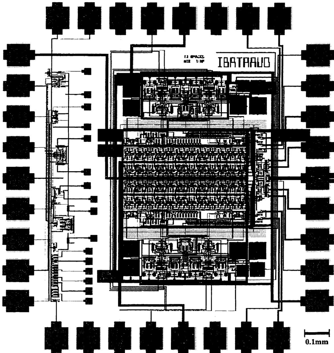
Figure 4.32: Layout of the class-IV analog Viterbi decoder, fabricated in the  $0.8\mu\text{m}$  NT BiCMOS process (BATMOS).
