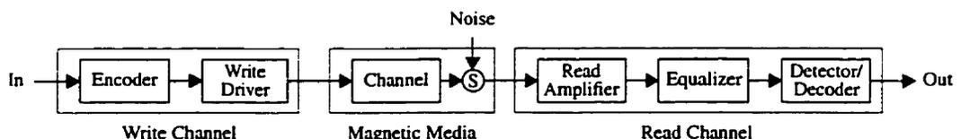
Figure 2.12: A typical magnetic data-storage system.
