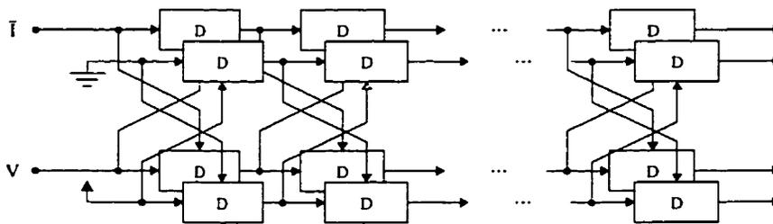
Figure 6.14: Path memory of the reduced-state quaternary decoder.
