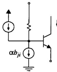
Figure 5.9: Reducing the DC threshold of the diodes by partially (entirely) bypassing the DC components of the error signals.
