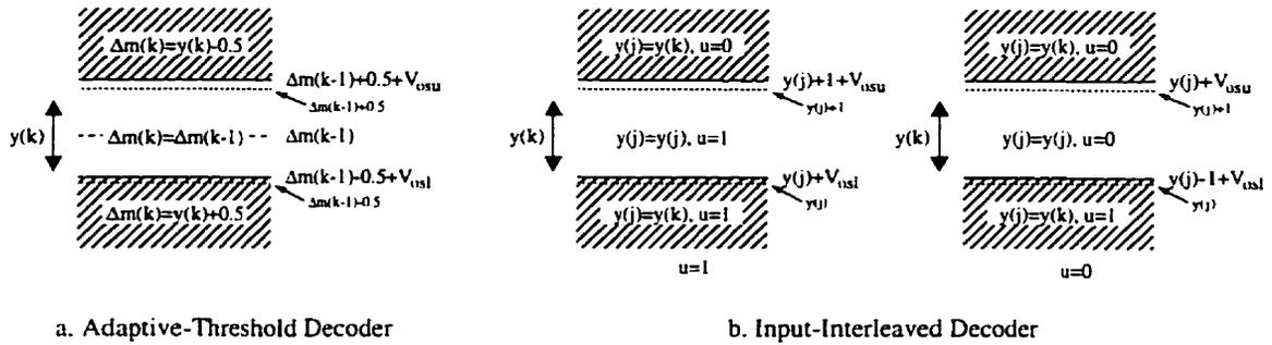
Figure 4.7: Effects of comparator offsets on the threshold levels of the decoders (Figures 4.1.a and 4.5).
