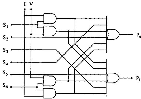
Figure 6.10: A typical combinational circuit for generating signals which set the polarity of the input signal in constructing the upper and lower threshold levels.
