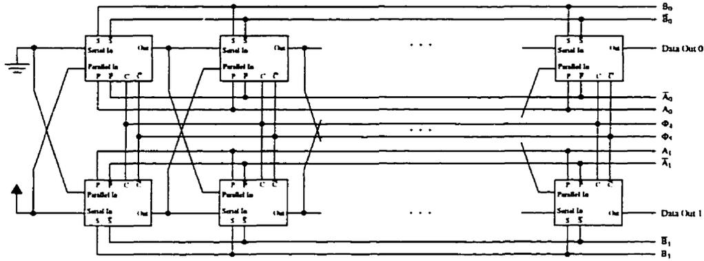
Figure 4.19: Path memory implementation using multiplexed-input D flip-flops.
