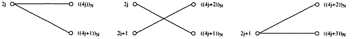
Figure 6.3: Survivor extensions in the binary PRS two-state RSSD, starting from states  $2j$  and  $2j+1$ , and assuming  $f_1 > 0$ .
