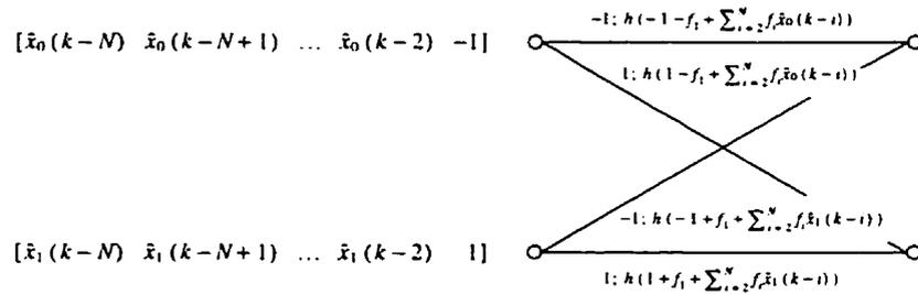
Figure 6.2: Two-state trellis of a binary-PRS system resulted from grouping even and odd states. The branch labels show the pairs of normalized *decoded; encoded* signals.
