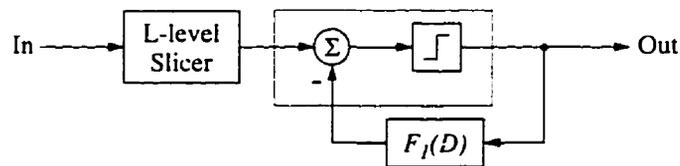
Figure 2.11: An alternative to the conventional DFE-based symbol-by-symbol PRS detector.
