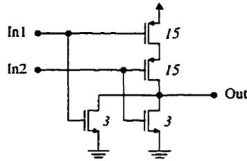
Figure 5.22: The schematic of the NOR gate used in the clock generator circuit.
