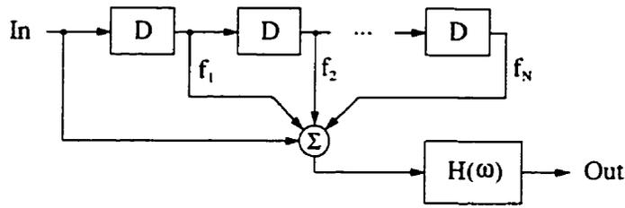
Figure 2.1: A partial-response encoder model.
