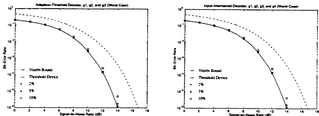
Figure 4.13: Worst-case performance degradation when all of the mismatches are present.
