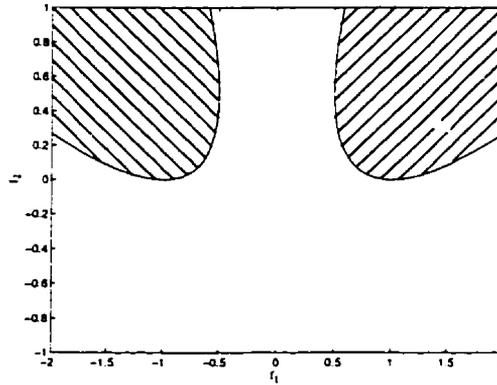
Figure 3.10: The region in the  $f_1 - f_2$  plane in which the PR code is a maximal-distance code (unshaded area).
