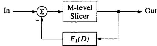
Figure 2.8: Symbol-by-symbol PRS detector based on a DFE.
