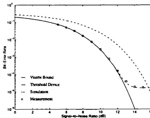
Figure 5.23: Measured BER performance of the dicode decoder at  $50\text{Mb/s}$ . Note that a relatively-short path memory with the local-optimum track-back method has been used.
