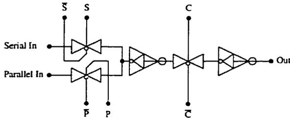
Figure 4.18: Multiplexed-input D flip-flop used to implement the path memory. Two small feedback inverters are shown inside the feed-forward inverters.
