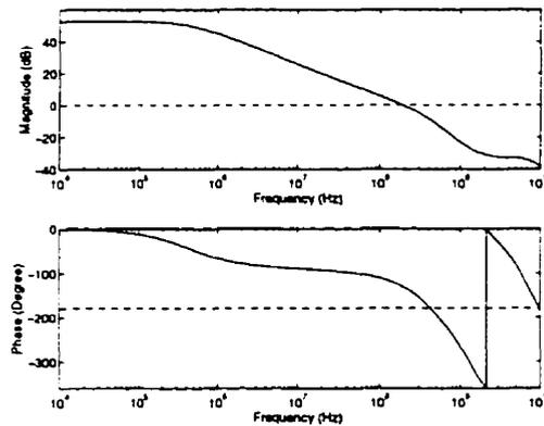
Figure 5.17: Bode plot of the CMFB circuit in the binary dicode decoder obtained by SPICE.
