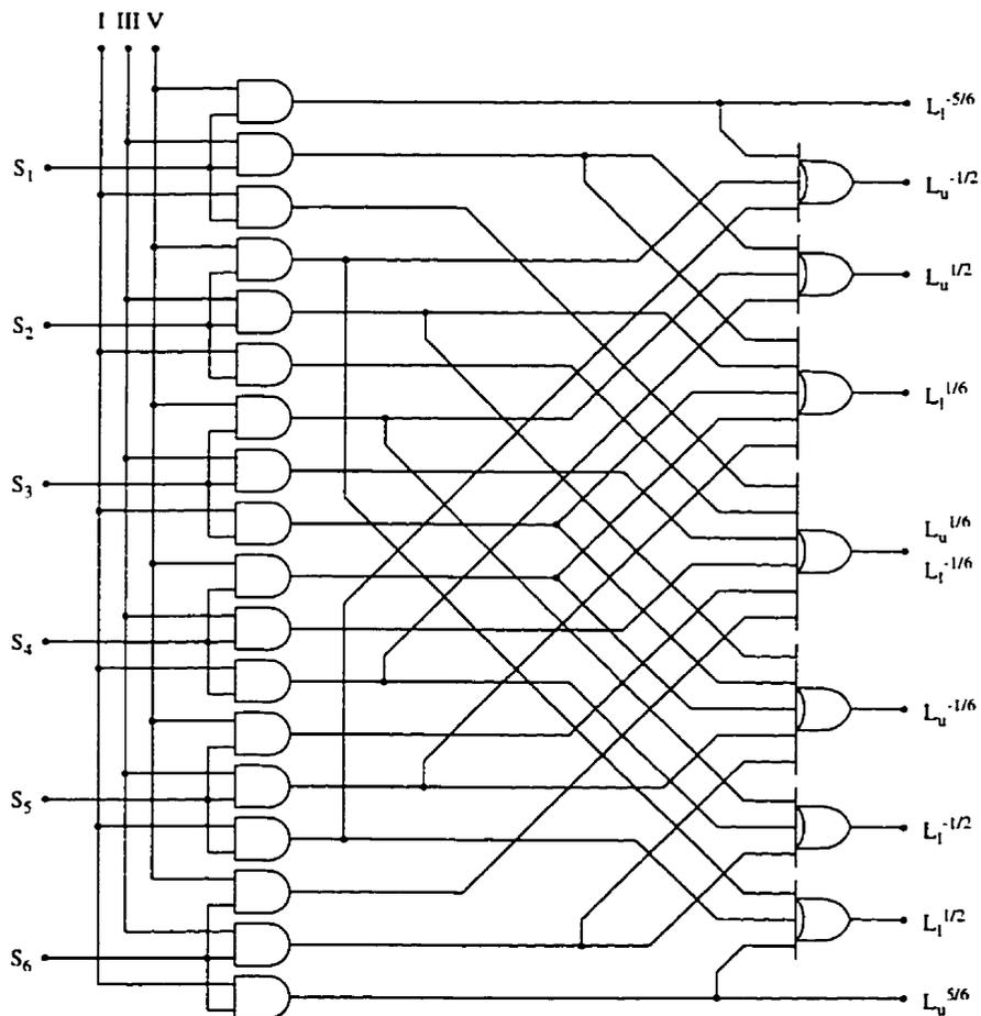
Figure 6.11: A typical combinational circuit for generating signals which set the DC values in constructing the upper and lower threshold levels.
