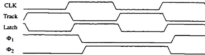
Figure 5.10: A typical timing diagram for the clock generator.
