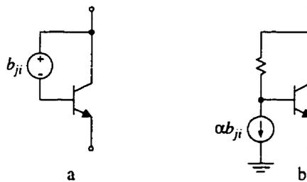
Figure 5.3: Threshold-programmable diode.
