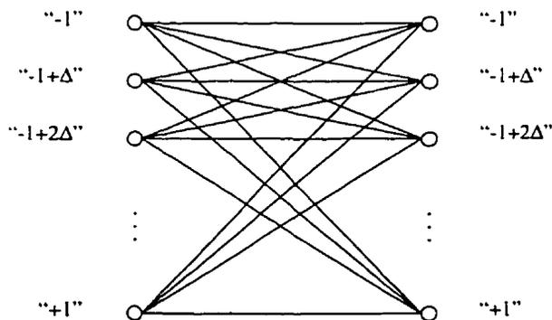
Figure 3.7: Trellis diagram of an  $M$ -ary first-order PRS scheme.
