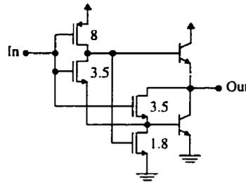
Figure 4.26: BiCMOS inverter capable of driving the output transistors of the buffer circuit as well as the pad.
