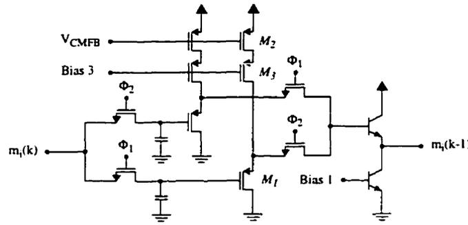
Figure 5.6: The ping-pong S/H circuit. Input and output are the new and previous state metrics of state  $i$ .
