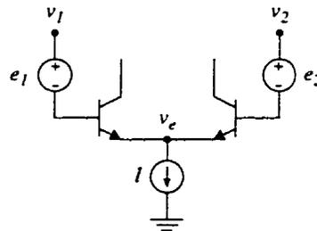
Figure 5.14: The generic circuit for generating the new state metrics.
