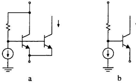
Figure 5.5: Sensing the current of a programmable diode by a. employing a mirror transistor and b. directing the collector current.
