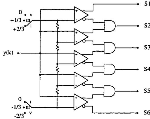
Figure 6.9: Slicing the input signal with five comparators and by making use of the previous state estimates.
