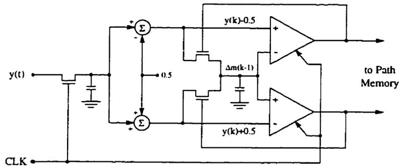
Figure 4.3: Block-diagram realization of the adaptive-threshold Viterbi detector for decoding a dicode signal (the adaptive-threshold architecture).
