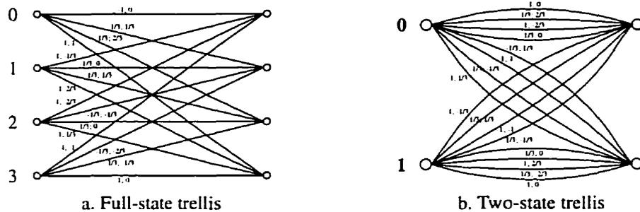
Figure 6.6: Full-state and two-state trellis diagrams of the quaternary dicode scheme. Branch labels represent the pairs of the normalized *uncoded; encoded* signals.
