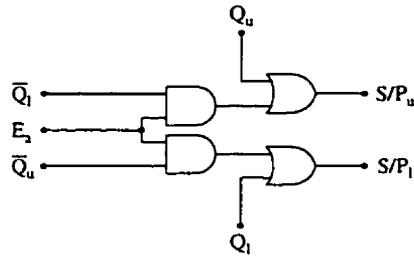
Figure 6.15: Generating signals for updating the path memory. Each signal controls the serial/parallel loading of its corresponding shift register. A “1” corresponds to a serial shift and a “0” to a parallel load.
