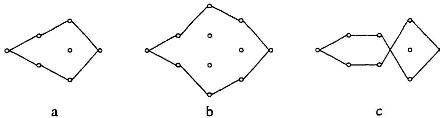
Figure 3.9: Different error events in a second order PRS-MLSD detector for calculating  $d_{min}$ .
