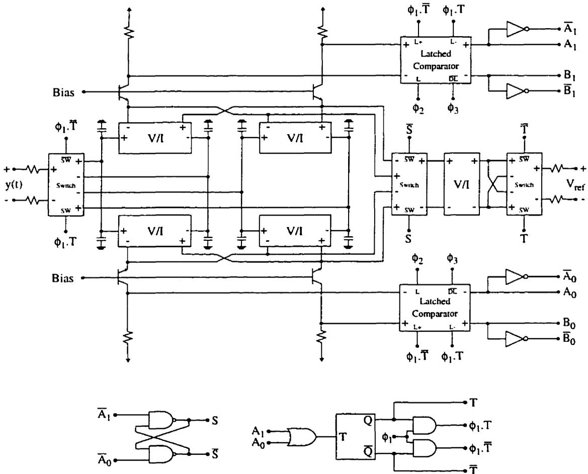
Figure 4.14: Circuit realization of the input-interleaved Viterbi detector.
