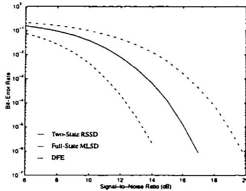
Figure 6.5: Noise performances of the MLSD and RSSD applied to the binary-EPR4 scheme.
