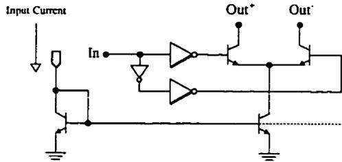
Figure 4.25: Open-collector output buffer.
