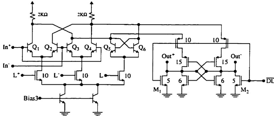
Figure 4.17: The latched-comparator circuit.
