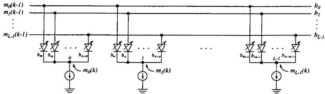
Figure 5.2: The diode network used to realize the ACS function.
