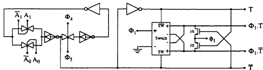
Figure 4.20: Circuit implementation of the T flip-flop and required gates shown in figure 4.14.
