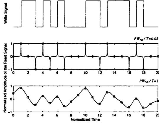
Figure 2.14: Typical write and read signals for low and high densities.
