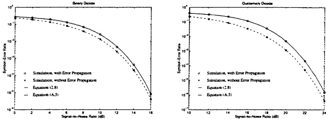
Figure 2.10: Noise performances of binary and quaternary dicode PRS schemes with DFE detectors.
