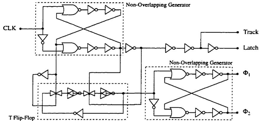
Figure 5.11: The clock generator circuit.
