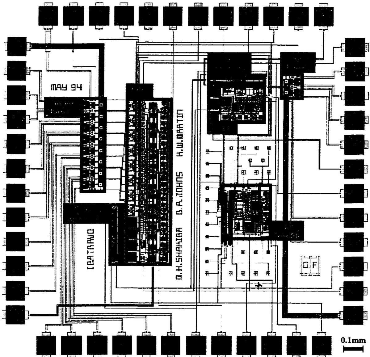
Figure 5.24: Layout of the dicode and EPR4 analog Viterbi decoders. A test dicode with test pads connected to some critical nodes is included in this layout as well.
