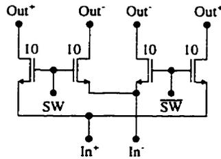
Figure 4.15: The differential dual switch used in figure 4.14.
