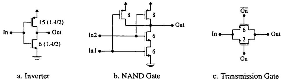
Figure 4.27: CMOS gates used in the decoder. The values inside brackets show the transistor sizes of the small feedback inverters in figure 4.18.
