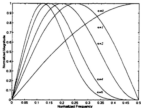
Figure 2.16: Output signal spectra of the EPR systems.
