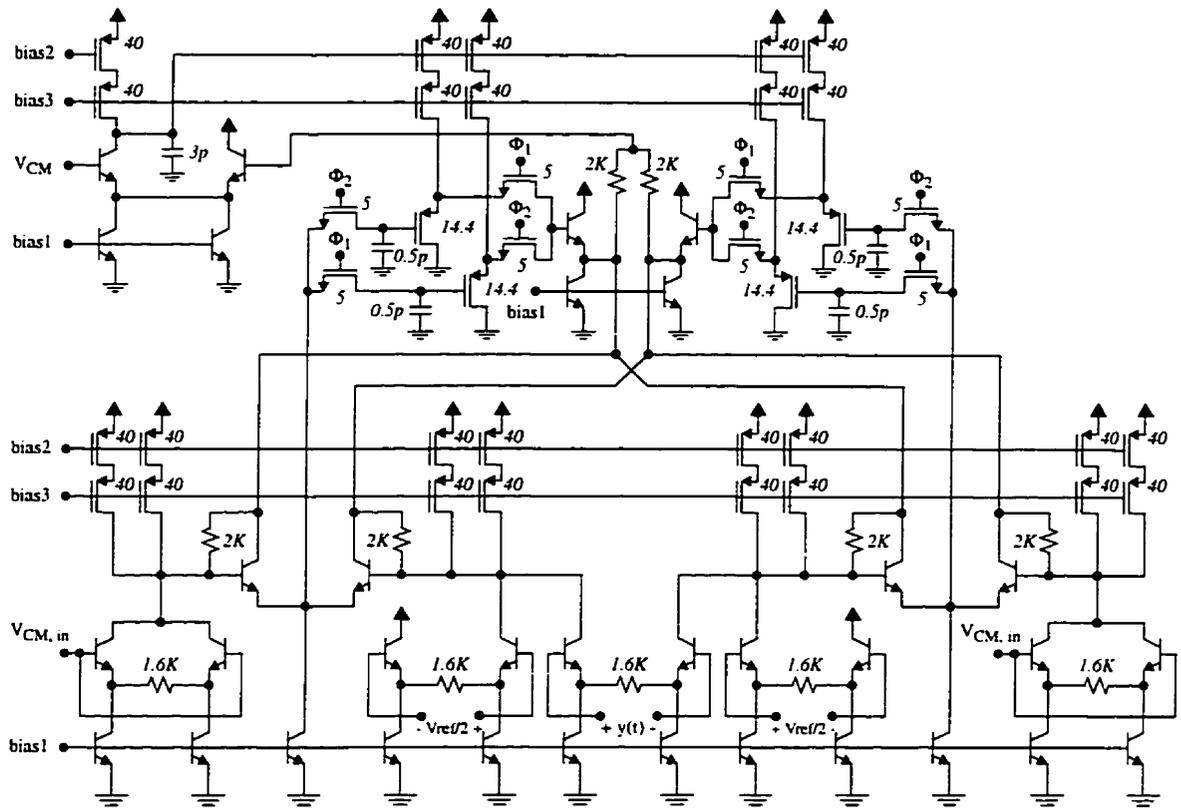
Figure 5.13: The binary dicode decoder.
