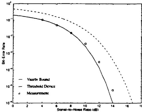
Figure 4.28: Measured BER performance of the discrete-prototype adaptive-threshold decoder.
