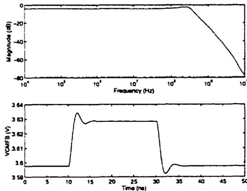
Figure 5.18: Frequency and time domain SPICE simulation results of the actual CMFB circuit.
