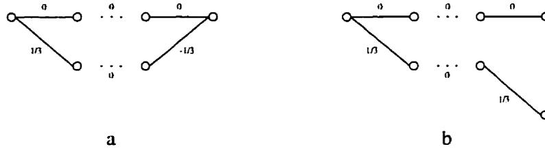
Figure 6.17: Minimum-distance error events in the full-state (a) and reduced-state (a and b) quaternary-dicode decoders.
