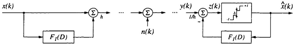
Figure 2.9: PRS-system model for noise-performance analysis.
