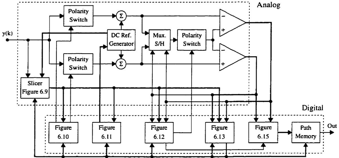
Figure 6.16: Circuit-level block diagram of the analog quaternary dicode decoder. Bold lines indicate multi-signal connections.
