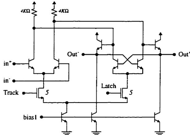
Figure 5.19: The latched-comparator circuit.
