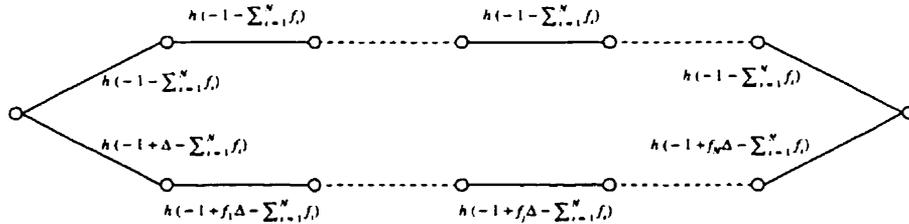
Figure 3.6: The minimum-length error event in a PR-MLSD decoder.
