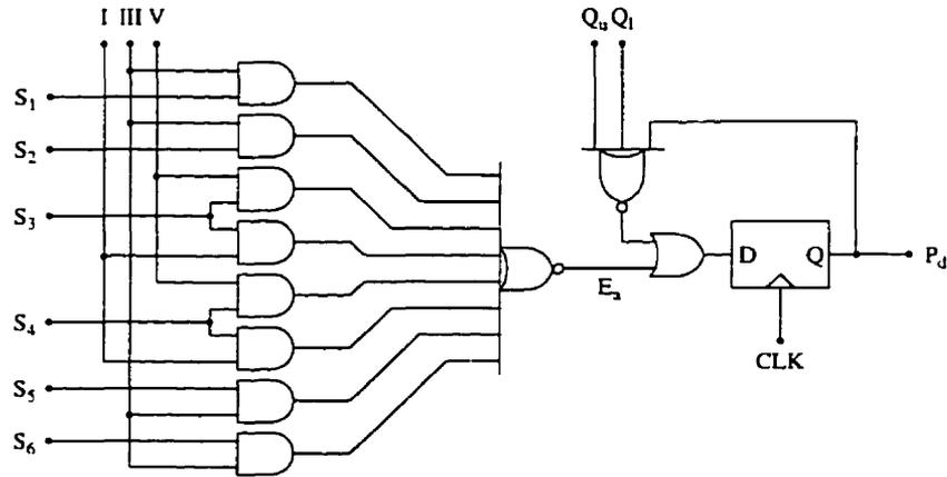
Figure 6.12: Generating the control signal which sets the polarity of the difference-metric signal. A "1" at the output corresponds to a positive polarity and a "0" to a negative polarity. AND gates are redrawn from figure 6.11.
