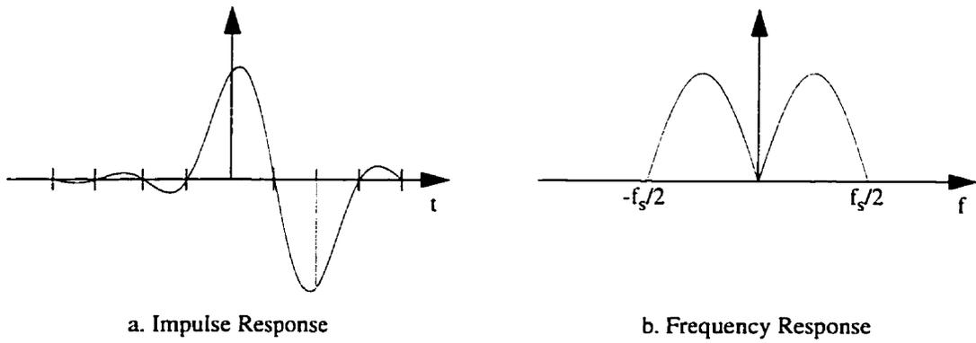
Figure 2.6: The class-IV (PR4) system.
