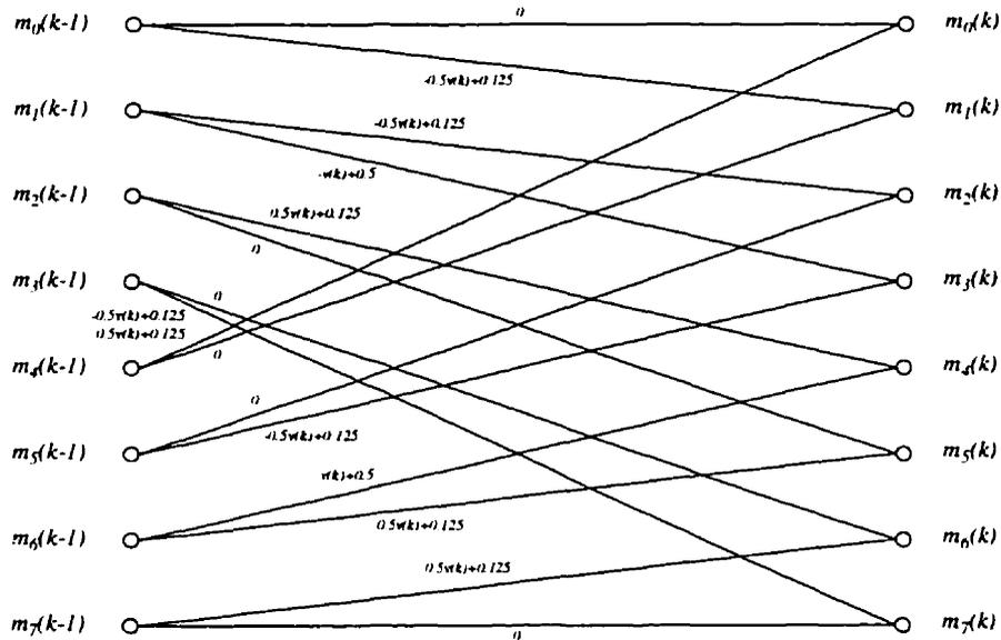
Figure 5.20: The trellis diagram of the binary EPR4 signaling scheme.
