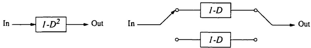
Figure 2.7: The class-IV system and its time-interleaved structure.
