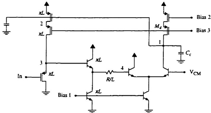
Figure 5.8: The equivalent circuit for analyzing the CMFB in presence of a change in the CM signal.
