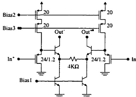
Figure 4.16: Circuit realization of the  $V/I$  block.
