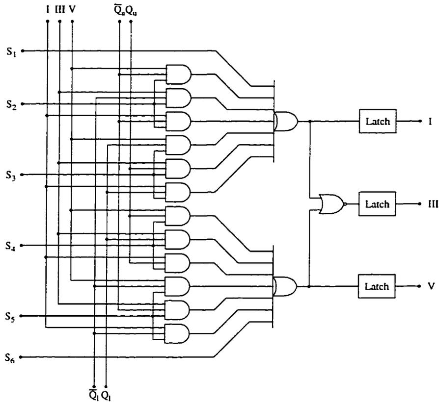
Figure 6.13: A typical circuit for generating new estimates of the combined states.
