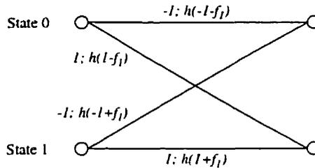
Figure 3.2: Trellis diagram of the system characterized by (3.5). Each branch is labeled with its corresponding pair of *uncoded: encoded* signals.
