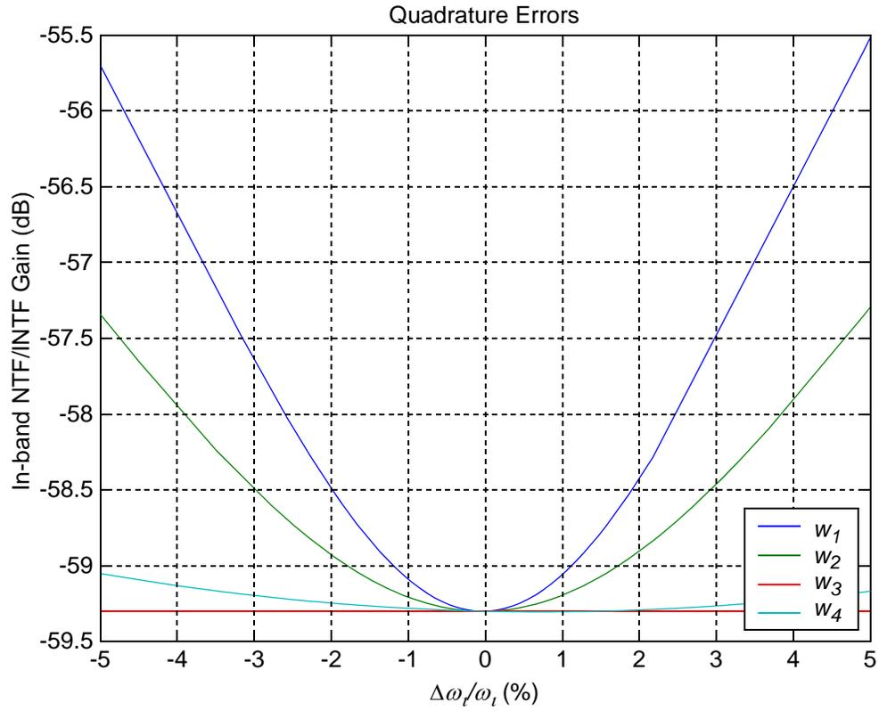
Fig. C.6 Variation of in-band NTF gain due to asymmetrical shifts in NTF zeros.
