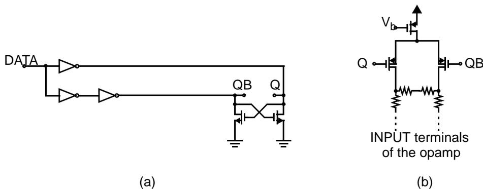
**Fig. 5.7** (a) Switch driver for DAC2. (b) Single current cell of DAC2.
