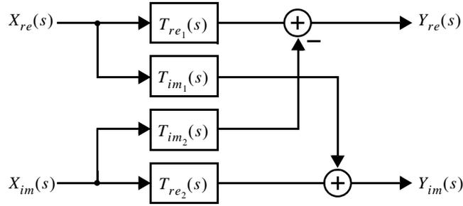
**Fig. 2.5** Block diagram of a generalized complex filter.
