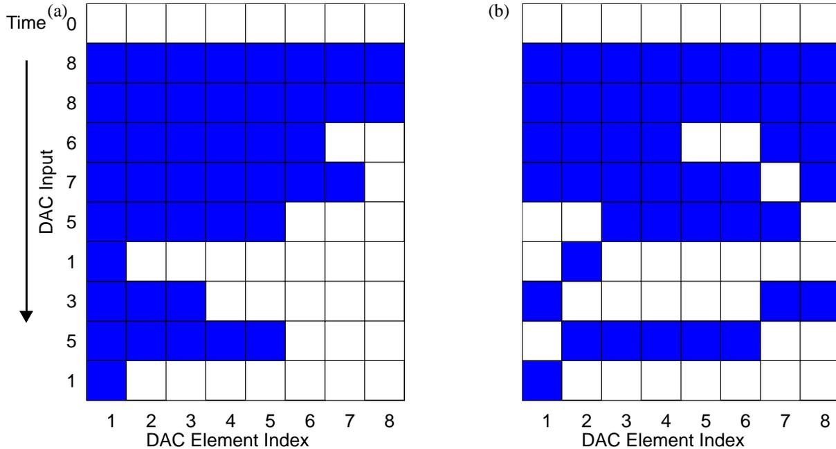
**Fig. 2.3** (a) Example of a DAC usage pattern with no mismatch shaping. (b) Example of a DAC usage pattern with a DWA algorithm. Note: each filled box represents a unit element of a thermometer coded DAC that is to be turned on. The output is the sum of all the elements turned on.
