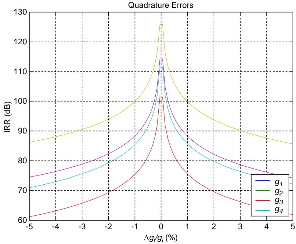
Fig. C.8 Variation of IRR due to change in feedforward gain coefficients.
