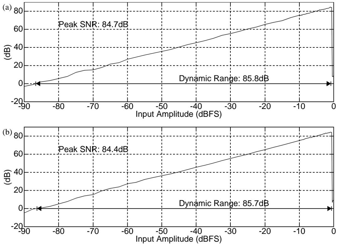
Fig. 3.6 In-band SNR vs. input level for (a) feedback structure (b) feedforward structure.
