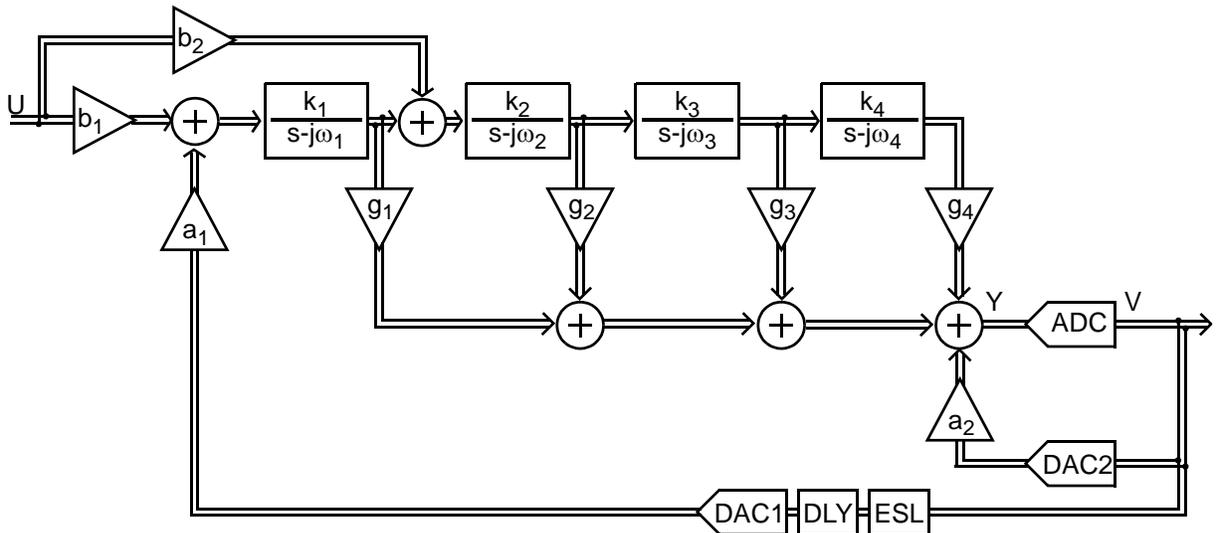
Fig. 3.5 General feedforward structure for implementing any arbitrary 4<sup>th</sup> order modulator.
