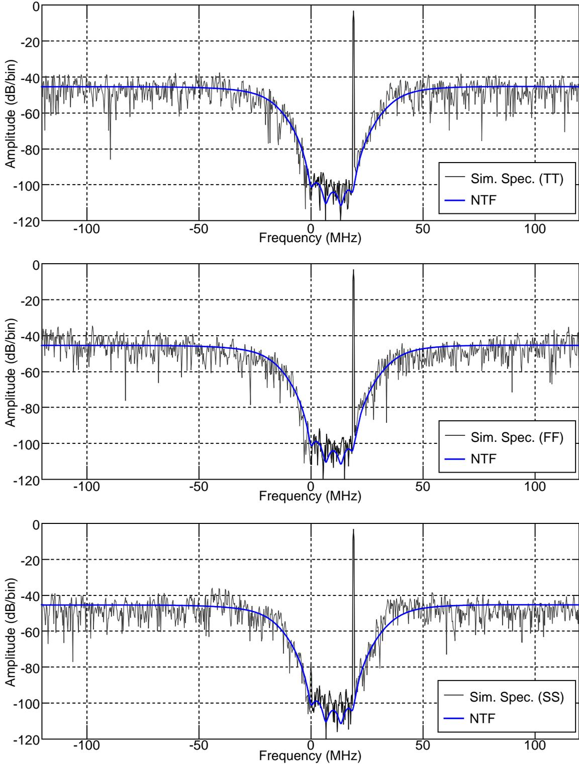
**Fig. 5.13** Simulated spectrum of the ADC with the new coefficients. (a) Spice simulation results using the typical library, 60C and typical absolute resistor and capacitor values. (b) Spice simulation results using the fast-fast library, 0C and -20% resistors and capacitor values. (c) Spice simulation results using the slow-slow library, 80C and +20% resistors and capacitor values.  $N_{FFT}=960$
