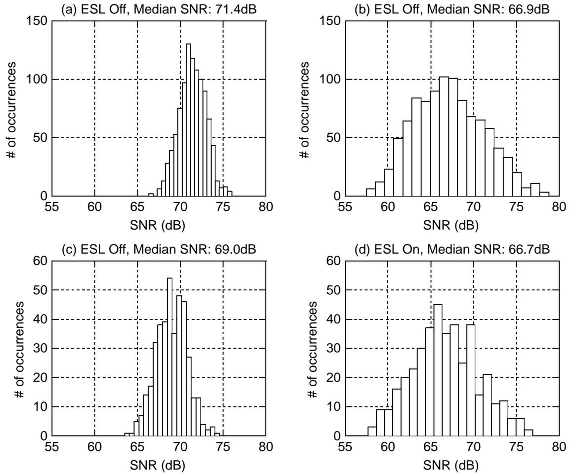
**Fig. 6.10** Matlab Monte-Carlo simulations of the modulator with 15ps of random DAC rise/fall time mismatch with (a) Dynamic mismatch only and DWA turned off, (b) Dynamic mismatch only and DWA turned on, (c) Dynamic and static DAC mismatch, coefficient mismatch, 3ps of clock jitter with the DWA turned off, (d) Dynamic and static DAC mismatch, coefficient mismatch, 3ps of clock jitter with the DWA turned on
