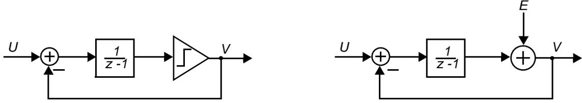
**Fig. 2.2** (a) MOD1: A first order  $\Delta\Sigma$  ADC (b) linearized MOD1.
