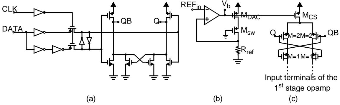
**Fig. 5.6** (a) Switch driver for DAC1 (b) Biasing circuit for DAC1. (c) Single current cell of DAC1.
