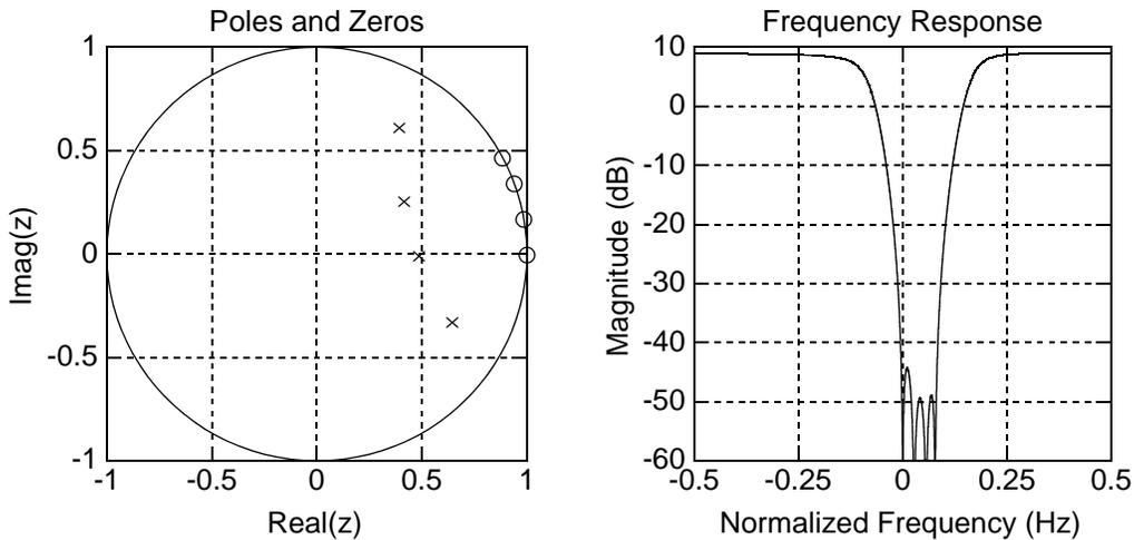
Fig. 3.2 Pole-zero and frequency response plot of the desired NTF.
