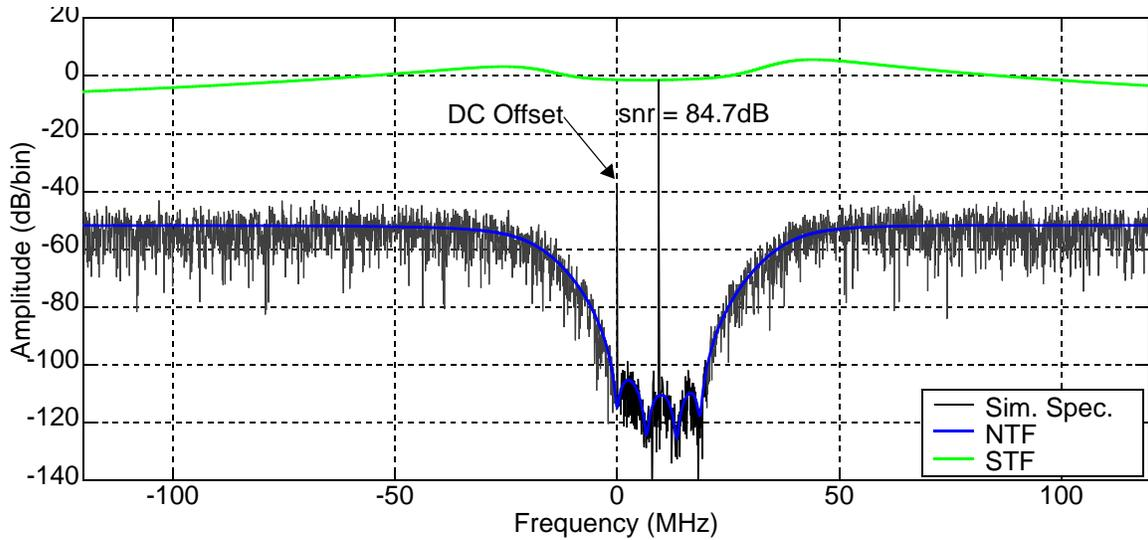
**Fig. 4.8** Spectrum of the modulator with  $10^{-2}$  integrator offset and an input level of -6.0dBFS ( $N_{\text{FFT}} = 4096$ ).
