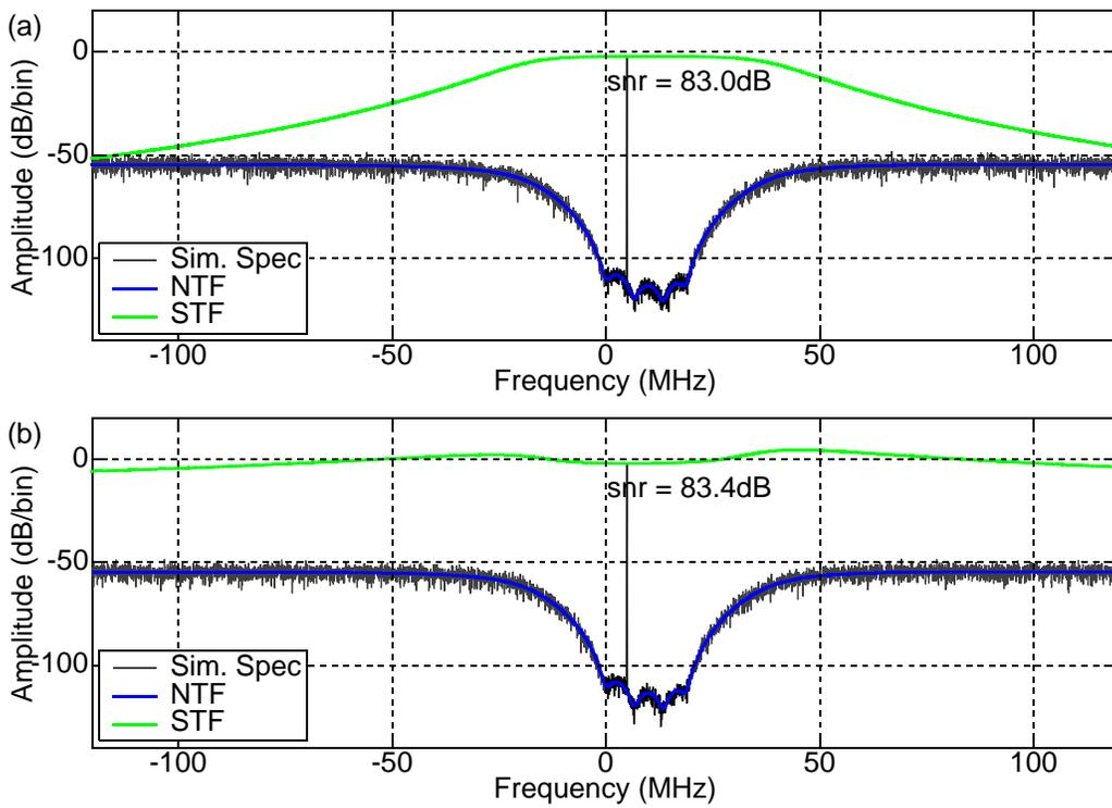
Fig. 3.7 4 Averaged output Spectra,  $N_{FFT} = 8192$  (a) feedback structure (b) feedforward structure.
