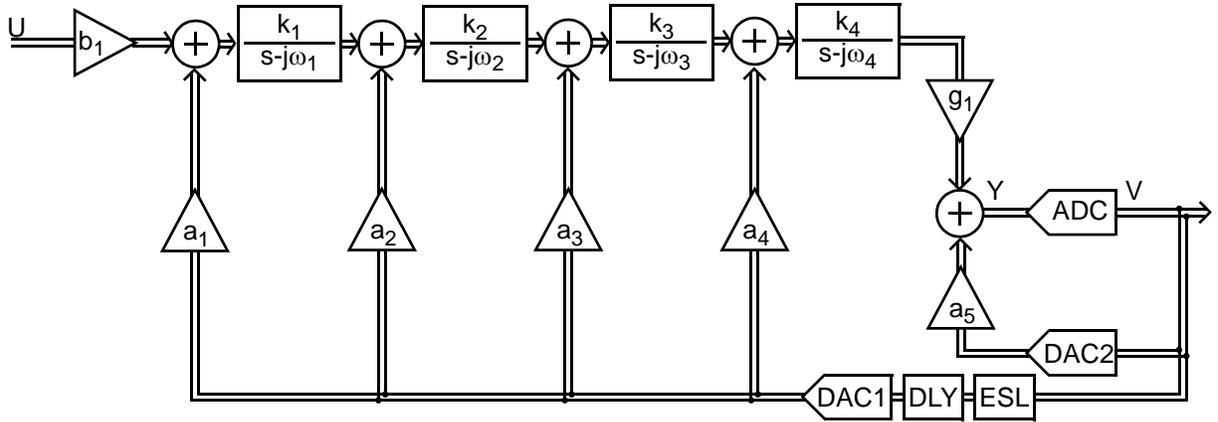
Fig. 3.4 General feedback structure for implementing any arbitrary 4<sup>th</sup> order modulator.
