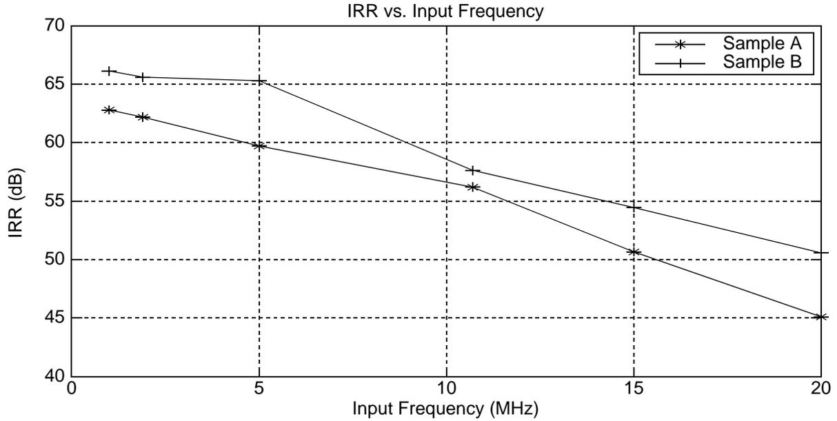
Fig. 6.11 Measured image rejection vs. input frequency at  $f_s=250\text{MHz}$  for two different samples.
