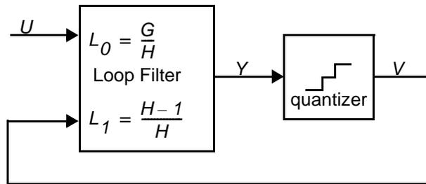
Fig. 2.1 A general block diagram of a  $\Delta\Sigma$  modulator.
