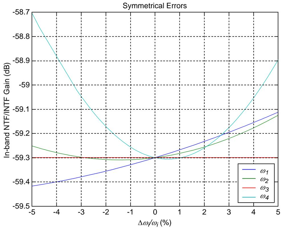
Fig. C.3 Variation of in-band NTF gain due to symmetrical shifts in NTF zeros.
