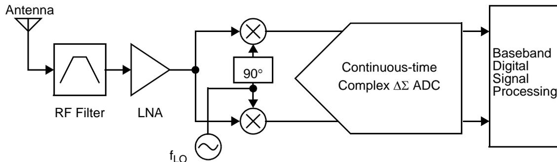
**Fig. 3.1** Block diagram of a low-IF architecture.
