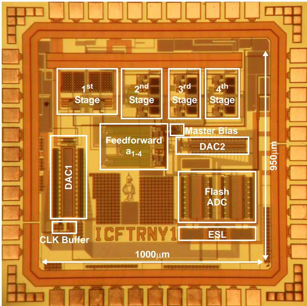
**Fig. 6.1** Micrograph of the IC
