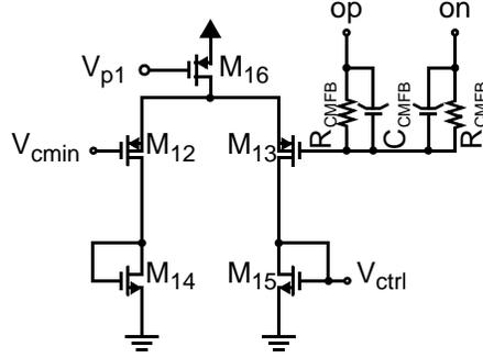
**Fig. 5.5** CMFB circuit used in opamp shown in Fig. 5.4.
