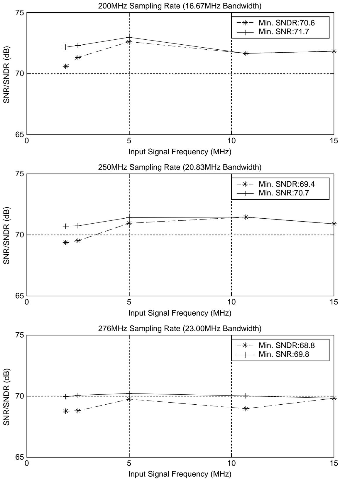
**Fig. 6.7** Measured SNR/SNDR vs. input signal frequency at different clock frequency (DWA turned off).
