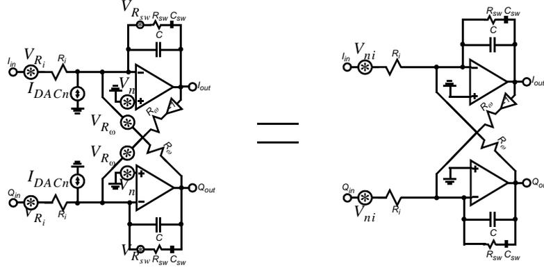
**Fig. 5.2** Equivalent noise model of the complex resonator and with all noise sources referred to the input.
