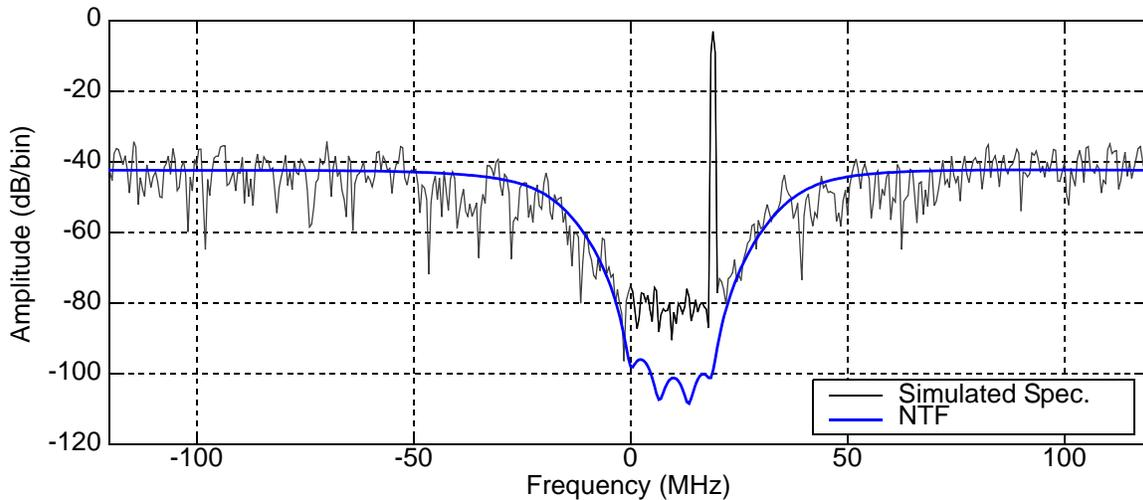
**Fig. 5.16** Simulated spectrum of the extracted using the typical library, 60C and typical absolute resistor and capacitor values.  $N_{\text{FFT}}=480$ .
