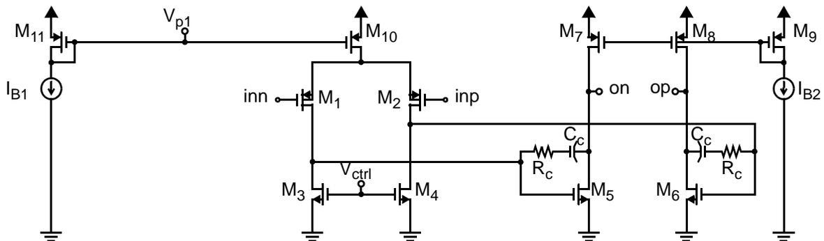
Fig. 5.4 A simple two stage Miller compensated opamp.
