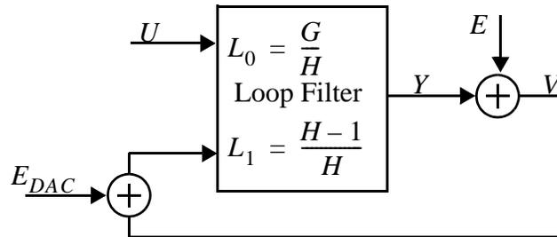
**Fig. 4.6** A general block diagram of a  $\Delta\Sigma$  modulator with DAC.
