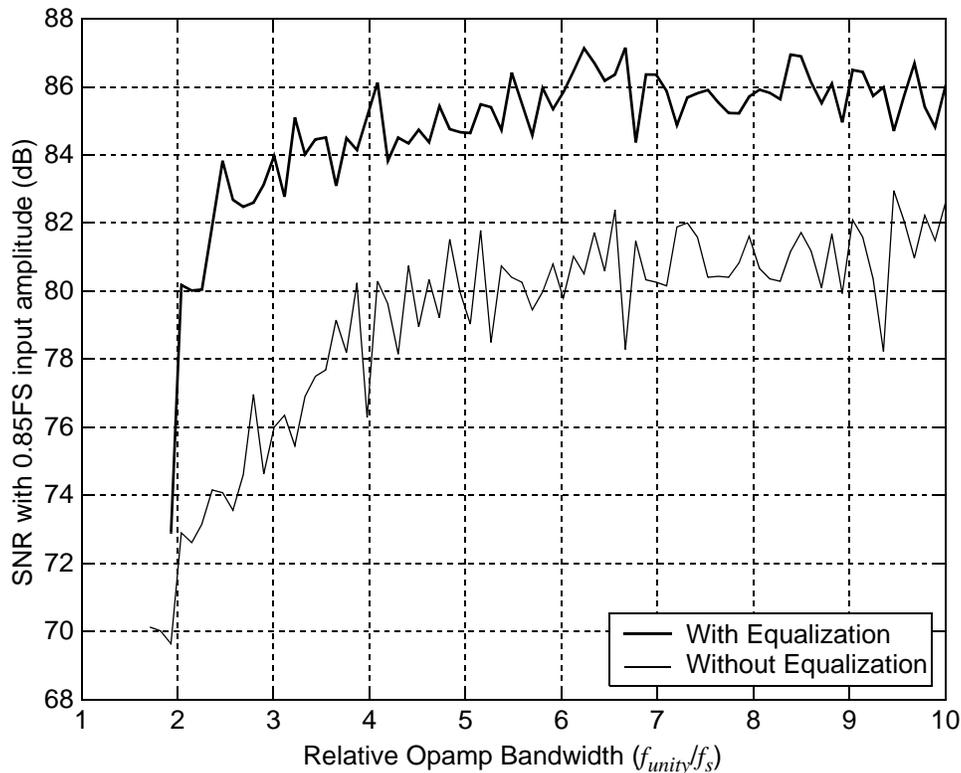
**Fig. 4.2** SNR vs. Opamp bandwidth with/without impulse matching.
