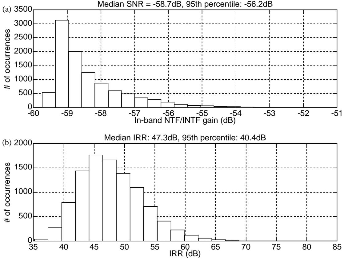
**Fig. 4.4** (a) In-band NTF/INTF gain and (b) IRR histogram of 10000 perturbed modulators shown in Fig. 4.6. Assuming the error introduced by element mismatches in the feedback DAC can be modeled as additive white noise, the linear model of a multi-bit  $\Delta\Sigma$  modulator is
