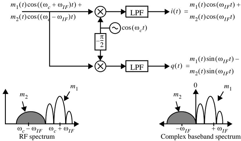
**Fig. 2.4** Low-IF down conversion using an image reject mixer.
