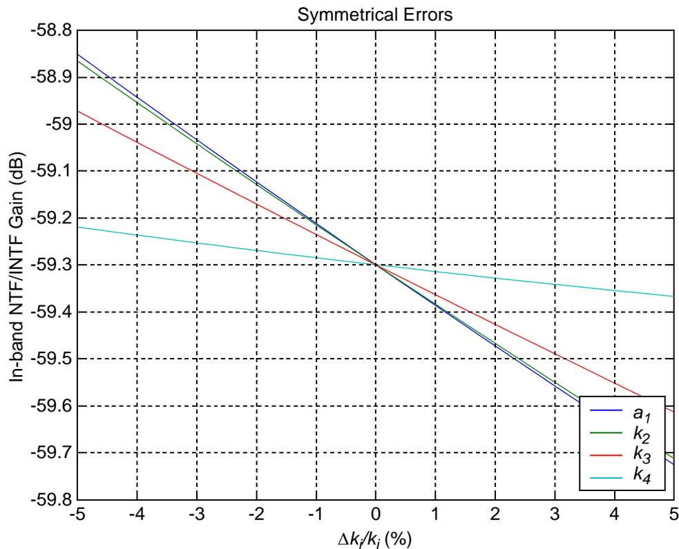
**Fig. C.1** Variation of in-band NTF gain due to symmetrical shifts in inter-stage gain coefficients.
