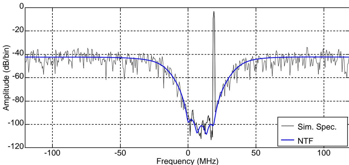
**Fig. 5.12** Simulated spectrum of the ADC with the DAC clock advanced by 700ps.
