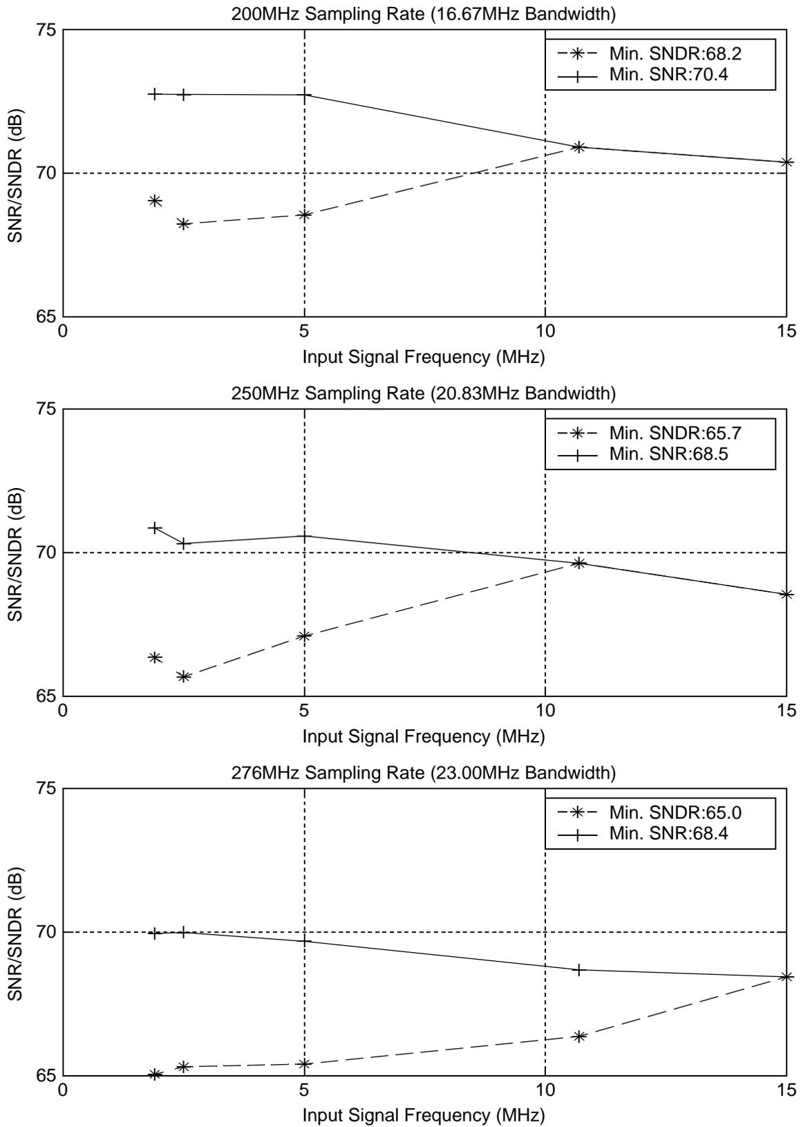
**Fig. 6.6** Measured SNR/SNDR vs. input signal frequency at different clock frequency (DWA turned on).
