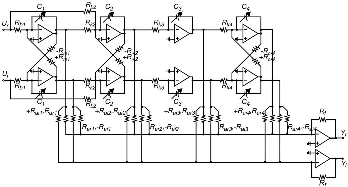
Fig. 5.1 Single-ended representation of the ADC loop filter.
