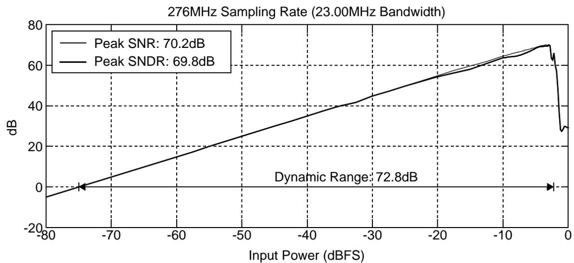
**Fig. 6.5** Measured SNR/SNDR vs. input signal power at different clock frequency with an input signal frequency of 5.0MHz. (DWA turned off).
