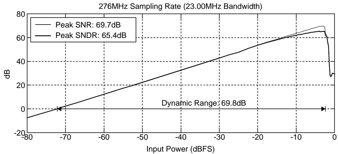
**Fig. 6.4** Measured SNR/SNDR vs. input signal power at different clock frequency with an input signal frequency of 5.0MHz. (DWA turned on).
