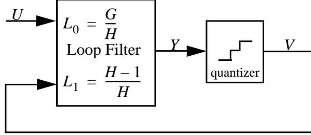
**Fig. A.1** A general block diagram of a  $\Delta\Sigma$  modulator.
