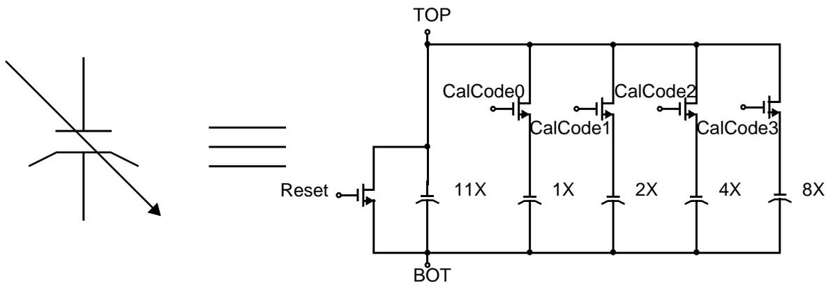
**Fig. 5.3** Circuit used to tune for variations in RC time constant due to process variations.
