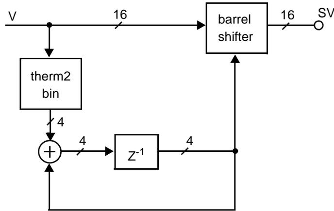
**Fig. 5.10** Block diagram of the DWA circuit.
