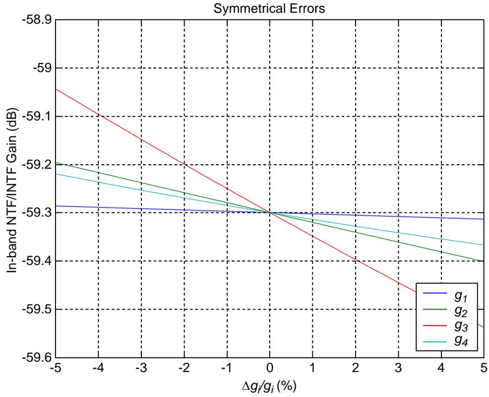
Fig. C.2 Variation of in-band NTF gain due to symmetrical shifts in feedforward gain coefficients.
