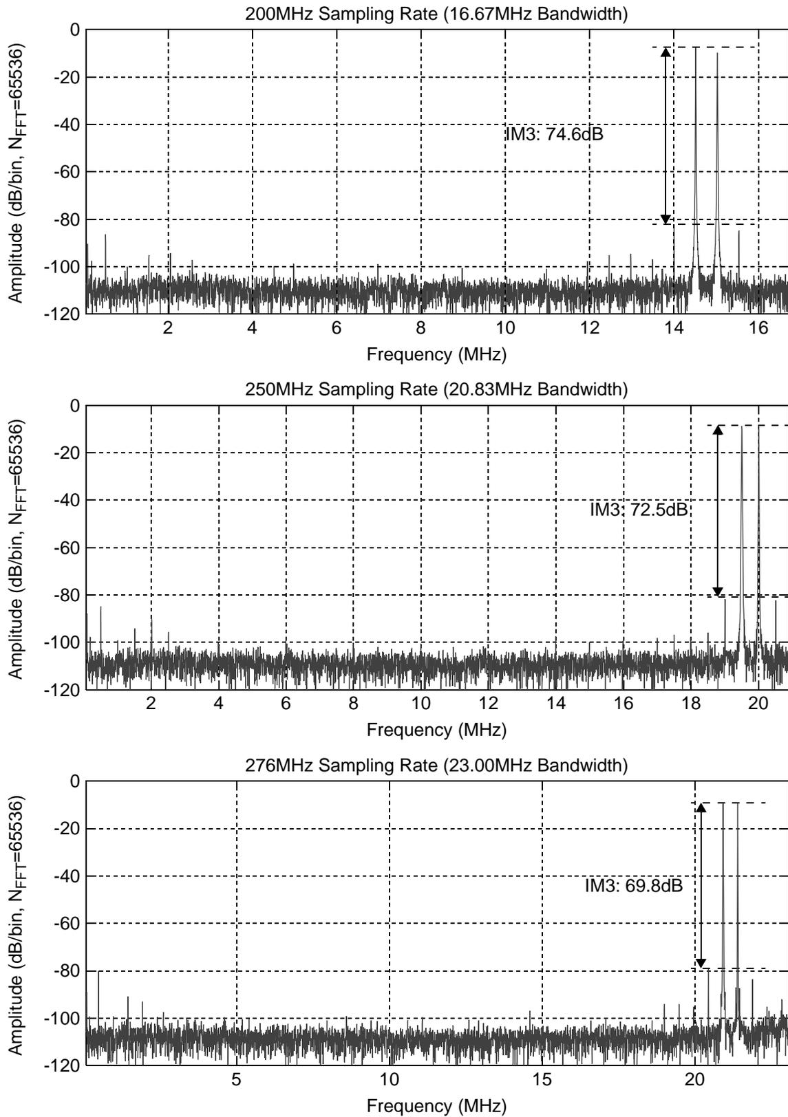
**Fig. 6.8** Output spectra of two-tone intermodulation distortion test. Peak-to-peak signal amplitude is same as the signal amplitude which produces peak SNDR with a single tone at 5.0MHz (DWA turned off).
