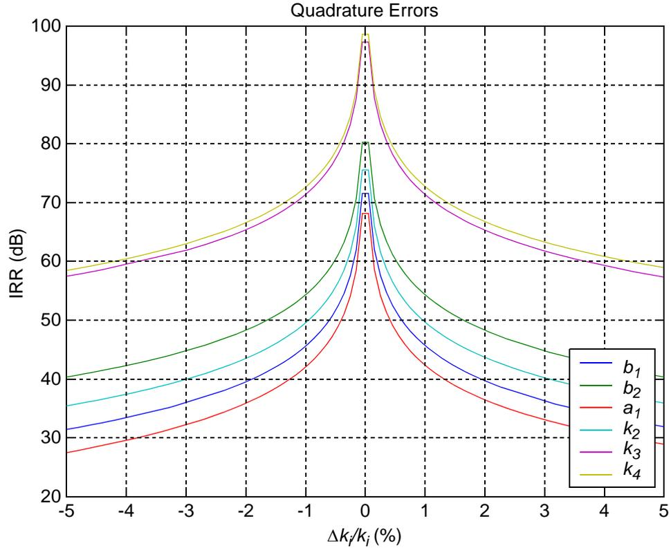
Fig. C.7 Variation of IRR due to changes in inter-stage gain and input coefficients.
