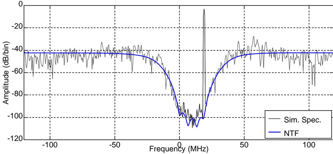
**Fig. 5.11** Simulated spectrum of the ADC using initial values of  $g_i$ .
