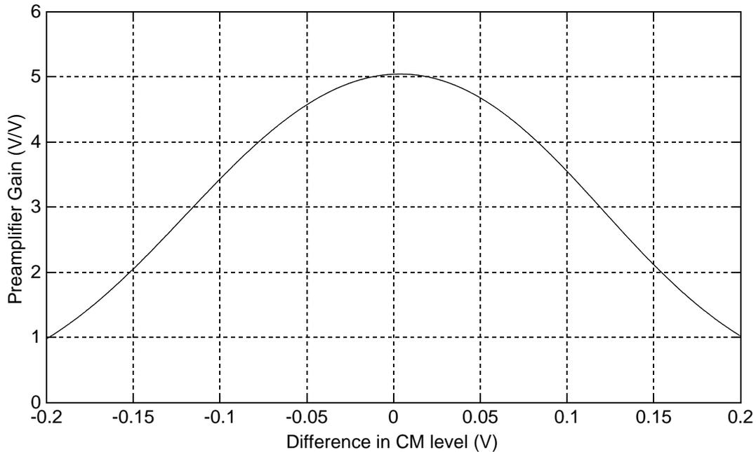
Fig. 5.8 Preamp gain vs. difference in CM level.
