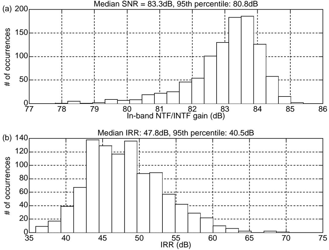
**Fig. 4.5** (a) In-band SNR and (b) IRR histogram of 1000 perturbed modulators.
