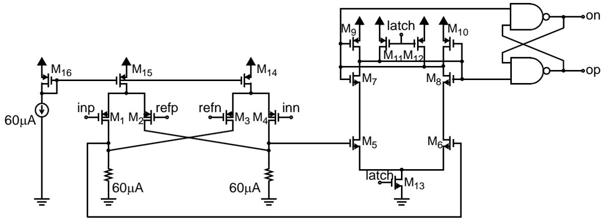
Fig. 5.9 CMOS comparator.
