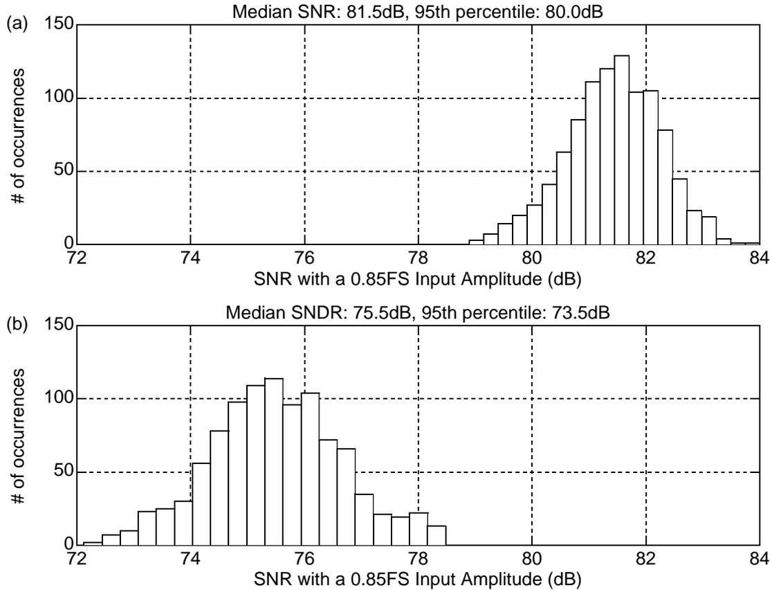
**Fig. 4.7** Histogram of 1000 modulators with 0.5% mismatch in DAC1 and 1% mismatch in DAC2 with (a) DWA turned on and (b) DWA turned off.
