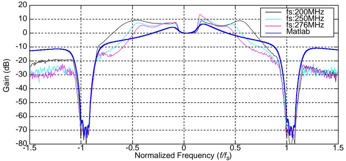
**Fig. 6.9** Measured signal transfer function at various clock frequencies. DWA turned off.
