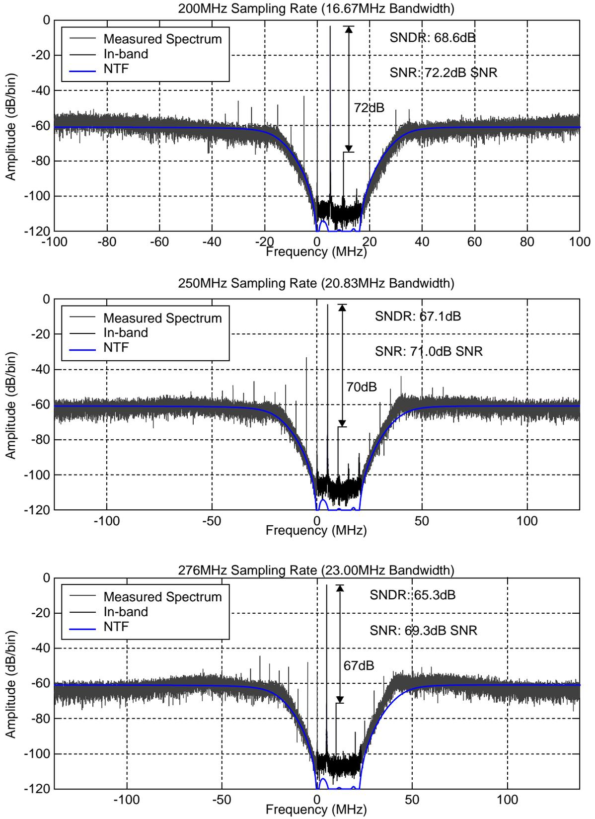
**Fig. 6.2** Measured spectra at different clock frequency with an input signal frequency of 5.0MHz (DWA turned on,  $N_{FFT}=32768$ ).
