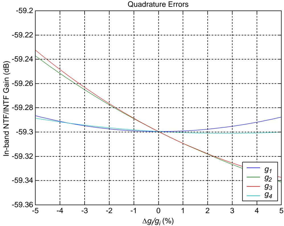
**Fig. C.5** Variation of in-band NTF gain due to asymmetrical shifts in feedforward gain coefficients.
