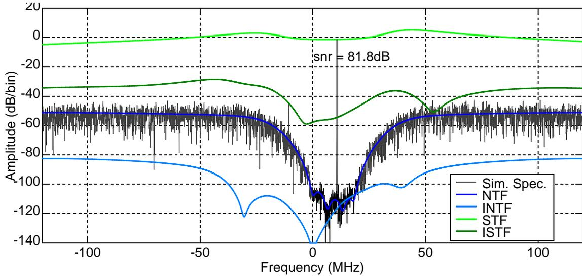
**Fig. 4.3** Output spectrum of the modulator with 1.0% quadrature mismatch in coefficient values.
