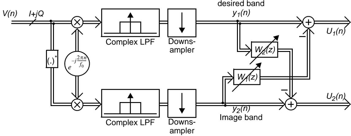
**Fig. 2.6** Block diagram of the mismatch cancellation system.
