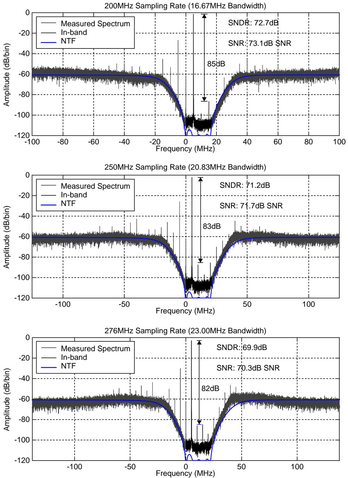
**Fig. 6.3** Measured spectra at different clock frequency with an input signal frequency of 5.0MHz (DWA turned off,  $N_{FFT}=32768$ ).
