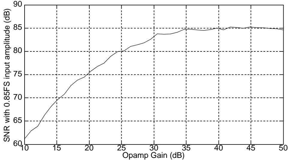
**Fig. 4.1** SNR vs. finite opamp gain.
