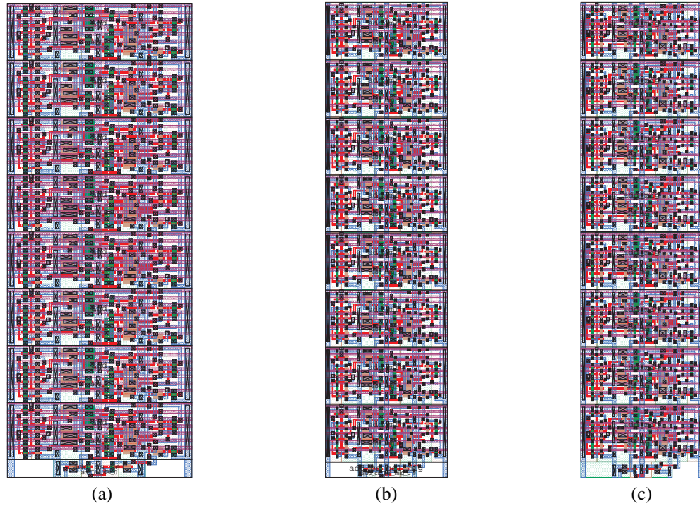
Figure 7: Migration of 8-bit adder (a)Original layout; (b) Migrated layout in TSMC 0.25 \mu\text{m} ; (c) Migrated layout in TSMC 0.18 \mu\text{m} .
