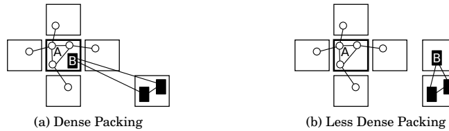
Fig. 3: Packing density and wire length example.
