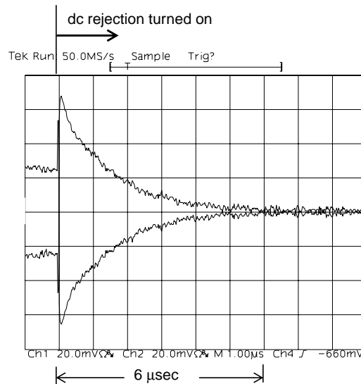
Figure 6.25 Measured step response of dc photocurrent rejection circuit to 10\text{ }\mu\text{A} dc input.
