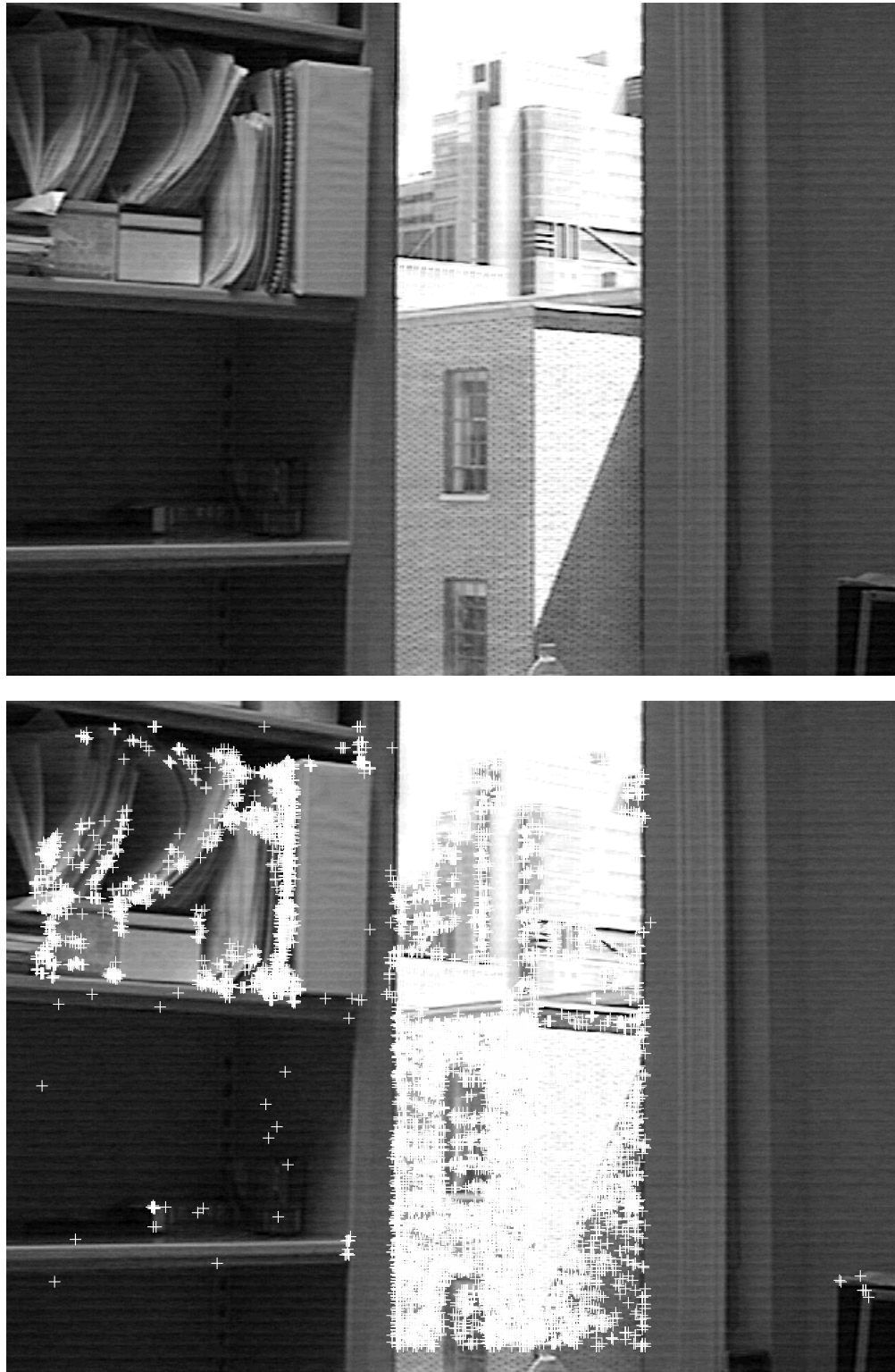
Figure 4.11: Sample output of the feature detector running on the Transmogriker-4. The original image is shown at the top. The location of the features obtained from the circuit have been superimposed on the original image and marked with white '+' signs
