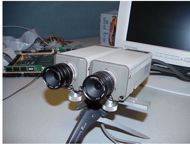
Figure 3.2: The camera head with two 1/2" CCD cameras. The focal length of the camera lenses is 12mm and the separation between the optic centers of the cameras is 70mm.
