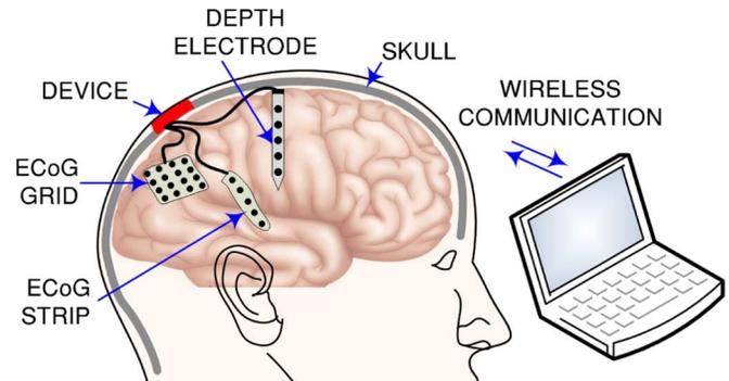
Fig. 1. Envisioned implant configuration of the proposed therapeutic neurostimulation device: neurostimulator interfaces with the ECoG grid/strip and/or the depth electrodes depending on the location of the epileptogenic zone.
