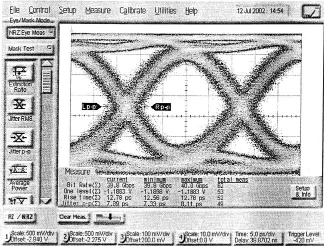
Fig. 24. Measured 40-Gb/s eye diagram with a  $2^{31}-1$  pattern showing the maximum output dc offset level of  $-1.1$  V.
