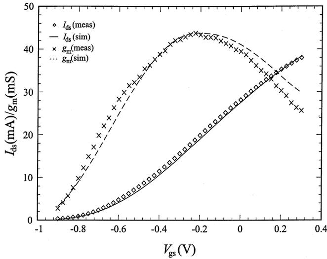
Fig. 1. Measured versus simulated drain current and transconductance for a  $2 \times 40 \mu\text{m}$  GaAs pHEMT biased at  $V_{ds} = 2.5 \text{ V}$ .
