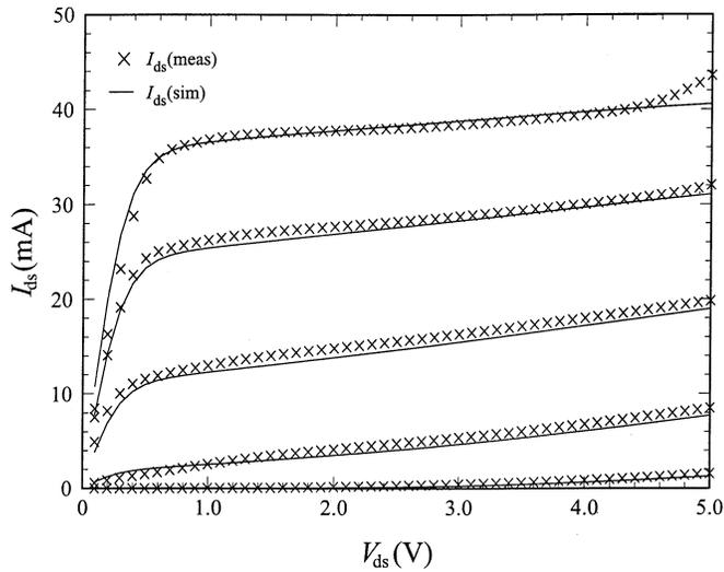
Fig. 2. Measured versus simulated dc output characteristics for a  $2 \times 40 \mu\text{m}$  GaAs pHEMT.
