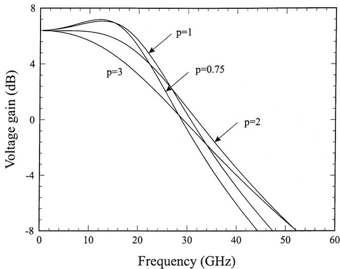
Fig. 12. Voltage gain of the SSF-INV stage as a function of frequency and of the scaling ratio  $p$  between the size of the transistors in the inverter and the source follower.
