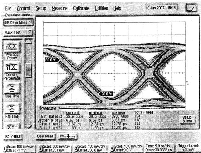
Fig. 18. Measured 40-Gb/s eye diagram with a  $2^{31} - 1$  pattern for the test setup without DUT.
