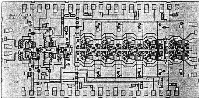
Fig. 17. Microphotograph of the EA modulator driver IC.
