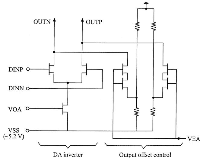
Fig. 9. Distributed amplifier inverting stage showing the output offset and amplitude control function implementations.
