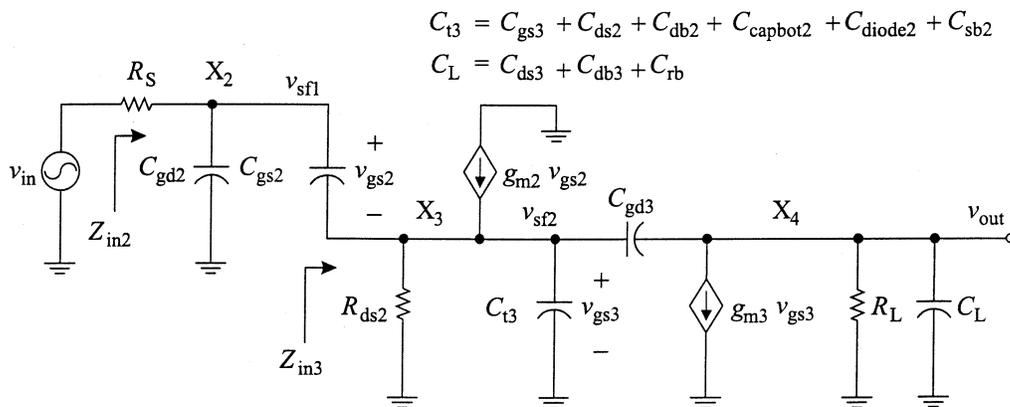
Fig. 11. Small-signal equivalent circuit used in the analytical derivation of the frequency response of a SSF-INV stage.
