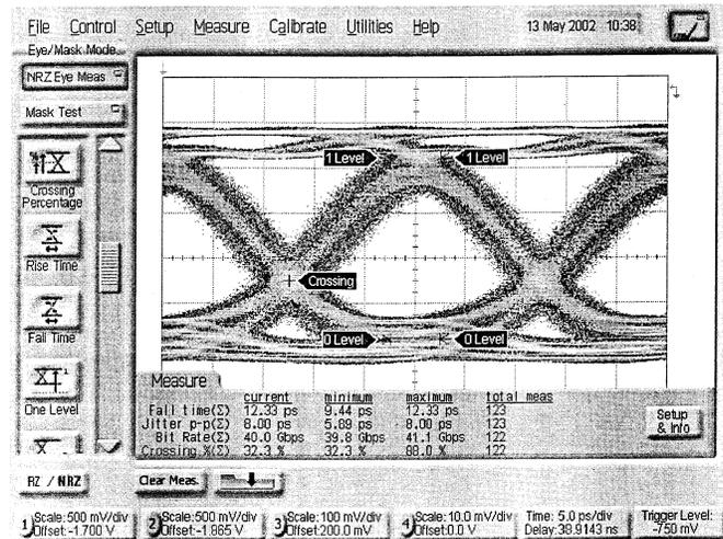
Fig. 22. Measured 40-Gb/s eye diagram with a  $2^{31} - 1$  pattern showing the eye crossing at 30% (pulsewidth control).
