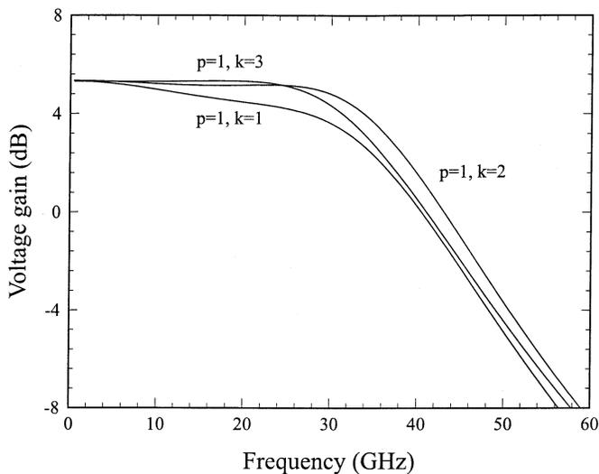
Fig. 15. Voltage gain of the DSF-INV stage as a function of frequency and of the scaling ratio  $k$  between the size of the transistors in the second and first source-follower stages. The scaling ratio  $p$  between the size of the transistors in the inverter and in the second source follower remains constant.
