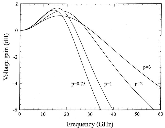
Fig. 13. Transfer function of the input voltage divider formed by the signal source impedance and the input impedance of the SSF-INV stage as a function of the scaling ratio  $p$  between the size of the transistors in the inverter and the source follower.
