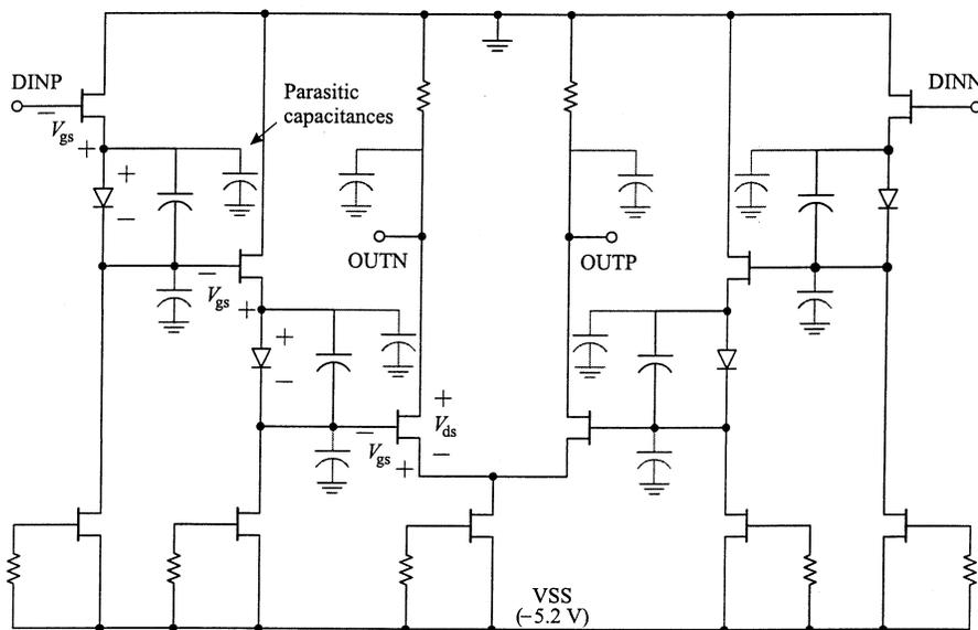
Fig. 10. Basic DSF-INV gain block with ac-bypassed level-shifting diodes. The parasitic capacitances to ground arising from the transistor terminals, level-shifting diodes, and bypass capacitors are illustrated.
