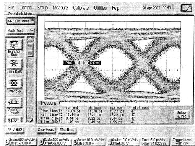
Fig. 21. Measured 44-Gb/s eye diagram with a  $2^{31} - 1$  pattern showing 3 V<sub>pp</sub> output swing per side.
