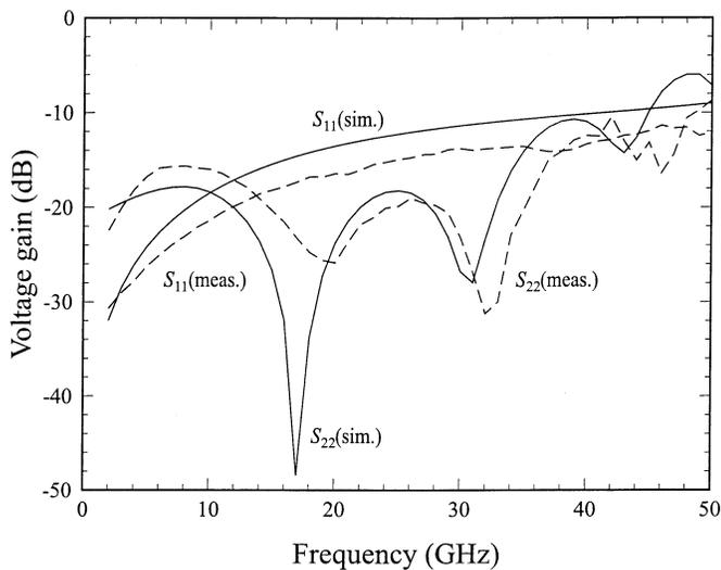
Fig. 19. Measured versus simulated input and output return loss at 18 °C.
