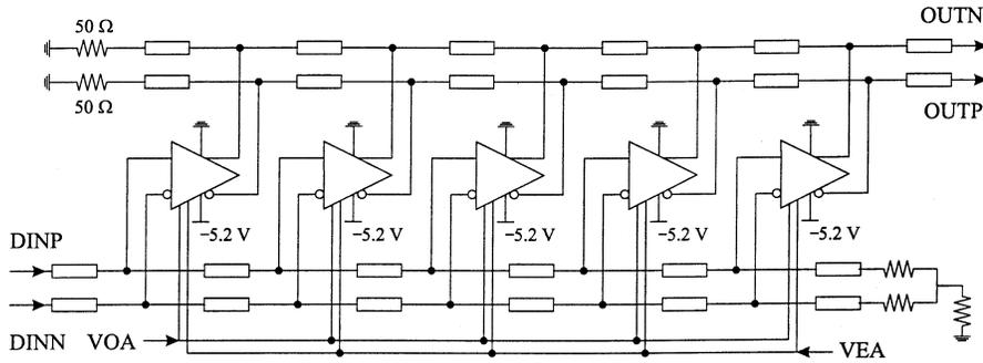
Fig. 8. Block diagram of the distributed amplifier section.
