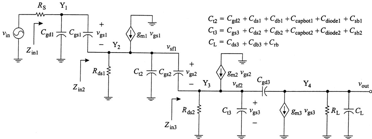
Fig. 14. Small-signal equivalent circuit used in the analytical derivation of the frequency response of a DSF-INV stage.
