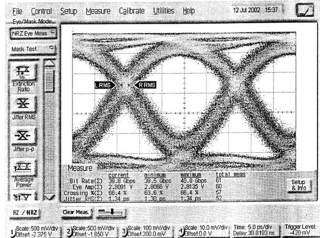
Fig. 23. Measured 40-Gb/s eye diagram with a  $2^{31} - 1$  pattern showing the eye crossing at 66% (pulsewidth control).
