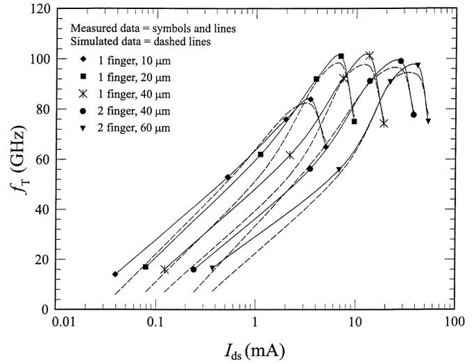
Fig. 3. Measured versus simulated  $f_T$ - $I_{ds}$  characteristics of  $1 \times 10 \mu\text{m}$ ,  $1 \times 20 \mu\text{m}$ ,  $1 \times 40 \mu\text{m}$ ,  $2 \times 40 \mu\text{m}$ , and  $2 \times 60 \mu\text{m}$  GaAs pHEMTs at  $18^\circ\text{C}$  and  $V_{ds} = 2.5 \text{ V}$ .
