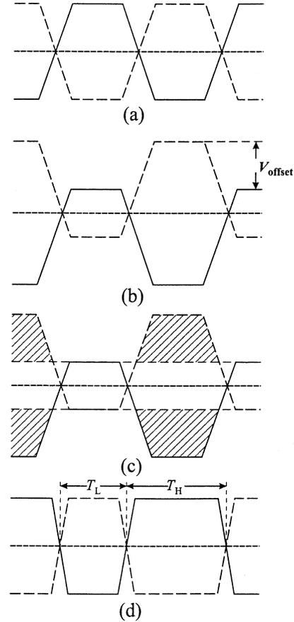
Fig. 7. Pulsewidth control function signal flow. (a) Signal at the input of the middle limiter inverter. (b) Signal at the output of the middle limiter inverter after applying a dc offset through the DCAP and DCAN control inputs. (c) Illustration of the amplitude limiting function of the next stage. (d) Resulting signal with modified pulsewidth at the output of the next limiting stage.
