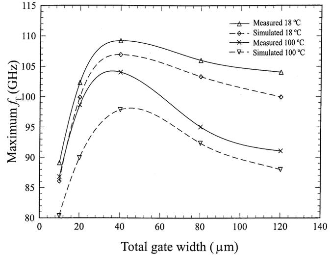
Fig. 4. Measured and simulated maximum  $f_T$  values versus total gate width and temperature for  $V_{ds} = 1.5 \text{ V}$  and  $V_{gs} = -0.1 \text{ V}$ .
