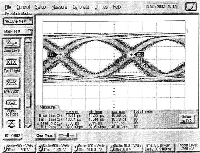
Fig. 25. Measured 40-Gb/s eye diagram with a  $2^{31}-1$  pattern showing the minimum  $1.7$  V<sub>pp</sub> output swing per side.
