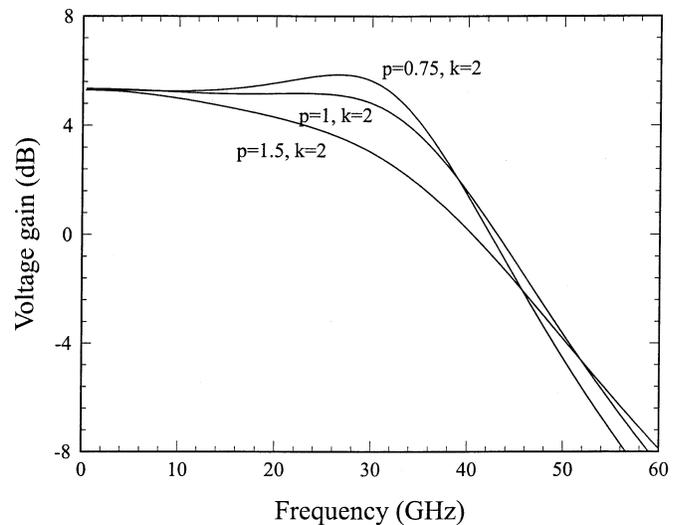
Fig. 16. Voltage gain of the DSF-INV stage as a function of frequency and of the scaling ratio  $p$  between the size of the transistors in the inverter and in the second source follower. The scaling ratio  $k$  between the size of the transistors in the second and first source follower stages remains constant.
