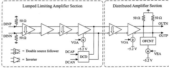
Fig. 5. Block diagram of the 40-Gb/s EA modulator driver illustrating the lumped and distributed sections.
