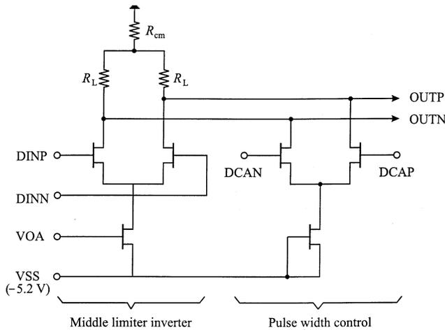
Fig. 6. Middle-stage inverter showing pulsewidth and output amplitude control function implementation.
