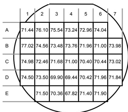
Fig. 12. Wafer map of the self-oscillation frequency (in GHz) for the BipX dividers without EF.
