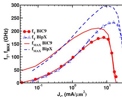
Fig. 5. Measured  $f_T$  and  $f_{MAX}$  at  $V_{CE}=1\text{V}$  on transistors with 3 emitter stripes, 6 base, and 4 collector contacts in the two technologies (BiCMOS9 and BipX).
