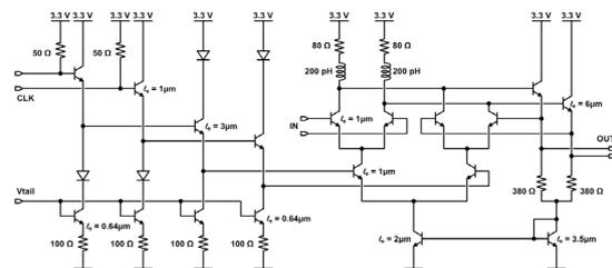
Fig. 3a. Schematic of the latch with emitter followers.
