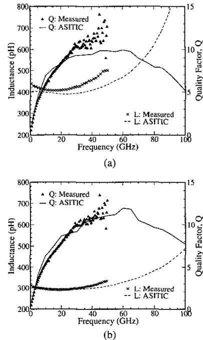
Fig. 6: Measured and modeled  $L_{EFF}$  and Q for (a) 440-pH and (b) for 330-pH inductors.
