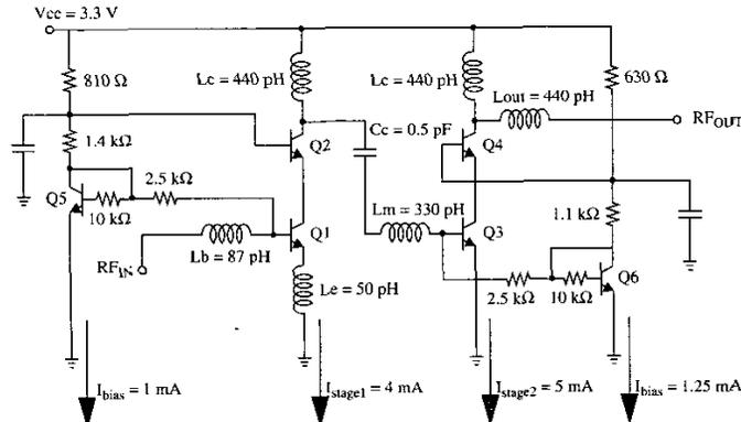
Fig. 2: LNA circuit schematic including the on-chip biasing network.
