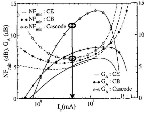
Fig. 1: Simulated  $NF_{\min}$  and  $G_A$  at 52 GHz for common-emitter, common-base, and cascode configuration versus the bias current ( $V_{CC}$  is 1.5 V for CE, CB and 2.5 V for cascode).
