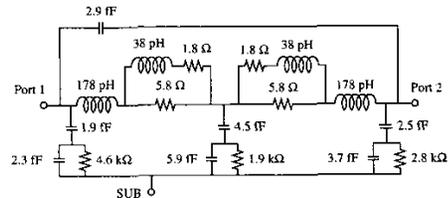
Fig. 3: 440-pH inductor 2- $\pi$  model.
