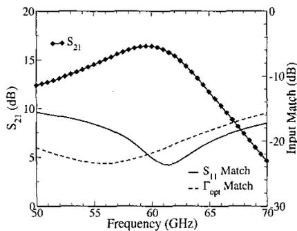
Fig. 4: Simulated gain, input return loss, and optimum noise reflection coefficient  $\Gamma_{\text{opt}}$ .
