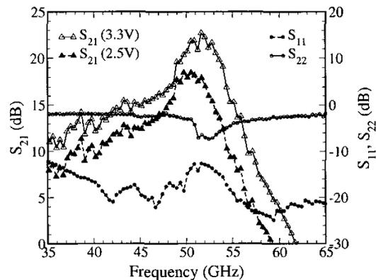
Fig. 7: LNA S-parameter measurements to 65 GHz.
