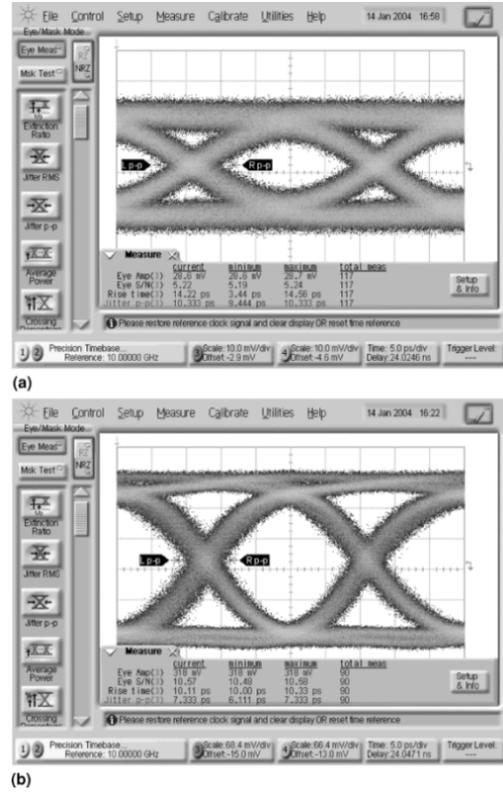
Fig. 19. On-wafer measured 43 Gb/s, single-ended input (a) and output (b) eye diagram corresponding to a 420  $\mu\text{A}_{\text{PP}}$  input with  $2^{31} - 1$  PRBS.
