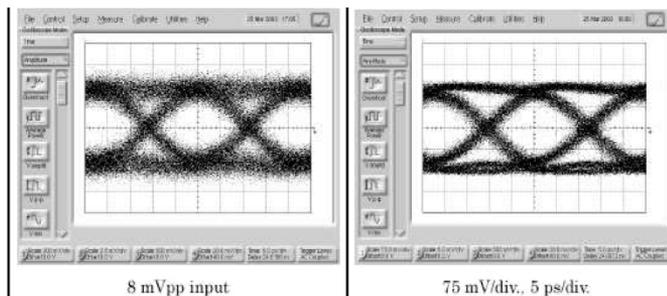
Fig. 21. Measured 43 Gb/s,  $2^{23} - 1$  input ( $8 \text{ mV}_{\text{pp}}$ ) and output ( $320 \text{ mV}_{\text{pp}}$ ) single-ended eye diagram of the TIALA mounted in a customer module as a limiting amplifier.
