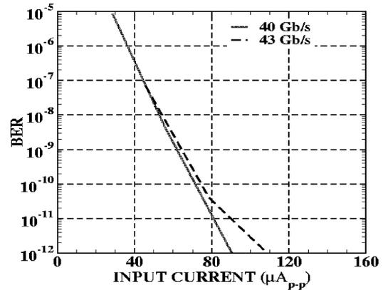
Fig. 15. Measured sensitivity with a  $2^{31} - 1$  PRBS.
