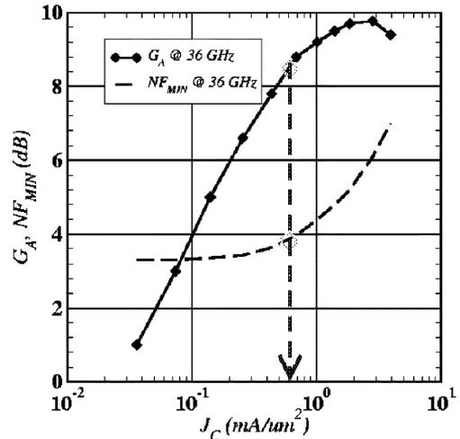
Fig. 3. Simulated  $NF_{MIN}$  and  $G_a$  versus  $I_c$  characteristics of a  $1 \times 5 \mu\text{m}^2$  InP HBT biased at  $V_{CE} = 1 \text{ V}$ .
