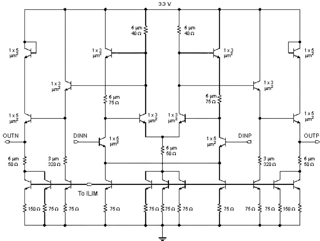
Fig. 6. Differential LA stage schematic.
