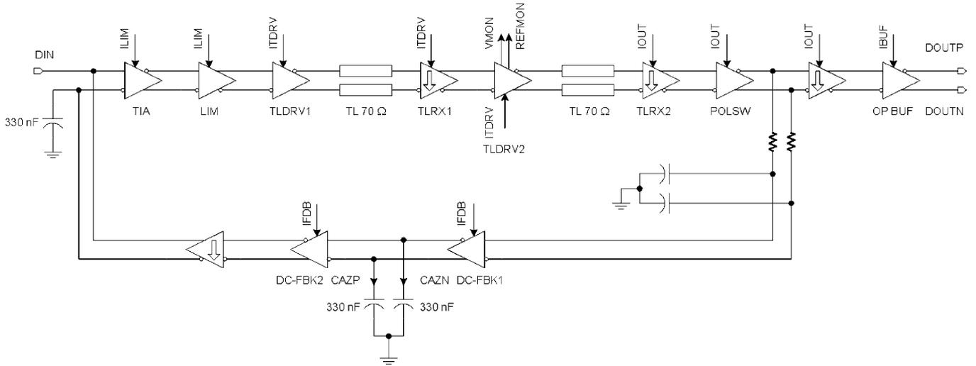
Fig. 1. Block diagram of the TIALA with single photodiode input. The unused TIA input is ac-coupled to ground in order to reduce noise. Emitter-follower stages are identified by a downward pointing arrow.
