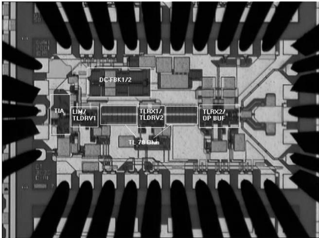
Fig. 10. Microphotograph of the TIALA with HF wafer probes.
