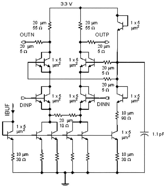
Fig. 8. Differential output stage schematic.
