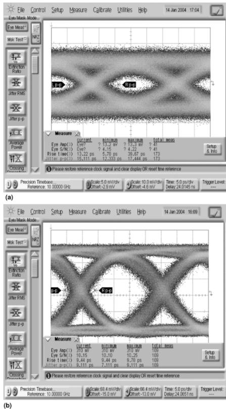
Fig. 20. On-wafer measured 43-Gb/s, single-ended input (a) and output (b) eye diagram corresponding to a  $190 \mu\text{A}_{\text{pp}}$  input with  $2^{31} - 1$  PRBS.
