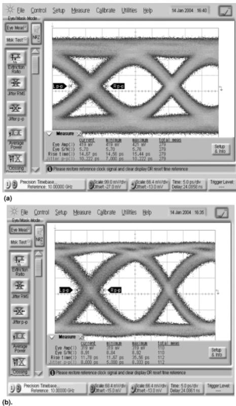
Fig. 18. On-wafer measured 43-Gb/s, single-ended (a) input and (b) output eye diagram corresponding to a 6.2  $\text{mA}_{\text{PP}}$  input with  $2^{31} - 1$  PRBS.
