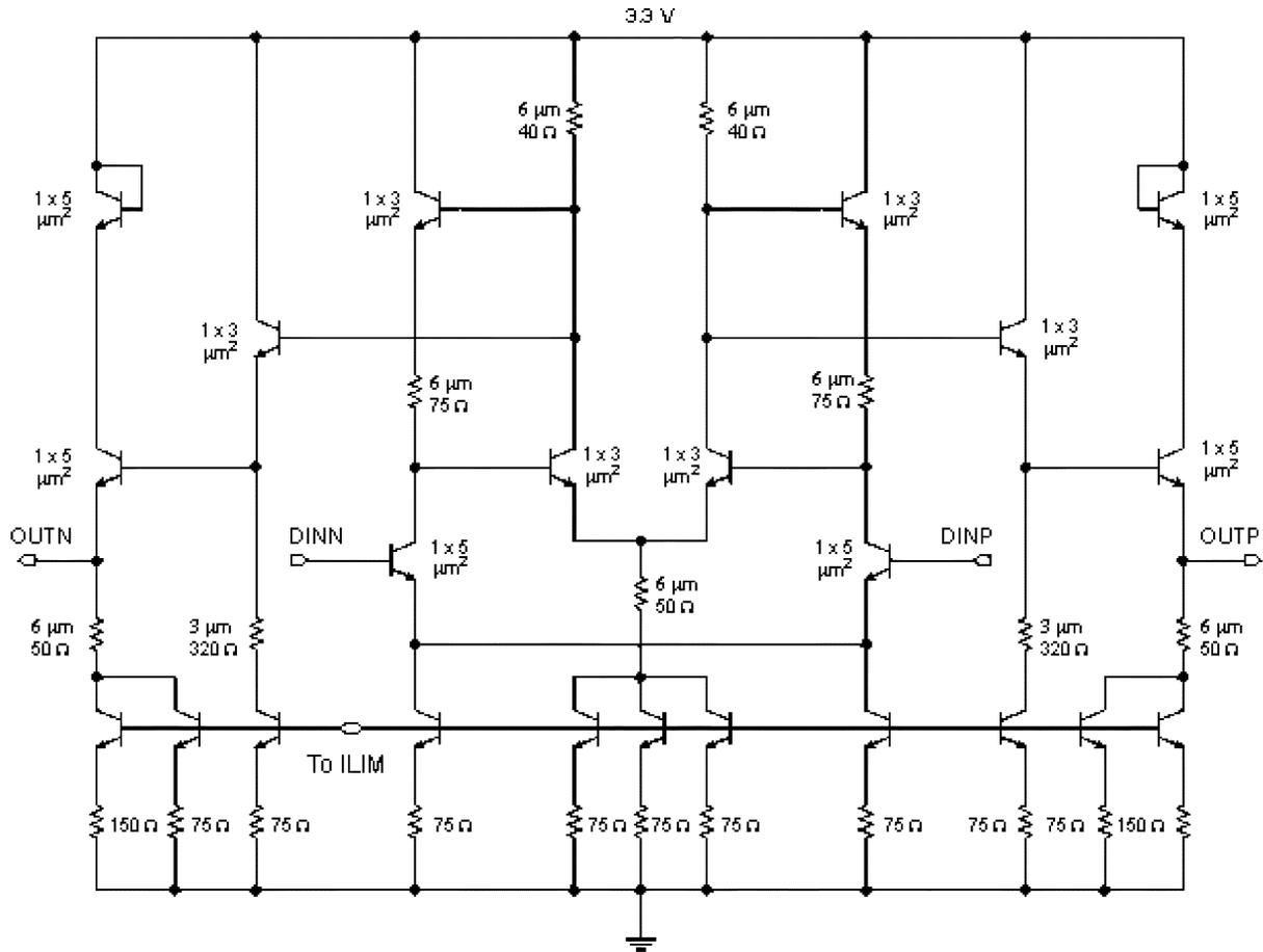
Fig. 6. Differential LA stage schematic.
