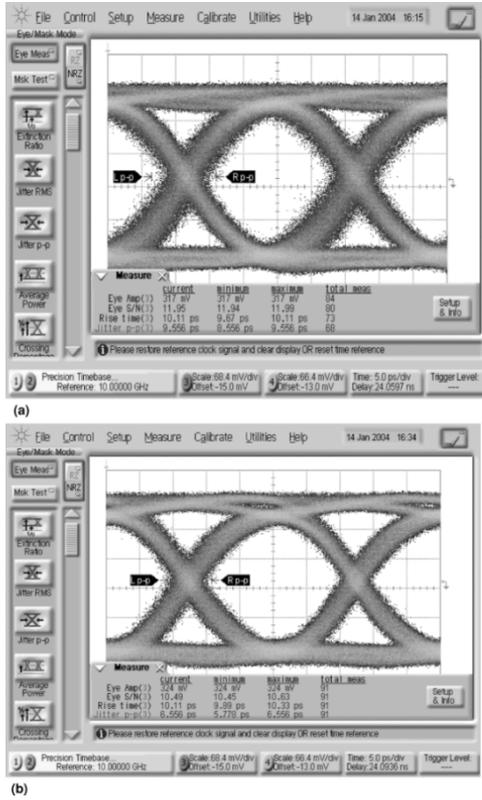
Fig. 17. On-wafer measured 40-Gb/s single-ended output eye diagrams corresponding to (a) 190  $\mu\text{A}_{\text{PP}}$  and (b) 6.2  $\text{mA}_{\text{PP}}$  inputs with  $2^{31} - 1$  PRBS.
