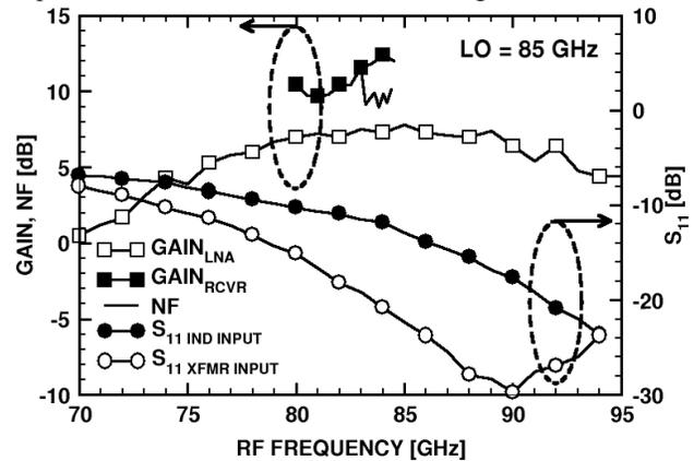
Fig. 6. Measured differential conversion gain, NF and  $S_{11}$  at RF port of the two receivers as functions of the RF frequency when the LO is 85 GHz. The gain of an inductor-feedback LNA breakout is also shown for reference.
