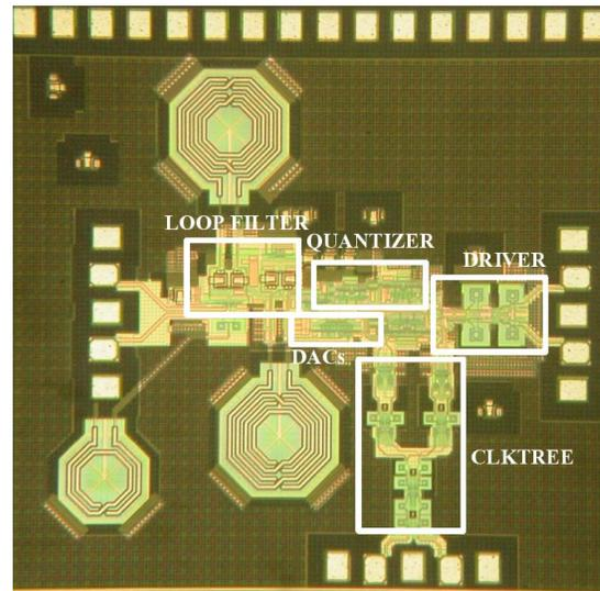
Fig. 12. Chip microphotograph.
