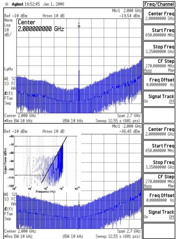
Fig. 8. Measured ADC spectrum for 2-GHz input and no input.
