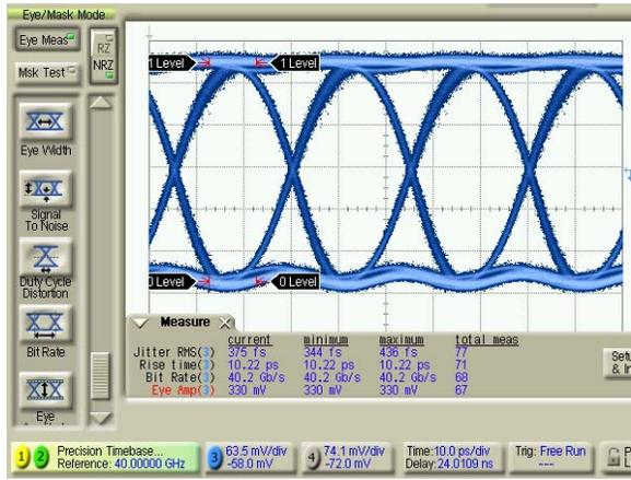
Fig. 6. Output eye diagram at 40Gbps.
