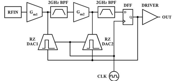
Fig. 1. System level ADC model.
