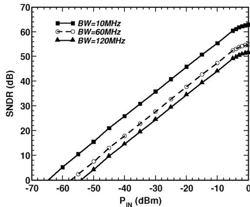
Fig. 10. Dynamic range for a 2-GHz single tone input.
