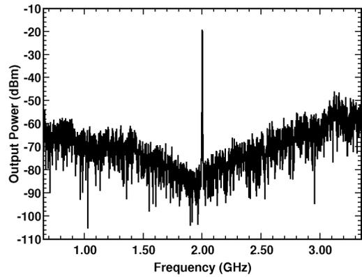
Fig. 7. Simulated ADC spectrum (NFFT=32K).
