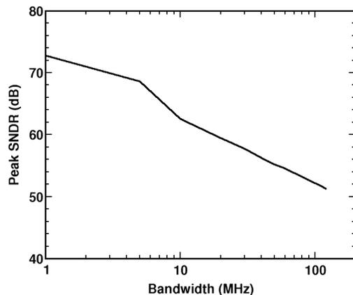
Fig. 11. Peak-SNDR vs bandwidth for a 2-GHz single tone input.
