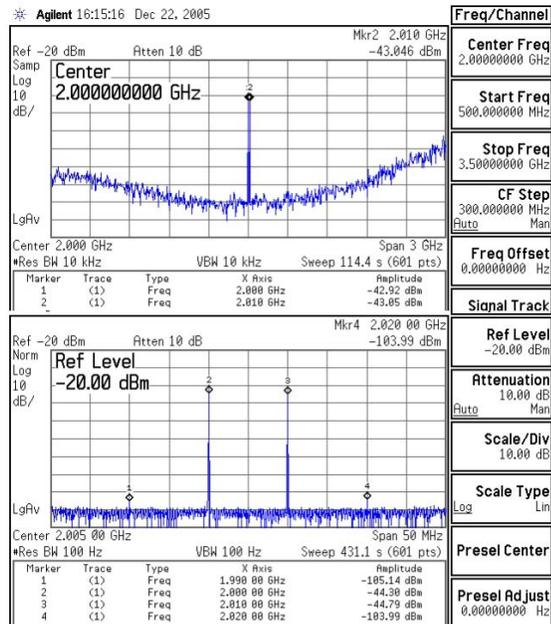
Fig. 9. ADC two-tone spectra at 2 GHz with  $P_{in}=-30$  dBm.
