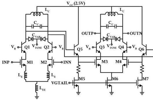
Fig. 2. Circuit schematic of 2-stage loop filter.
