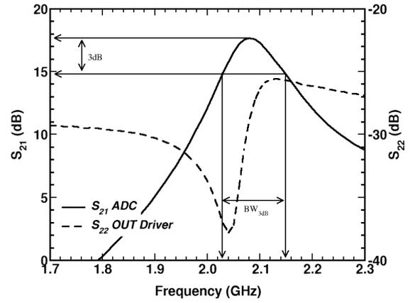
Fig. 5. Measured ADC single-ended S-parameters.
