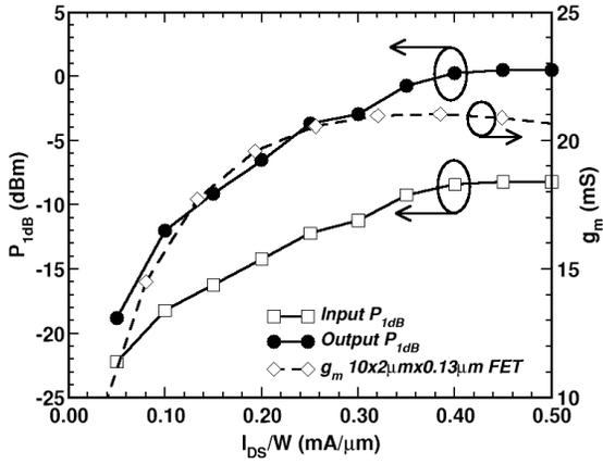
Fig. 3. Measured filter linearity and  $g_m$  of n-MOSFET vs current density.
