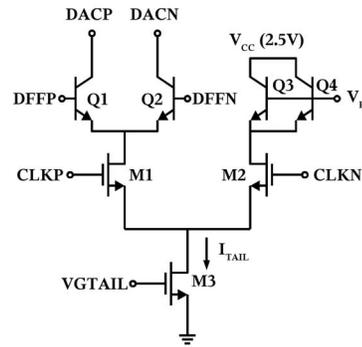
Fig. 4. Circuit schematic of RZ DAC.
