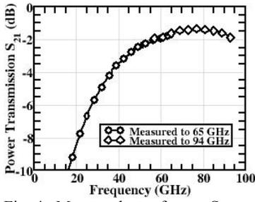
Fig. 4. Measured transformer  $S_{21}$ .
