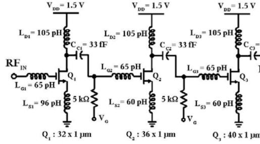
Fig. 5. 60-GHz PA schematic.
