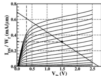
Fig. 3. Optimal load line for 90-nm CS n-MOSFET stage on measured I-V characteristic. The breakdown voltage is larger than 3V.
