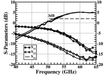
Fig. 10. Measured PA S-parameters across 3 different dice.
