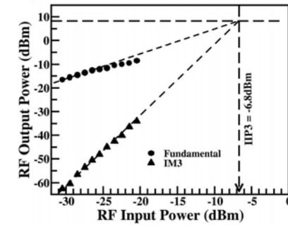
Fig. 15. Measured LNA IIP3 with 50-MHz tone spacing.
