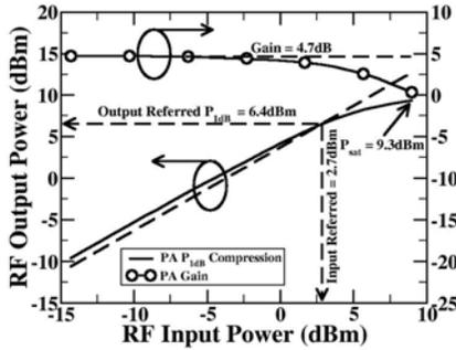
Fig. 11. Measured PA  $P_{1dB}$  at 60GHz.
