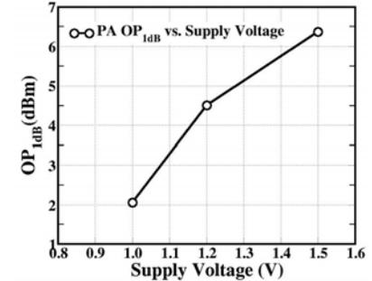
Fig. 13. Measured PA  $P_{1dB}$  vs. supply at 60GHz.
