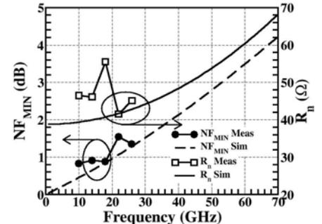
Fig. 16. Meas. vs. sim.  $NF_{MIN}$ ,  $R_n$  for a 40 x 90nm x 1  $\mu\text{m}$  n-MOS cascode.
