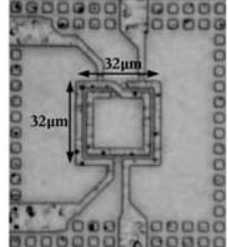
Fig. 7. Stacked 32  $\mu\text{m}$  x 32  $\mu\text{m}$  transformer in 90-nm RF-CMOS.
