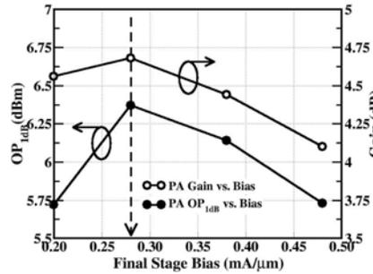
Fig. 12. Measured PA  $P_{1dB}$ , gain vs. final stage bias at 60GHz.
