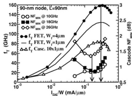
Fig. 1. Measured cascode  $f_T$ ,  $NF_{\text{MIN}}$  vs. bias.
