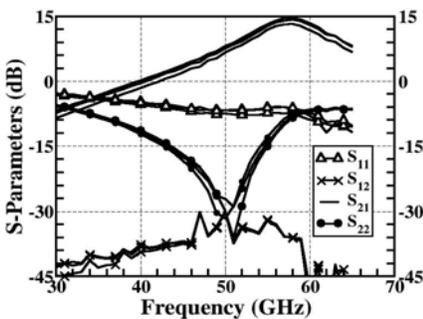
Fig. 14. Measured LNA S-parameters across 3 different dice.
