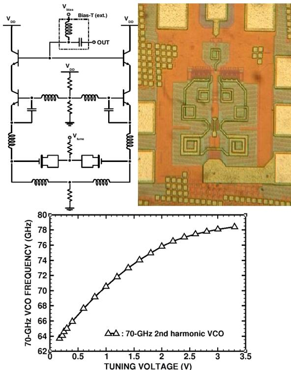
**Figure 9.** Schematics, layout and tuning characteristics of push-push SiGe-HBT VCO.
