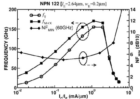
Figure 1. Measured  $f_T$ ,  $f_{MAX}$  and  $NF_{MIN}$  at 60 GHz as functions of current density in SiGe HBTs.
