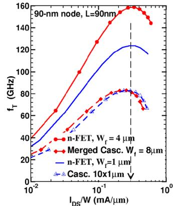
Figure 3. Measured  $f_T$  as a function of drain current density for 90-nm MOSFETs and cascodes.
