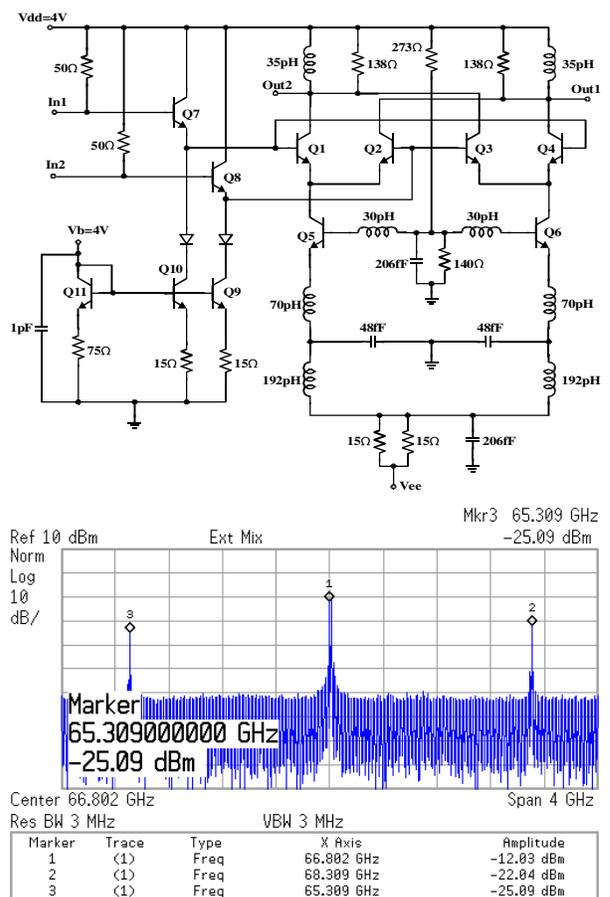
**Figure 10.** Schematics and measured spectrum at the output of 65-GHz BPSK transmitter for a 1.5 GHz data input.
