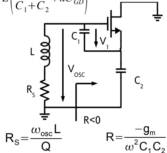
$$L(f_m) = \frac{|I_n|^2}{V_{osc}^2} \times \frac{1}{f_m^2} \times \frac{1}{C_1^2 \left( \frac{C_1}{C_2} + 1 \right)^2}$$
