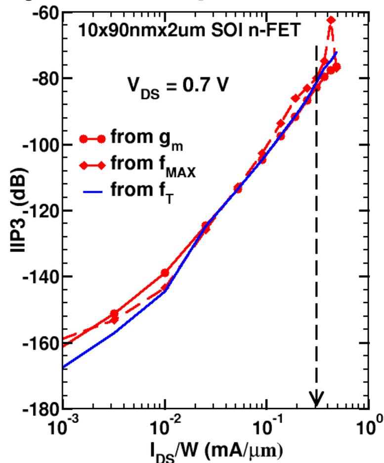
$$OIP3 \sim \frac{f_{MAX}}{\frac{\partial^2 f_{MAX}}{\partial V_{GS}^2}} \text{ vs. } \frac{g_m}{\frac{\partial^2 g_m}{\partial V_{GS}^2}}$$
