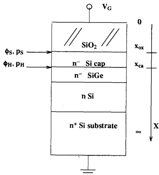
Fig. 1. Si/Si<sub>1-x</sub>Ge<sub>x</sub> MOS capacitor used as test structure. Notations used for hole concentration and electric potential at the top heterojunction and at the Si/SiO<sub>2</sub> interface are also shown.
