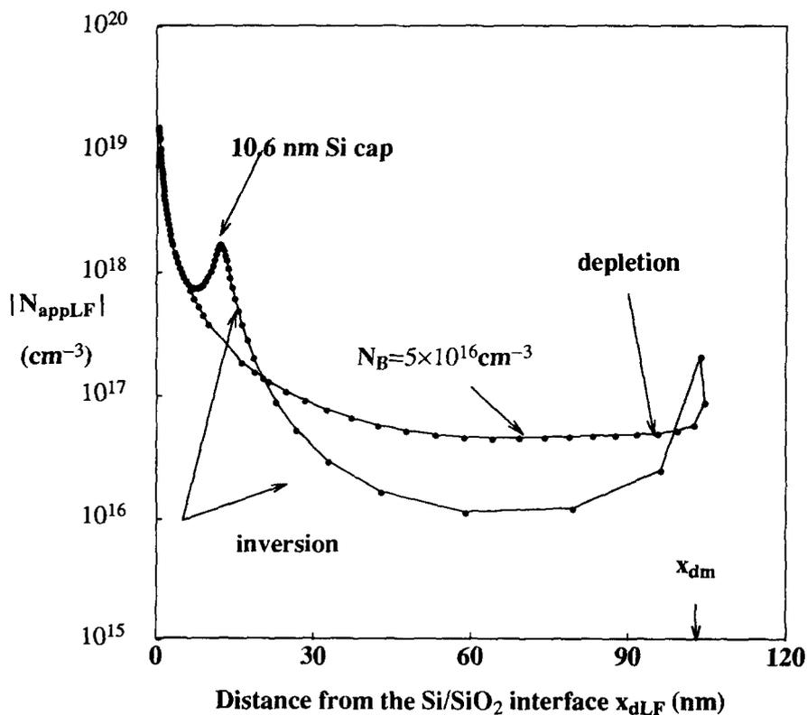
Fig. 5. Low frequency apparent doping vs depth profiles in  $\text{Si/Si}_{1-x}\text{Ge}_x$  MOS capacitors obtained from the simulated  $C_{LF}-V_G$  characteristics of Fig. 3.
