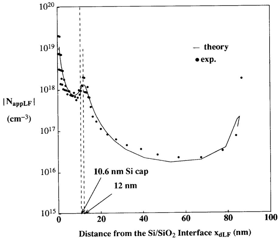
Fig. 10. Simulated and experimental apparent doping vs depth profiles. The experimental data are obtained from the inversion region of the measured  $C_{LF}-V_G$  characteristics of Fig. 6. The size-quantization-induced offset between the cap layer and the position of the hole charge centroid is also illustrated.
