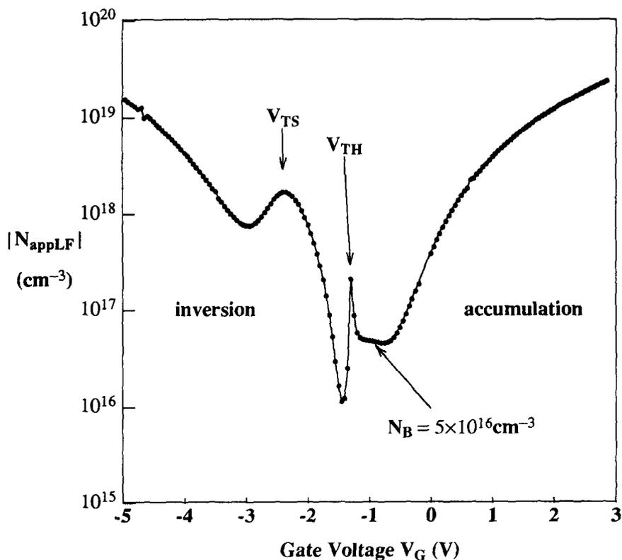
Fig. 4. Low frequency apparent doping vs gate voltage characteristics for a  $\text{Si/Si}_{1-x}\text{Ge}_x$  MOS determined from the simulated  $C_{LF}-V_G$  characteristics of Fig. 3.
