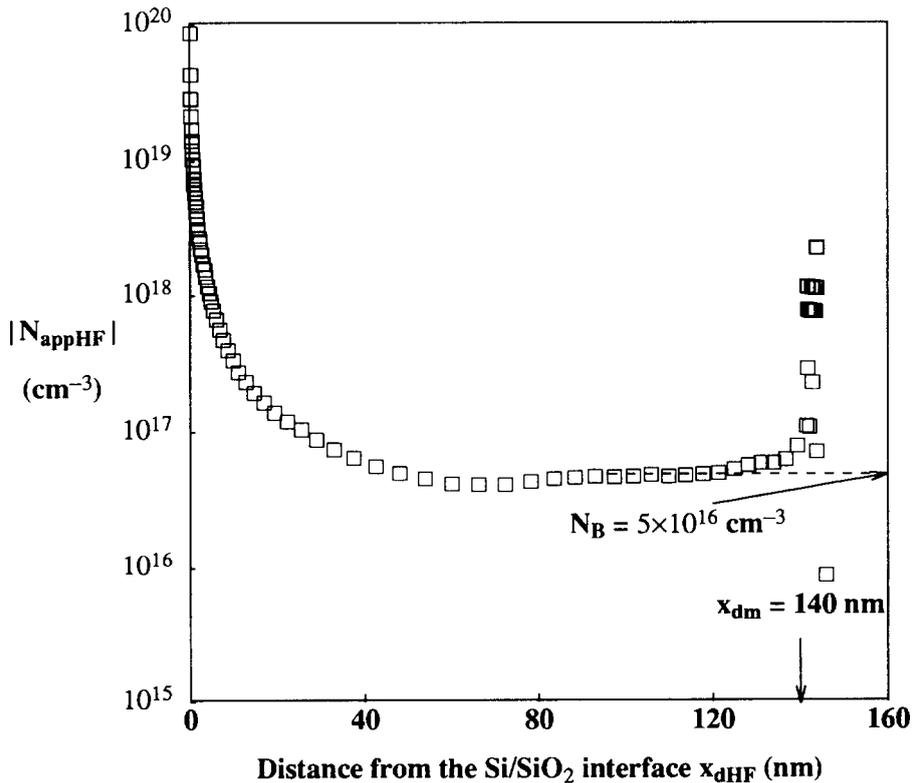
Fig. 7. Experimental high frequency apparent doping vs depth profiles in  $\text{Si/Si}_{1-x}\text{Ge}_x$  MOS capacitors obtained from the measured  $C_{HF}-V_G$  characteristics of Fig. 6.
