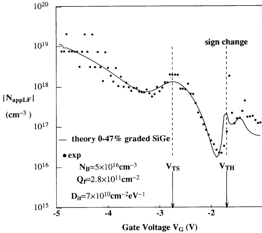
Fig. 9. Simulated and experimental apparent doping vs gate voltage characteristics for a graded 0–47% Ge Si/Si<sub>1-x</sub>Ge<sub>x</sub> MOS capacitor as determined from the measured  $C_{LF}-V_G$  characteristics shown in Fig. 6.
