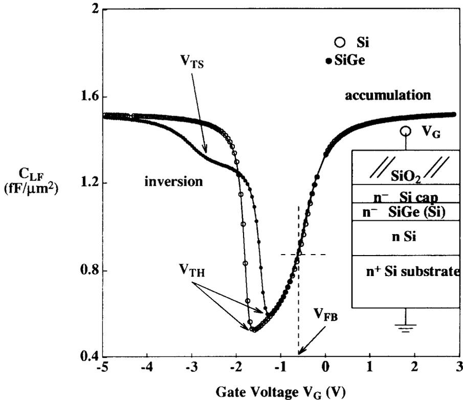
Fig. 3. Comparison of simulated  $C_{LF}$ - $V_G$  characteristics of Si and Si/Si<sub>1-x</sub>Ge<sub>x</sub> MOS capacitors with layer structure shown in the inset.
