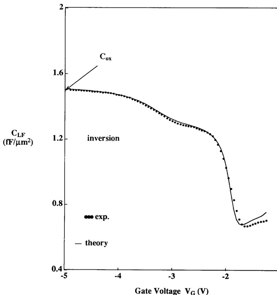
Fig. 8. Comparison of measured and simulated  $C_{\text{LF}}-V_G$  characteristics of  $\text{Si/Si}_{1-x}\text{Ge}_x$  MOS capacitors based on extracted structural and material data.
