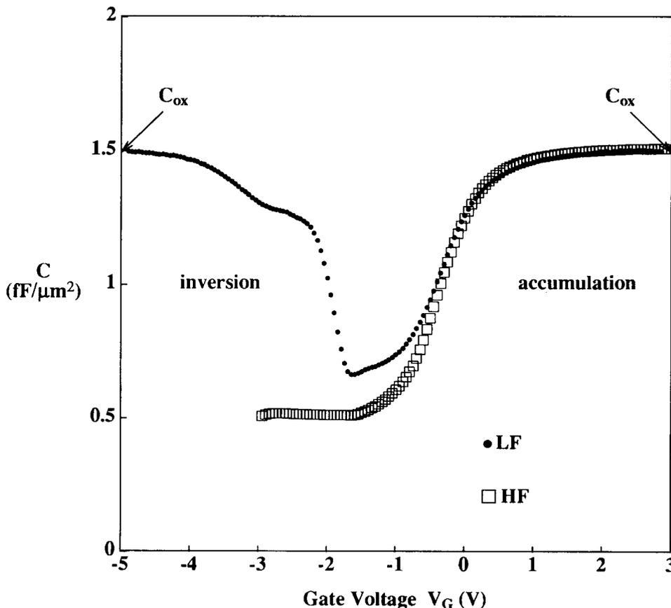
Fig. 6. Typical experimental  $C_{HF}-V_G$  and  $C_{LF}-V_G$  characteristics of graded (0–47% Ge) Si/Si<sub>1-x</sub>Ge<sub>x</sub> MOS capacitors. The structure is similar to that presented in Fig. 3.
