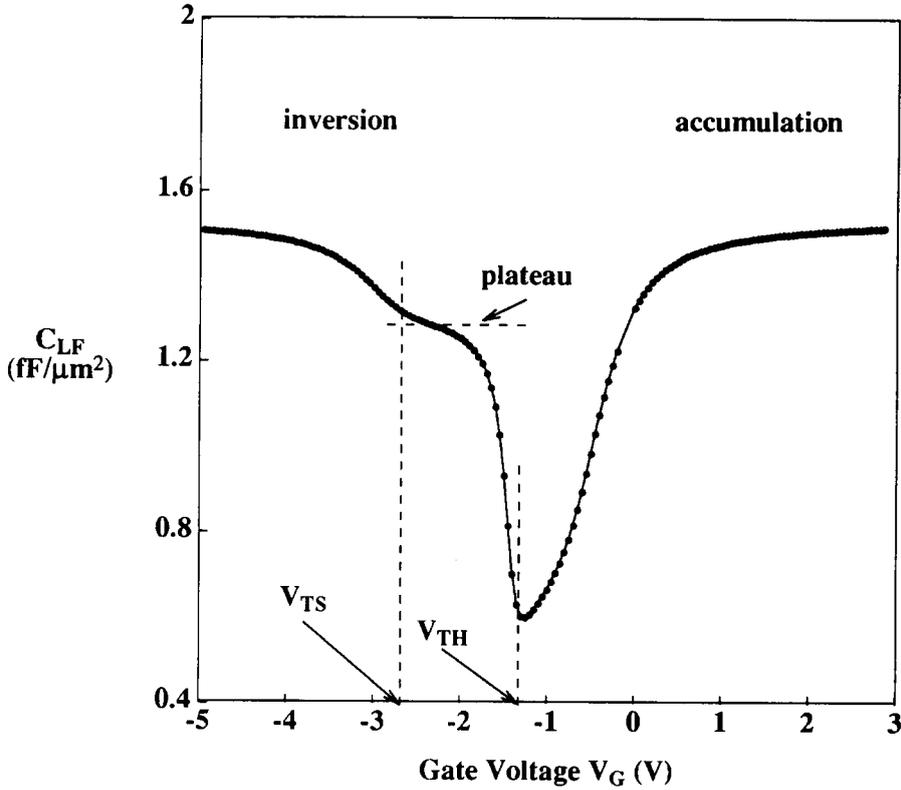
Fig. 2. Typical  $C_{LF}$ - $V_G$  characteristics of Si/Si<sub>1-x</sub>Ge MOS capacitors showing threshold voltages and capacitance plateau.
