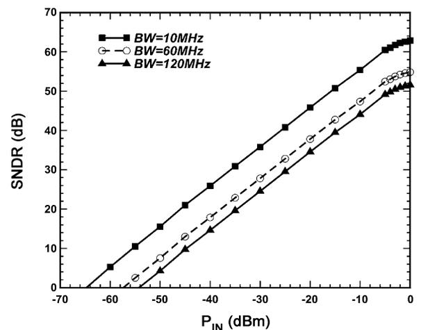
Fig. 21. Measured dynamic range for a 2-GHz single tone input.
