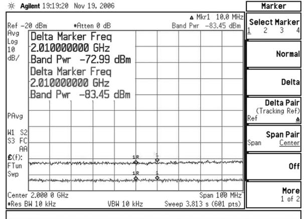
Fig. 19. Measured noise floor at the ADC output (top trace). The noise floor of the ADC drops from  $-73$  dBm to  $-83.45$  dBm (bottom trace) when the feedback is off, indicating that quantization noise is limiting the ADC.
