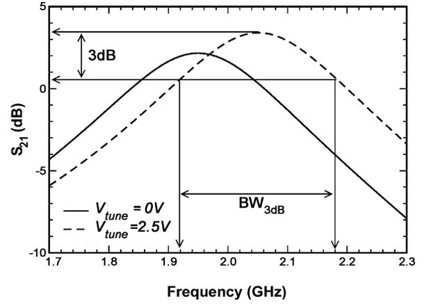
Fig. 6. Measured  $S_{21}$  of the filter test structure.
