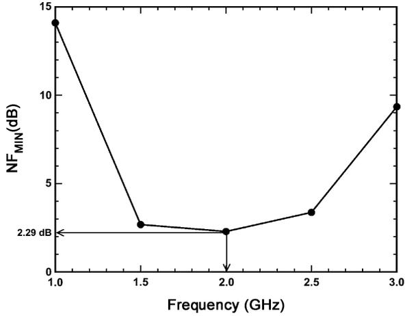
Fig. 7. Measured  $NF_{MIN}$  of the filter test structure.
