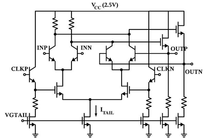
Fig. 11. Circuit schematic of latch.
