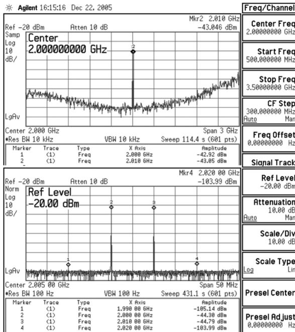
Fig. 23. Measured ADC two-tone spectra at 2 GHz with  $P_{IN} = -30$  dBm.
