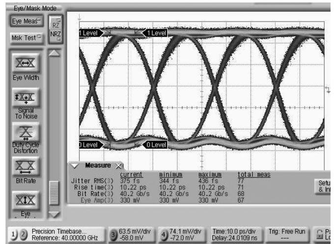
Fig. 17. Measured output eye diagram at 40 Gb/s.
