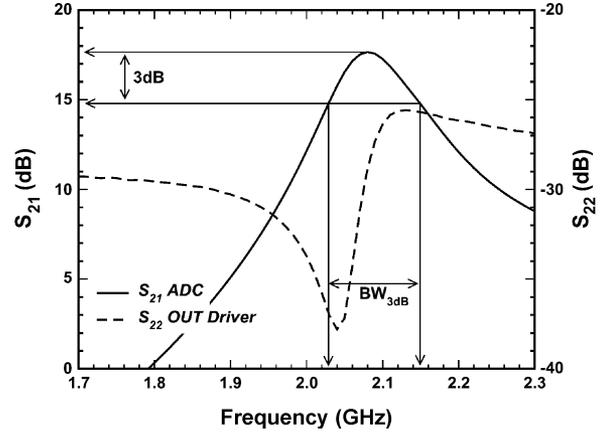
Fig. 16. Measured ADC single-ended S-parameters.
