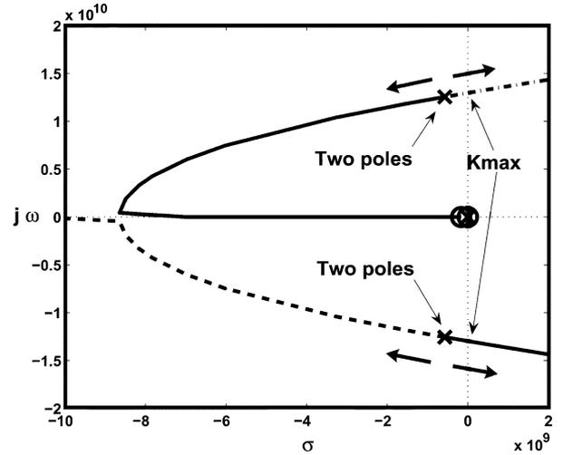
Fig. 3. Root locus of fourth-order bandpass  $\Delta\Sigma$  ADC.
