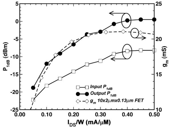
Fig. 8. Measured filter linearity and  $g_m$  of nMOSFET versus current density.
