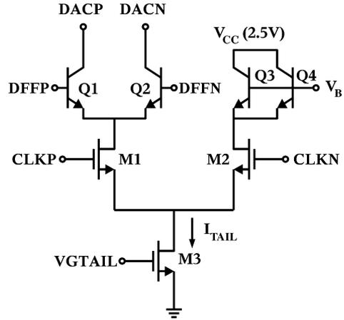
Fig. 10. Circuit schematic of RZ DAC.
