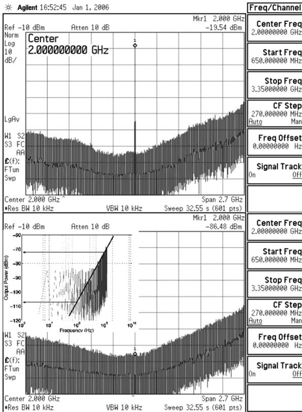
Fig. 18. Measured ADC output spectrum with and without a 2-GHz input sinusoid.
