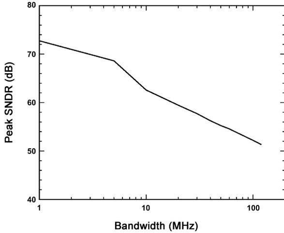
Fig. 22. Measured peak SNDR versus bandwidth for a 2-GHz single tone input.
