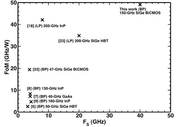
Fig. 24. Comparison of mm-wave  $\Delta\Sigma$  ADCs.
