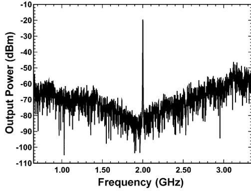
Fig. 14. Simulated ADC spectrum ( $N_{\text{FFT}} = 32768$ ).
