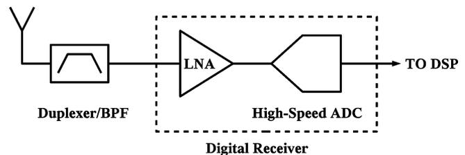
Fig. 1. Top level architecture of a digital receiver.
