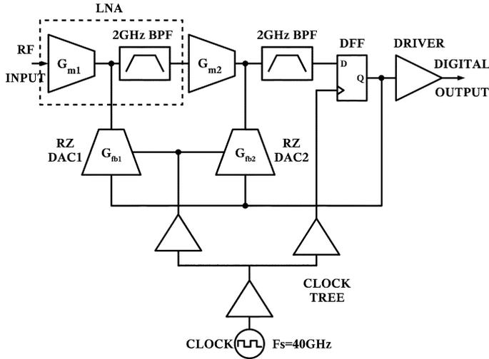
Fig. 2. System-level ADC block diagram.
