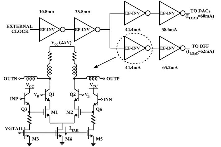
Fig. 12. Block diagram of clock distribution tree and schematic of emitter-follower MOS-HBT inverter.
