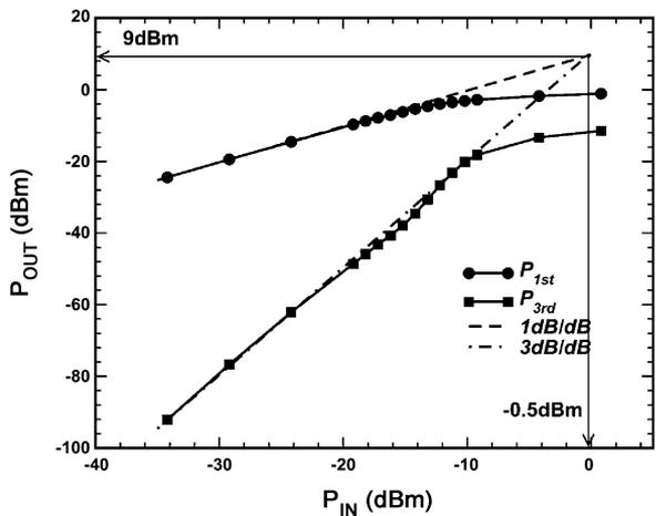
Fig. 9. Measured IP3 of the filter test structure.
