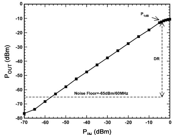
Fig. 20. Measured output versus input power of the ADC for a 2-GHz single-tone input.
