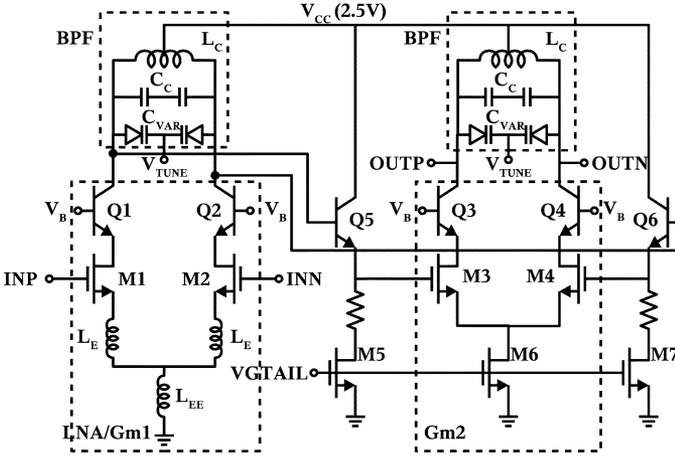
Fig. 5. Circuit schematic of 2-stage loop filter.
