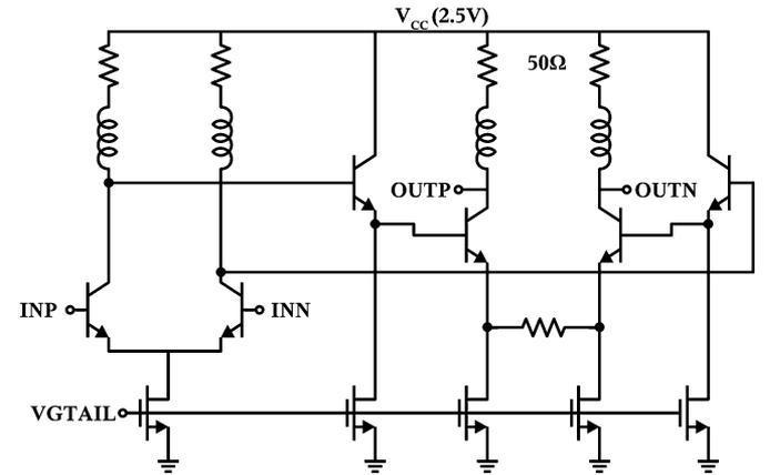
Fig. 13. Circuit schematic of 50- $\Omega$  output driver.
