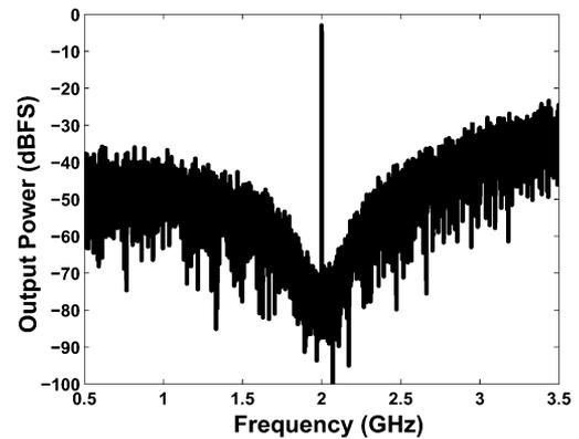
Fig. 4. System-level simulation of  $\Delta\Sigma$  ADC ( $N_{\text{FFT}} = 65536$ ).
