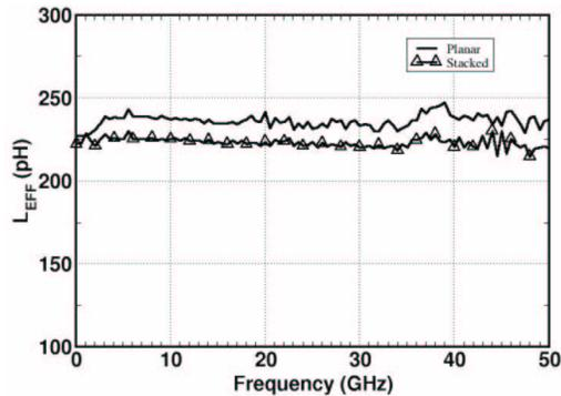
Fig. 3. Measured  $L_{\text{EFF}}$  for 220-pH planar and stacked inductors.
