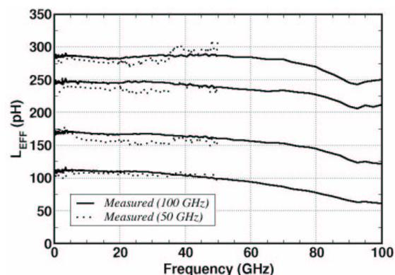
Fig. 1.  $L_{\text{EFF}}$  for planar mm-wave inductors measured using 50-GHz and 100-GHz network analyzer systems.
