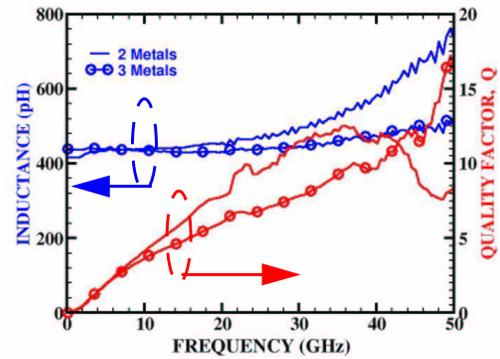
Fig. 5. Measured  $L_{\text{EFF}}$  and Q of 420-pH stacked inductors implemented in two and three metal layers.
