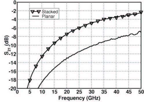
Fig. 9. Comparison of stacked and planar mm-wave transformers.
