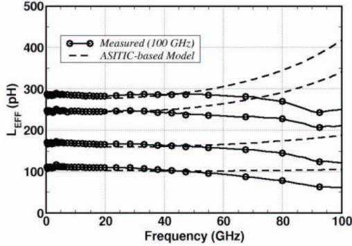
Fig. 11. Measured and ASITIC-modeled  $L_{EFF}$  to 100 GHz.
