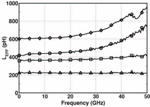
Fig. 2. Measured  $L_{\text{EFF}}$  of mm-wave stacked inductors.
