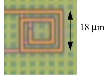
Fig. 4. Die photo of 220-pH 2-metal stacked inductor.
