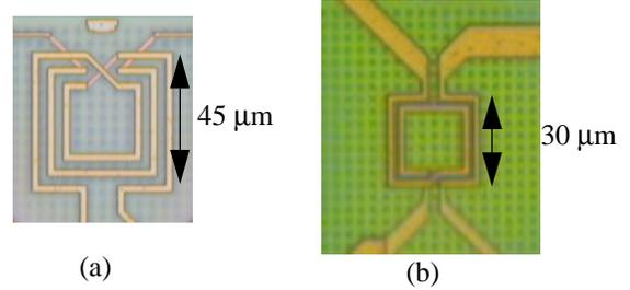
Fig. 8. Die photos of mm-wave transformers (a) planar and (b) stacked.
