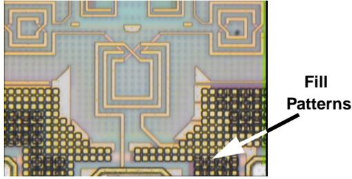
Fig. 6. CMP fill patterns near mm-wave inductors and transformer.
