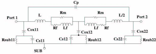
Fig. 10. Double- $\Pi$  inductor model.
