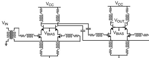
Fig. 7 Clock buffer with transformer for single-ended-to-differential conversion (biasing omitted for clarity)
