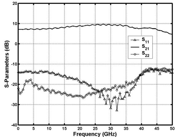
Fig. 9 Measured  $S$ -parameters of input amplifier and output driver
