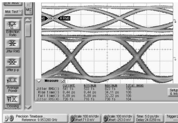
Fig. 11 Input (top) and output 40-Gb/s eye diagrams
