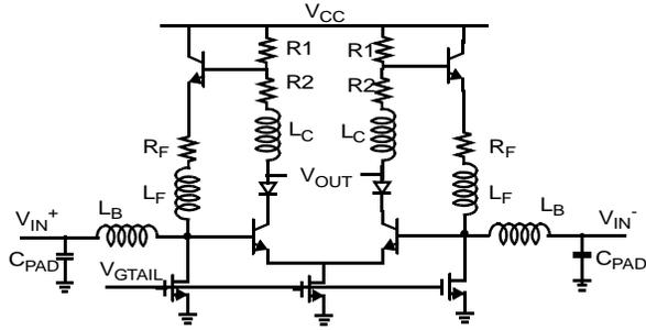
Fig. 6 Transimpedance voltage preamplifier
