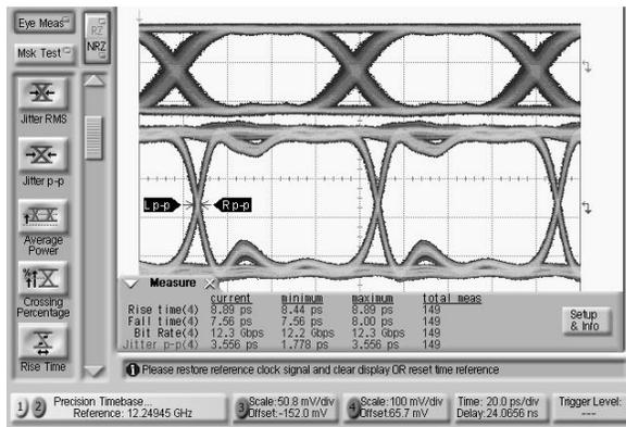
Fig. 10 Input (top) and output 12.5-Gb/s eye diagrams with 37.5-GHz clock signal.
