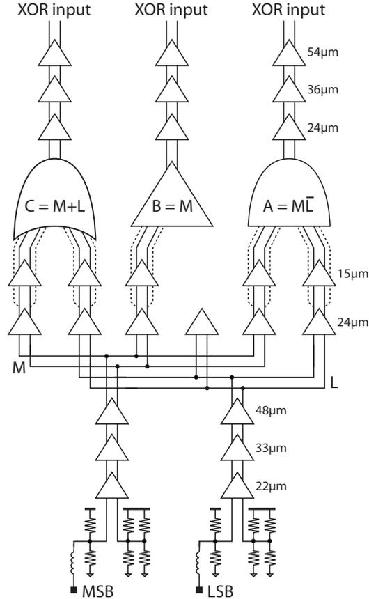
Figure 4.20: Data distribution circuits
