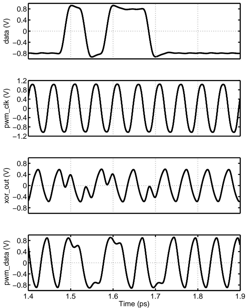
Figure 4.16: Simulated transient waveforms for XOR stage with high-gain buffers
