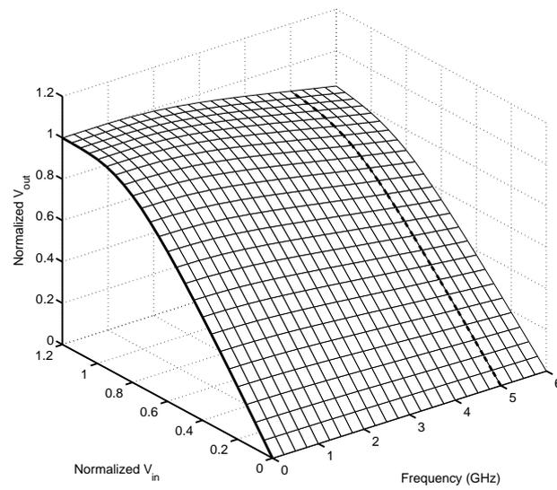
Figure 3.10: VTCs of design IV:  $W = 17\mu m$ ,  $\Delta V_{MAX} = 800mV$
