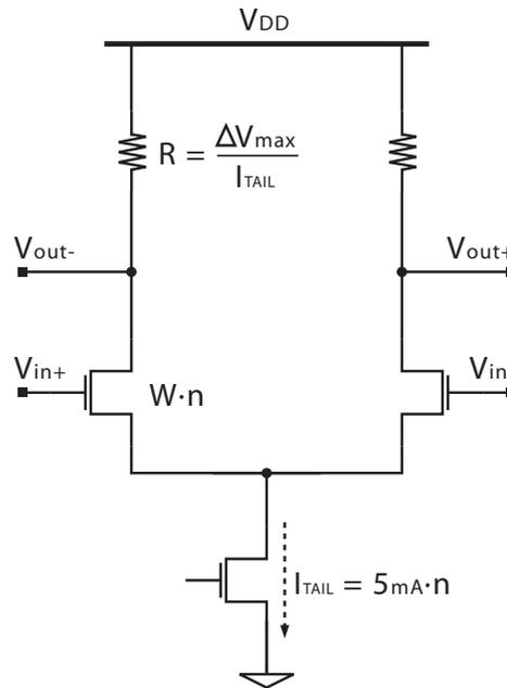
(b) Schematic of CML buffer used for circuit simulation
