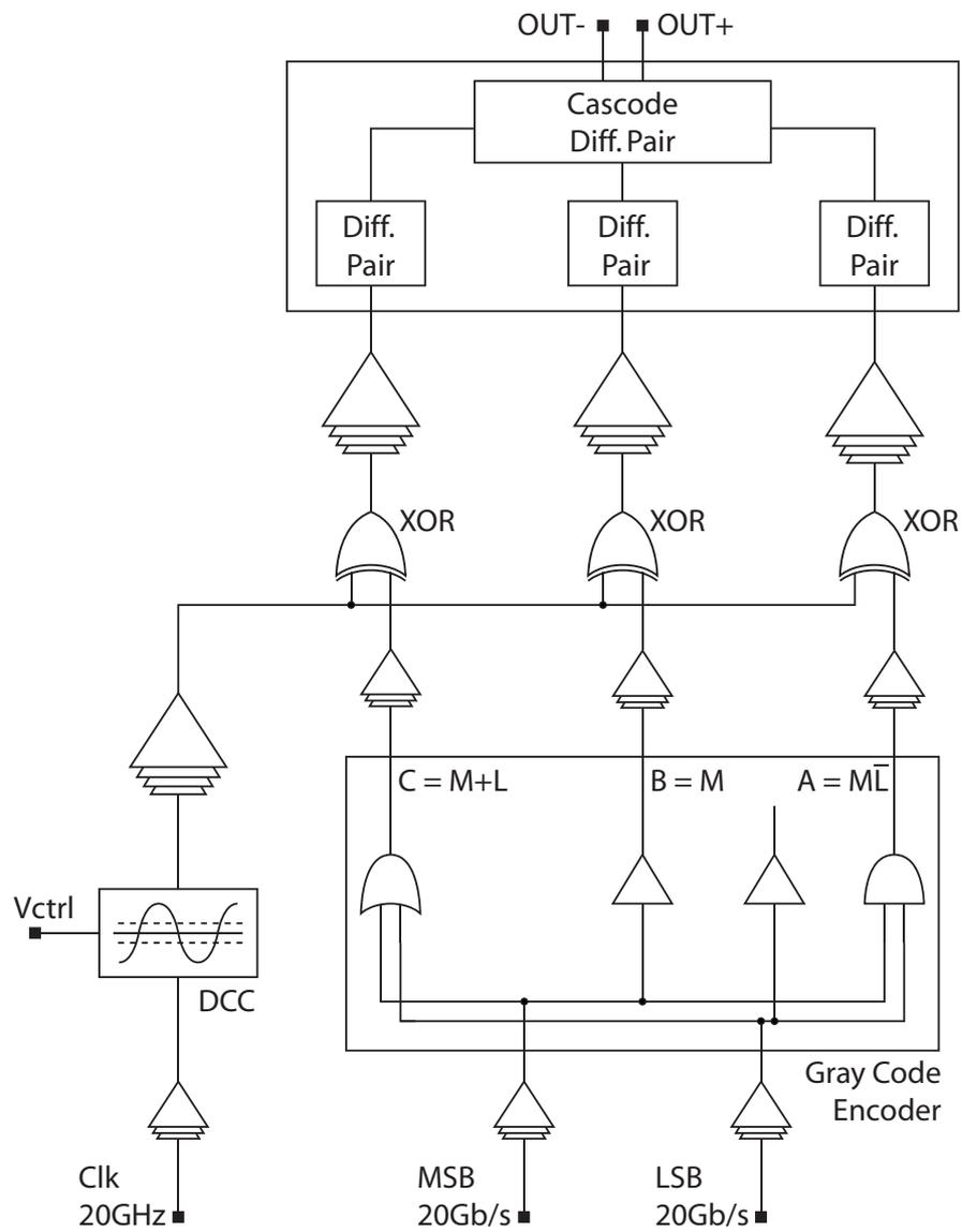
Figure 4.3: Block diagram of transmitter
