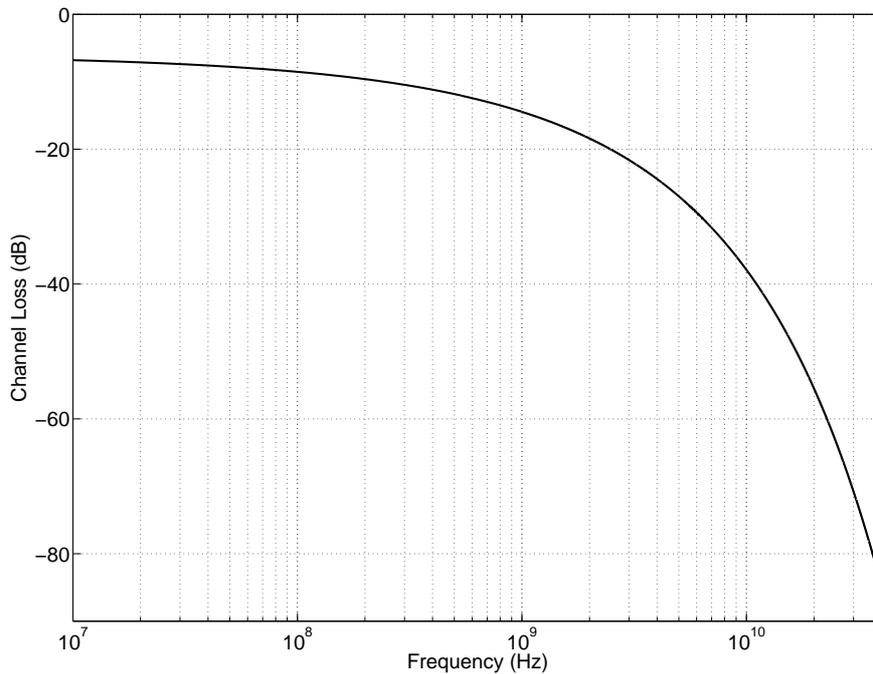
Figure 2.1: Channel loss characteristic of 1694A coaxial cable of length 40m
