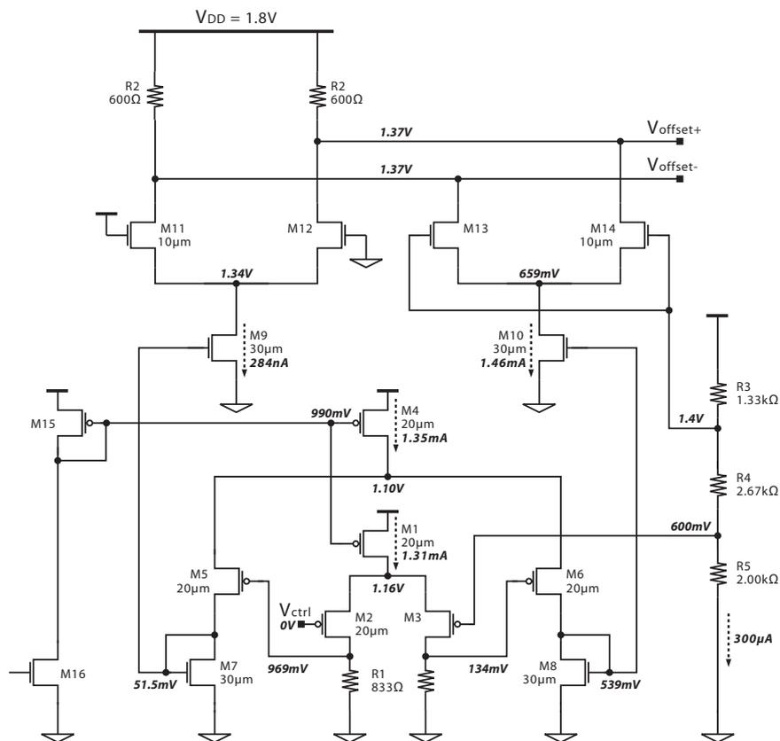
(a) DCC offset control circuit schematic
