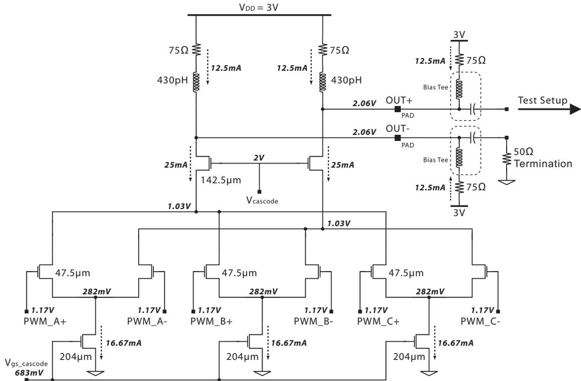
Figure 4.17: Schematic of Cascode stage
