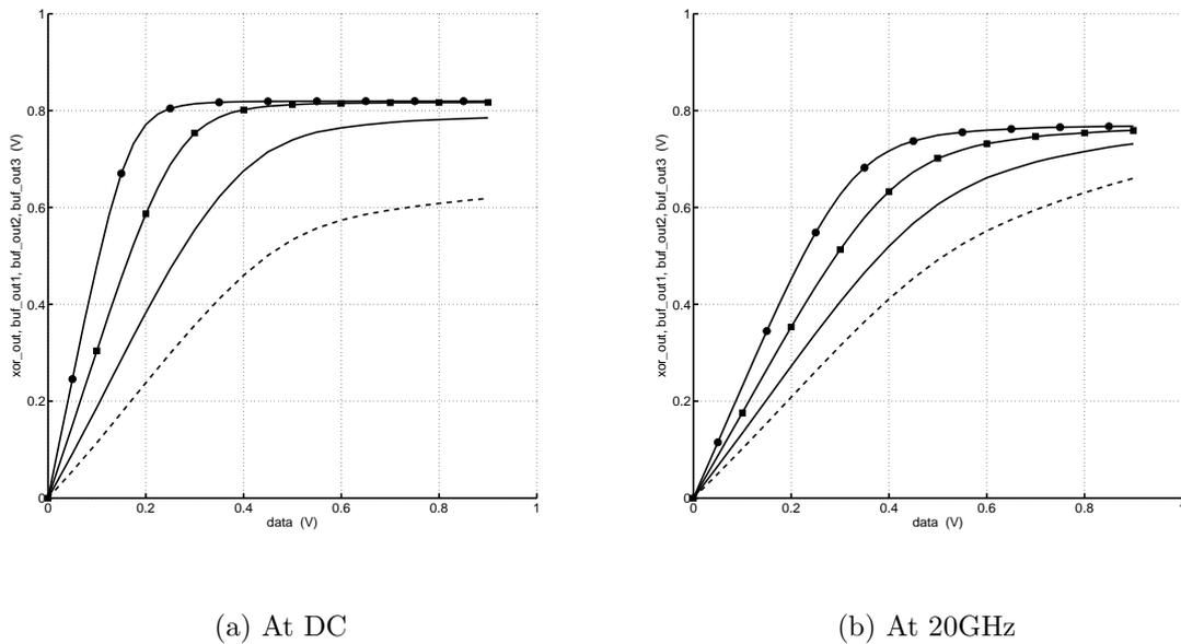
Figure 3.17: VTCs of XOR CML circuit with high gain buffers; *xor\_out*(dashed), *buf\_out1*(solid), *buf\_out2*(square marker), *buf\_out3*(circular marker)
