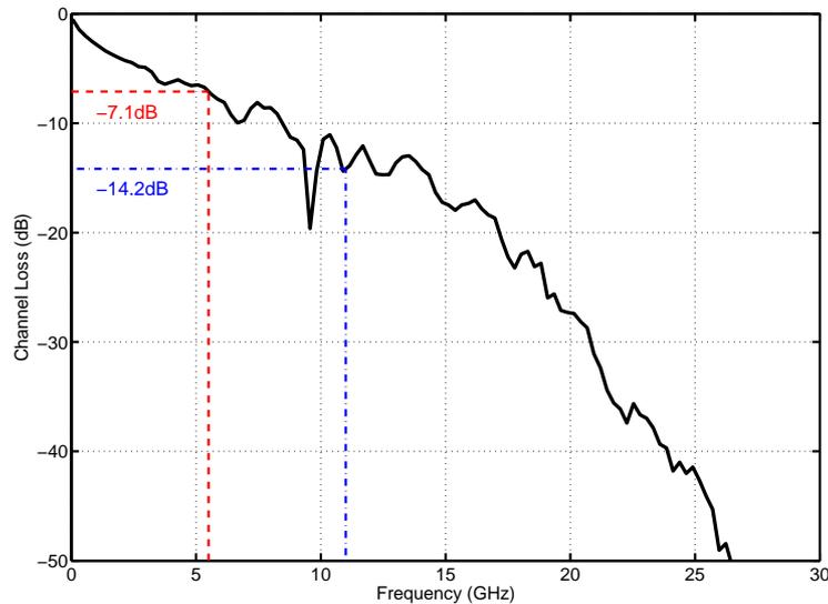
Figure 5.20: Channel A loss curve and channel loss at 5.5GHz and 11GHz
