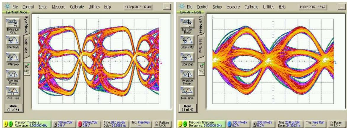
(a) Eye diagram at output of transmitter
