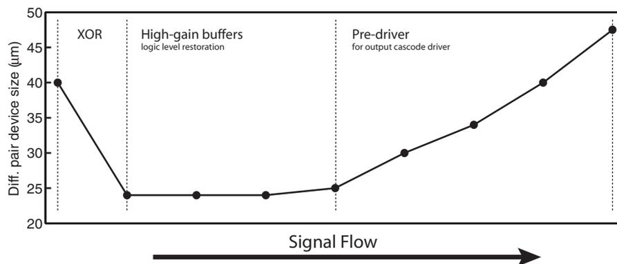
(b) Differential pair device widths from XOR to output driver
