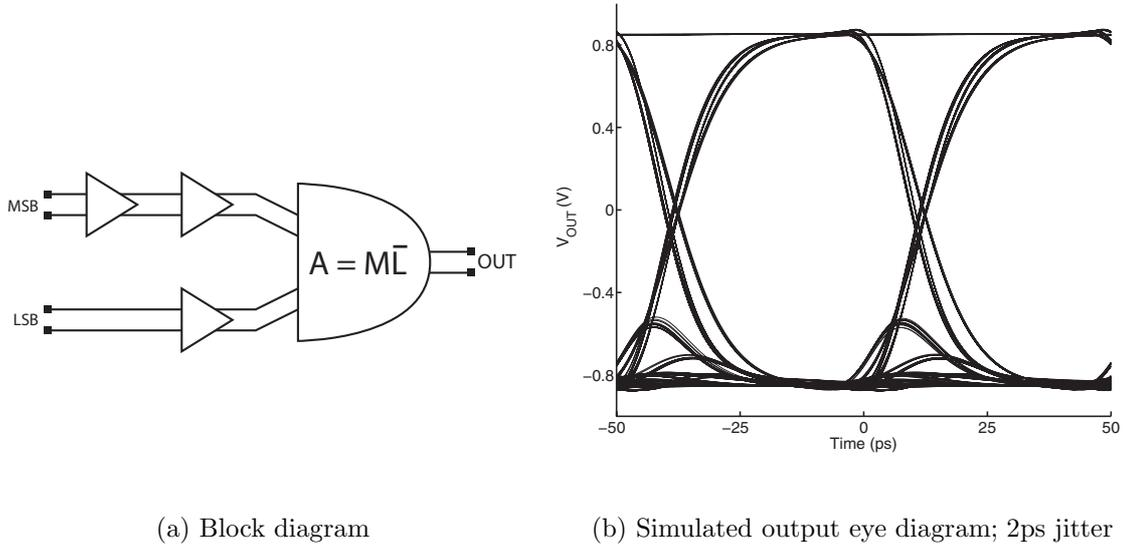
Figure 4.11: Design with early LSB input for  $A = M \cdot \bar{L}$
