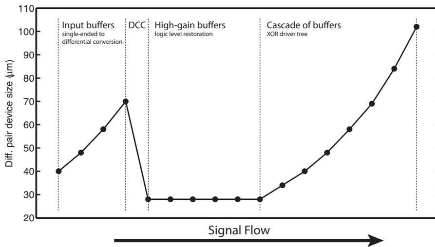
(b) Differential pair device widths along clock distribution network
