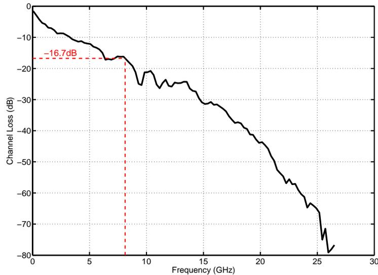
Figure 5.9: Channel B loss curve
