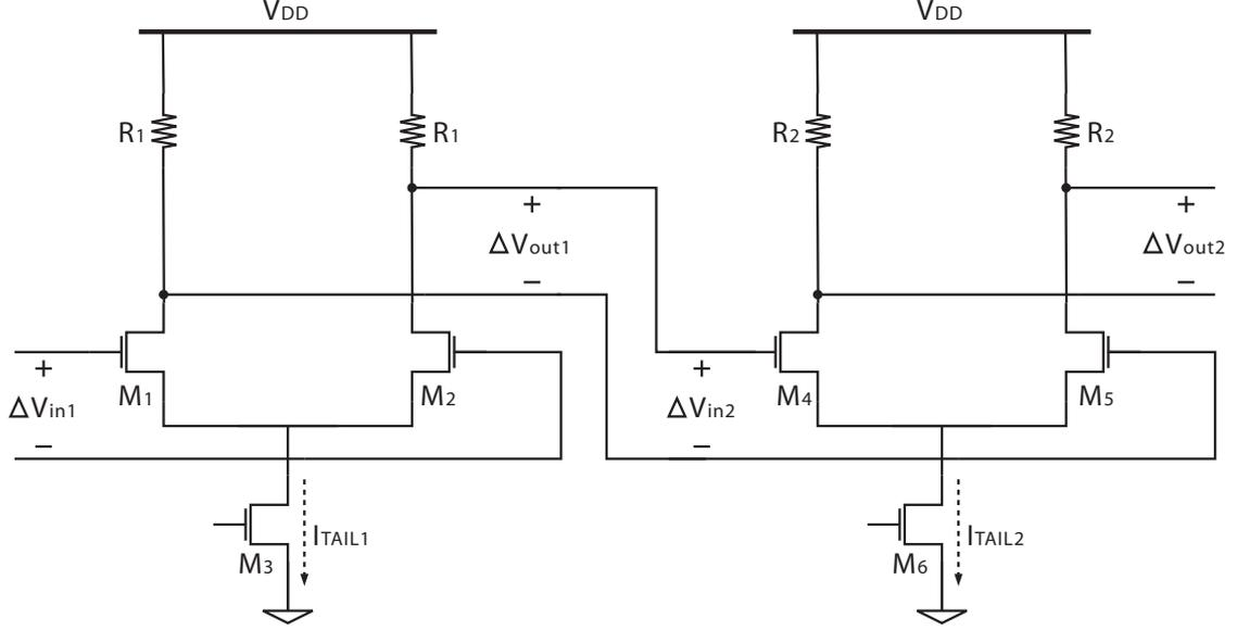
Figure A.2: Schematics of two CML buffers connected in cascade
