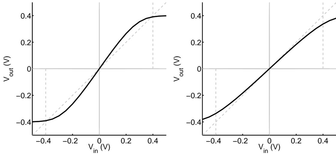
(a) Design I:  $W = 54\mu m$ ,  $\Delta V_{MAX} = 400mV$
