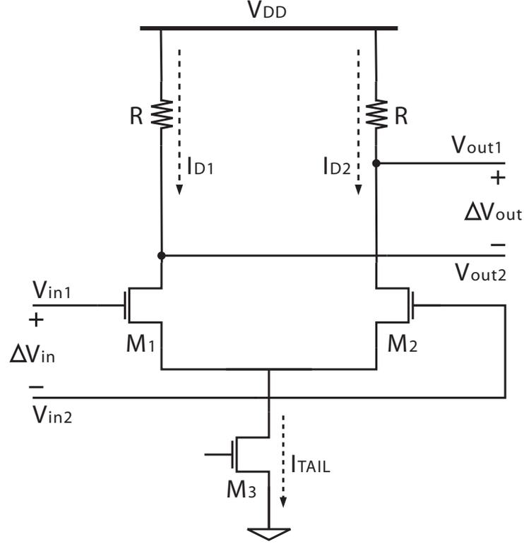
Figure A.1: Schematics of a CML buffer
