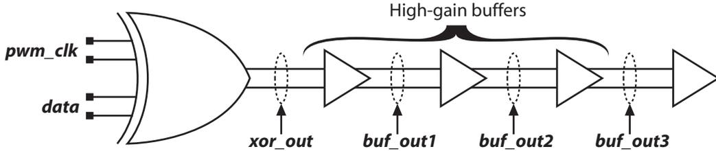
Figure 3.14: Block diagram of XOR CML circuit with high gain buffers
