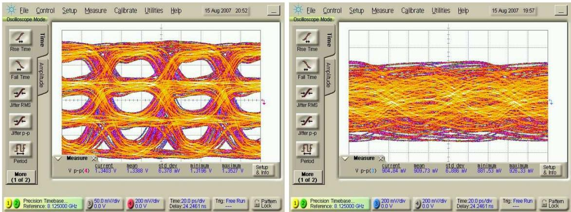
(a) Eye diagram at output of transmitter
