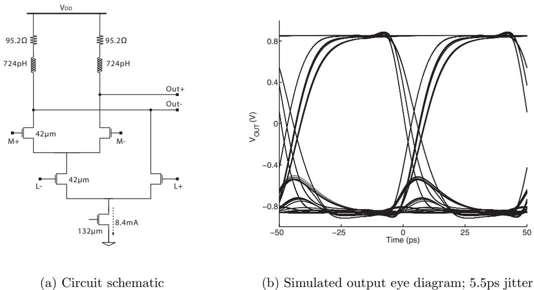
Figure 4.9: Basic design for  $A = M \cdot \bar{L}$
