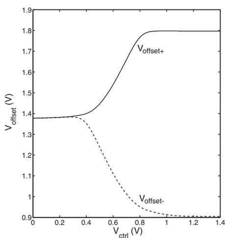
(b) Tuning curve: Single-ended outputs  $V_{offset+}$  &  $V_{offset-}$
