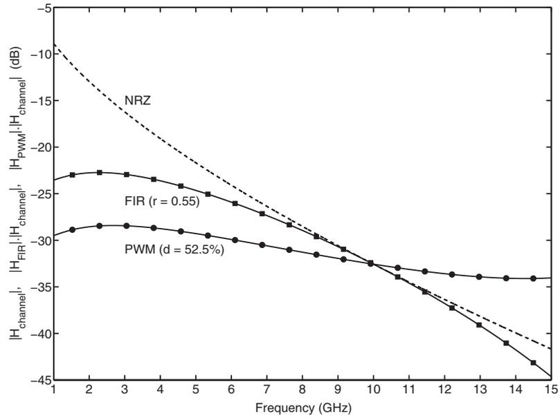
Figure 2.6: Combined pre-emphasis and channel response for FIR-PE and PWM-PE
