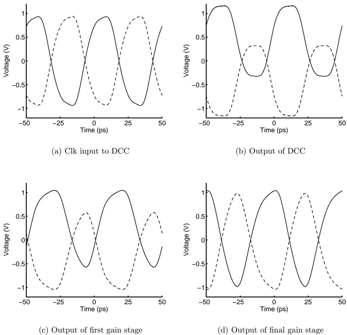
Figure 4.8: DCC and high-gain buffer waveforms; dotted line is inverted clock signal for eye diagram representation
