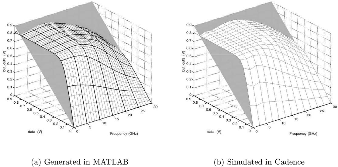
Figure 3.18: VTC of *buf\_out3* with  $V_{out} = V_{in}$  plane
