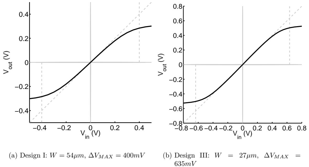
Figure 3.3: Frequency-dependent VTCs of CML buffers at 5GHz
