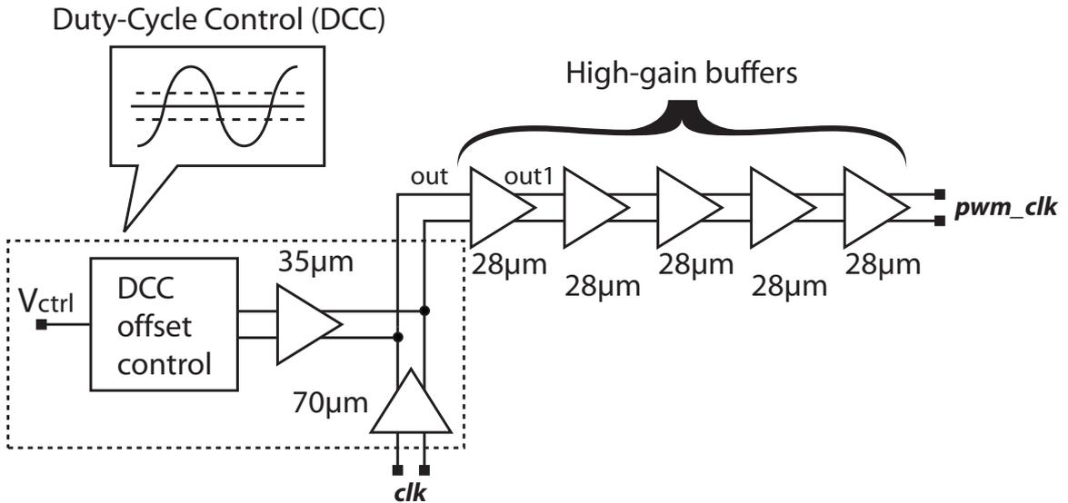
Figure 4.7: block diagram of DCC stage with high-gain buffers with the width of differential pair devices labeled for each stage
