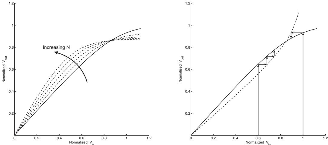
(a) VTCs of a cascade of soft-switching CML buffers; solid line - one stage VTC; dashed line - cascaded stage 2 to 5
