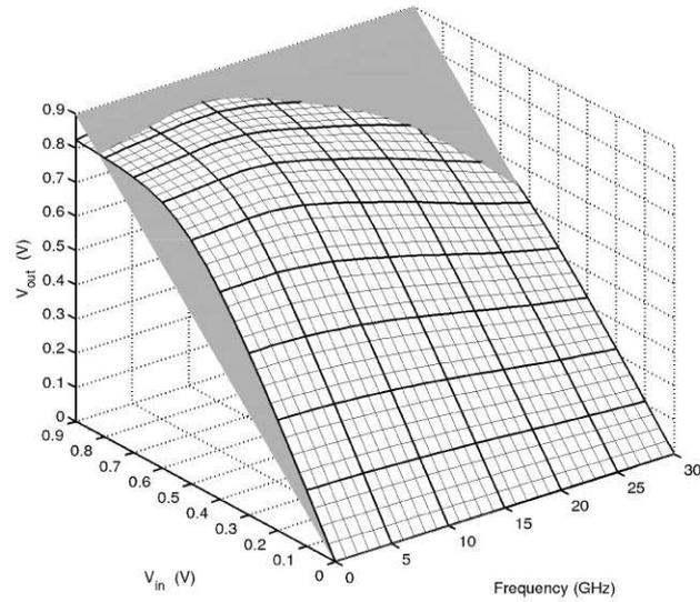
Figure 3.16: VTC of high-gain buffer with  $V_{out} = V_{in}$  plane
