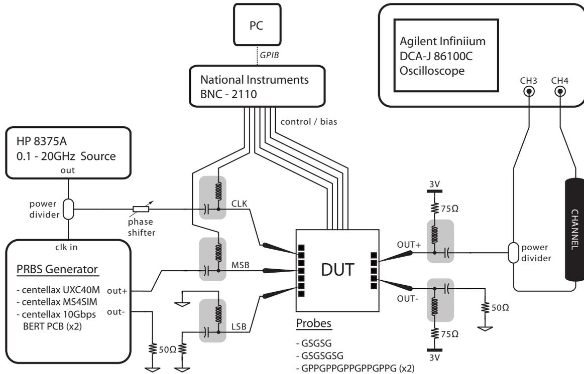
Figure 5.4: Binary mode measurement setup
