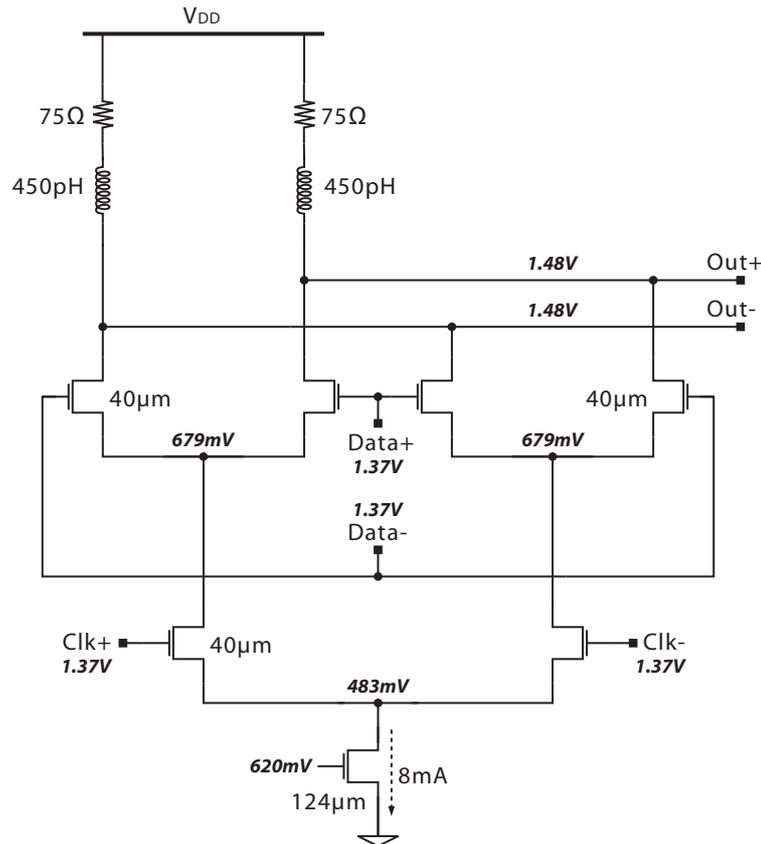
Figure 4.14: Schematic of XOR stage
