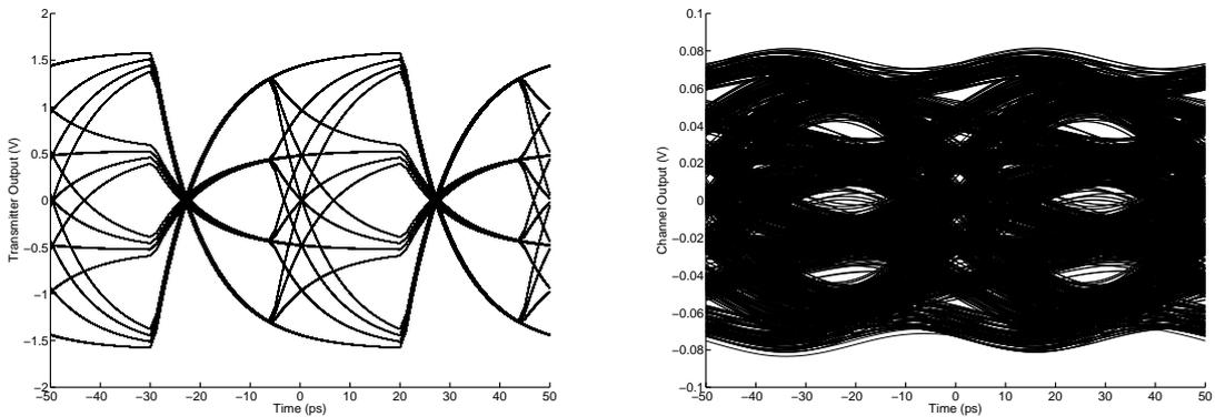
(a) Eye diagram of transmitter output with PWM-PE,  $d = 52.5\%$ ,  $T_{symbol} = 50ps$
