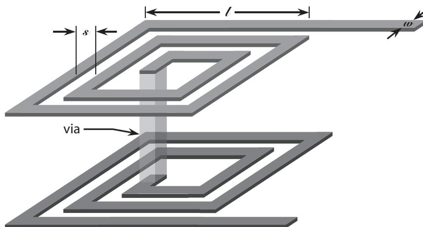
Figure B.1: Three-dimensional conceptual view of a two-layer metal spiral inductor
