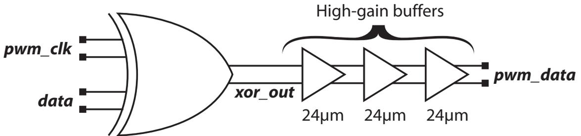
Figure 4.15: Block diagram of XOR stage with high-gain buffers
