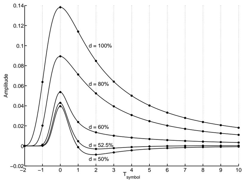
(b) Pulse response of PWM pre-emphasis at  $T_{symbol} = 50ps$ Figure 2.5: Pulse response after 40m of Belden 1694A coaxial cable at  $T_{symbol} = 50ps$
