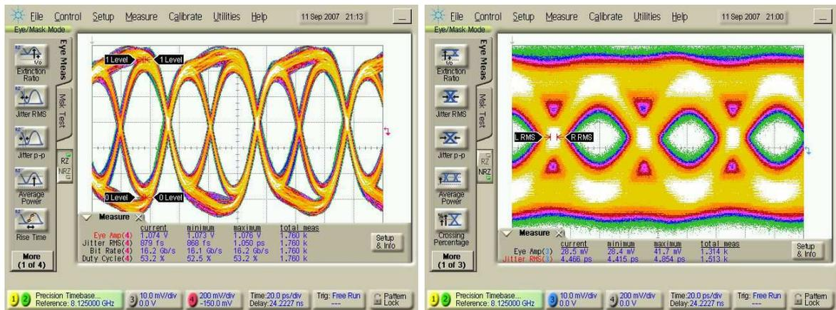
(a) Eye diagram at output of transmitter
