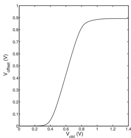
(c) Tuning curve: Differential output  $V_{offset} = V_{offset+} - V_{offset-}$
