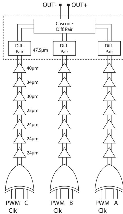
(a) Block diagram of PWM-PE and 4PAM generation circuits
