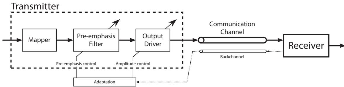
Figure 1.1: Transceiver Link
