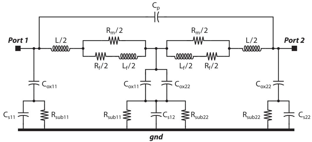
Figure B.2: Schematic of 2 –  $\pi$  inductor model used in ADS environment
