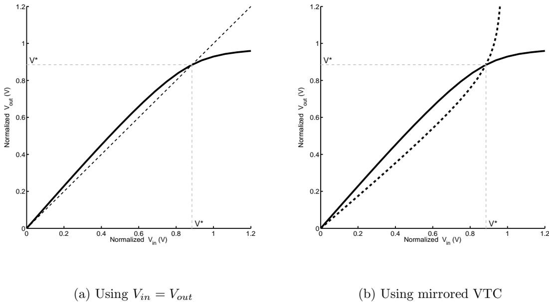
Figure 3.7: Two methods of obtaining  $V^*$  from VTC
