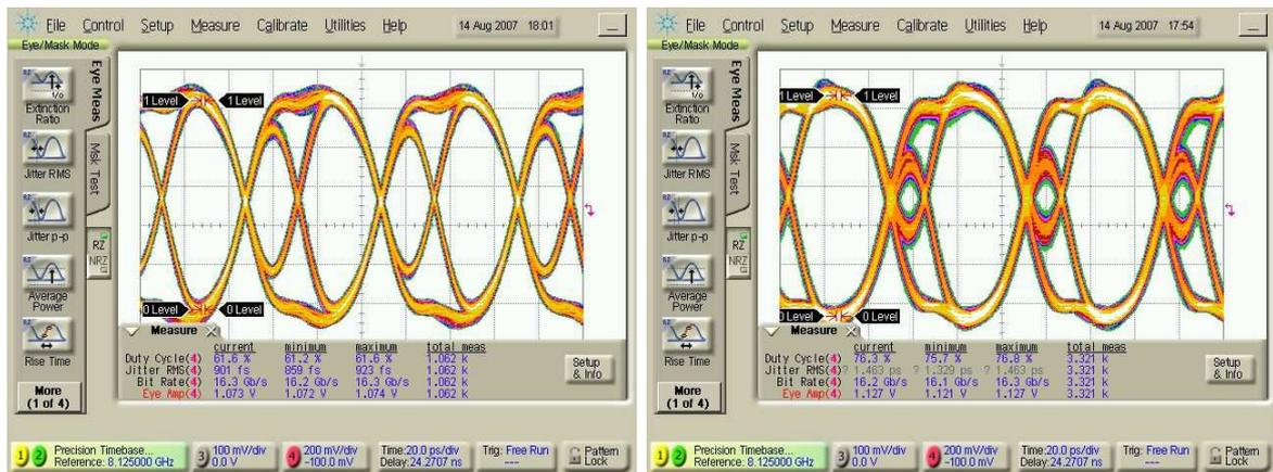
Figure 5.6: Transmitter output eye diagrams at 16.25Gb/s in binary transmit mode: Duty-cycle control
