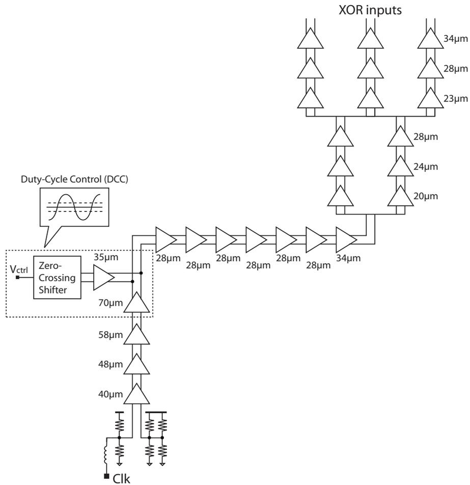
(a) Block diagram of clock distribution network
