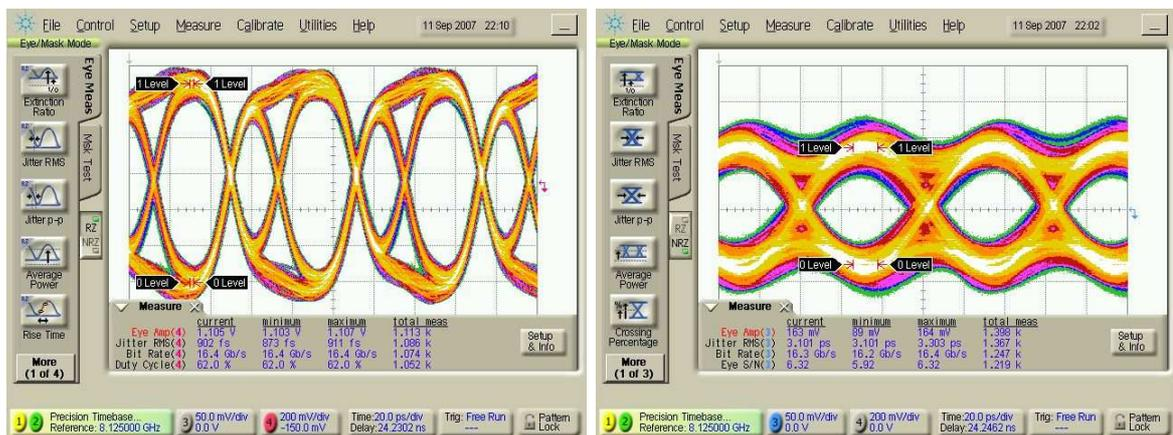
(a) Eye diagram at output of transmitter
