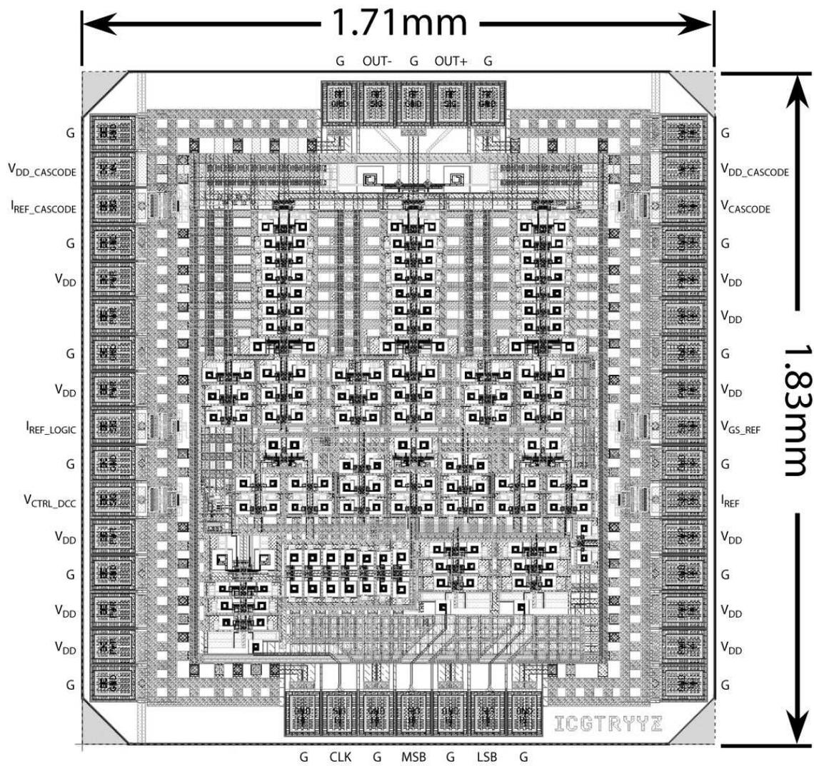
Figure 4.23: Layout of complete transmitter circuit
