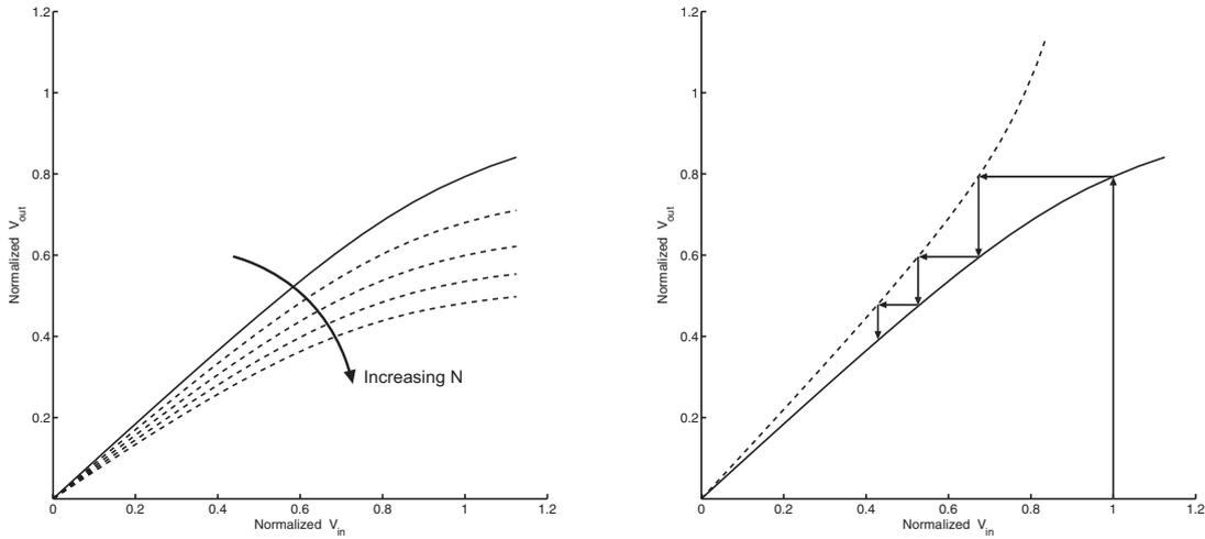
(a) VTCs of a cascade of attenuating CML buffers; solid line - one stage VTC; dash line - cascaded stage 2 to 5
