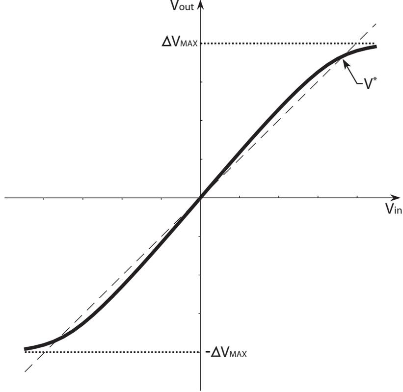
Figure 3.6: VTC of a CML circuit operating in soft-switching region
