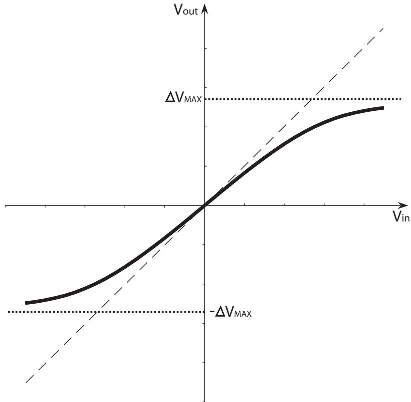
Figure 2.11: VTC of a CML circuit operating in attenuating region
