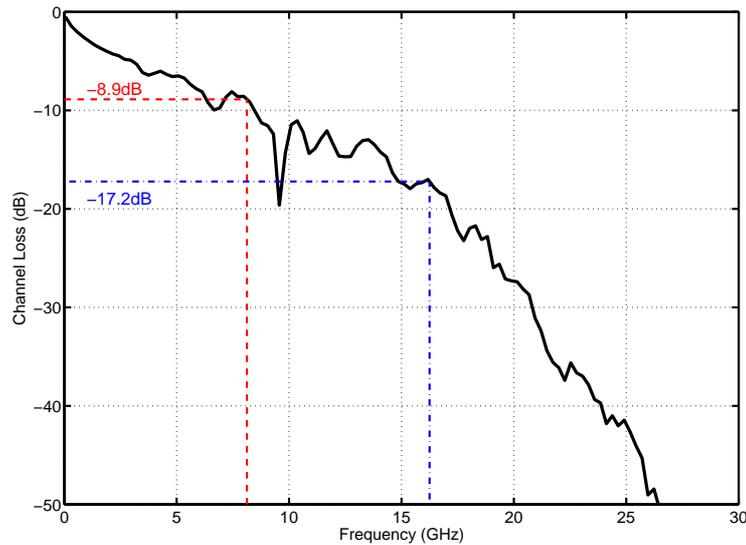
Figure 5.23: Channel A loss curve and channel loss at 8.125GHz and 16.25GHz
