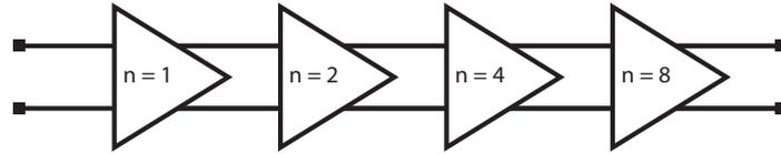
(a) Cascade of CML buffers used for circuit simulation
