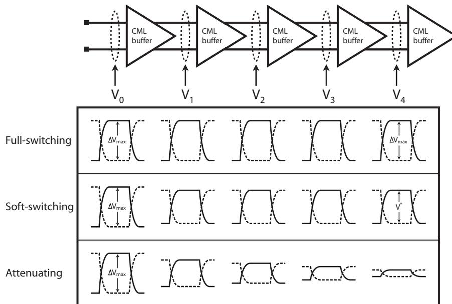
Figure 3.5: The three regions of operation for CML circuits
