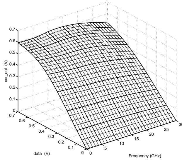
Figure 3.15: VTC of XOR circuit with data as input and clock signal fully-switched
