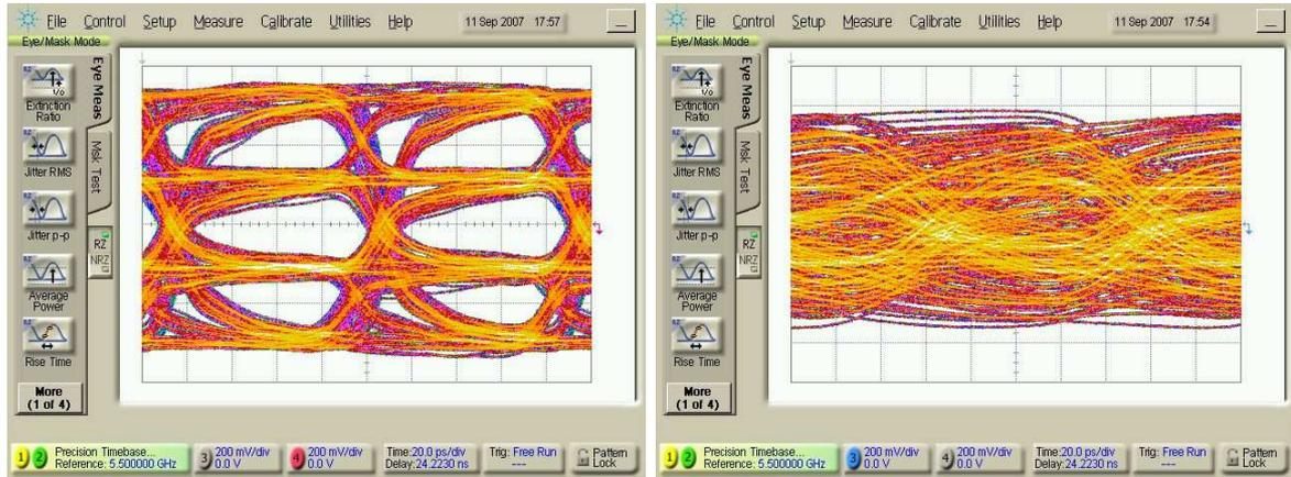
(a) Eye diagram at output of transmitter
