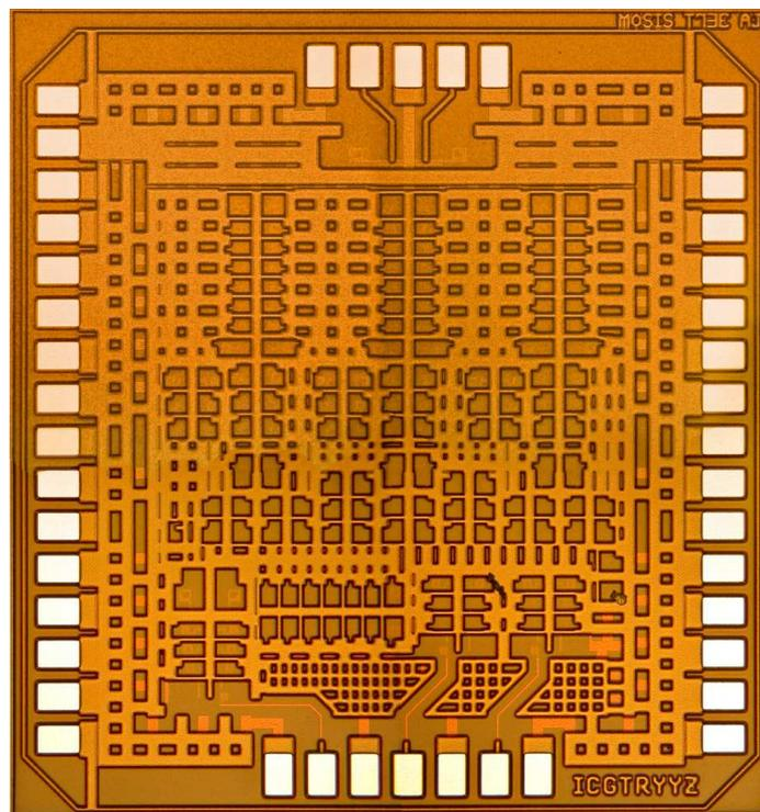
Figure 5.1: Die photo of transmitter
