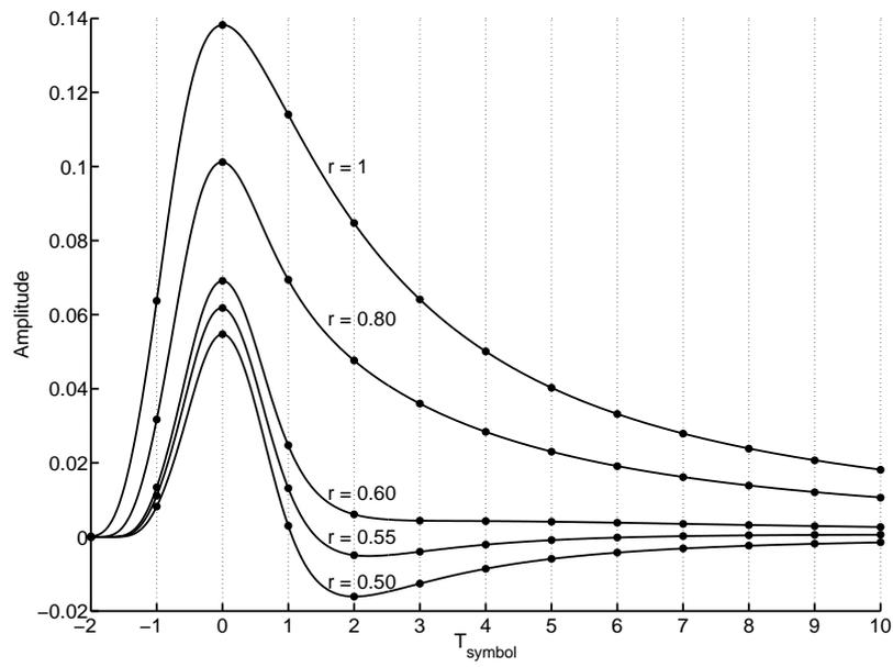
(a) Pulse response of FIR pre-emphasis at  $T_{symbol} = 50ps$
