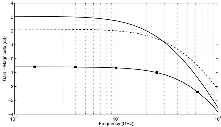
Figure 3.9: AC gain response for design I(solid), II(square marker), IV(dashed)
