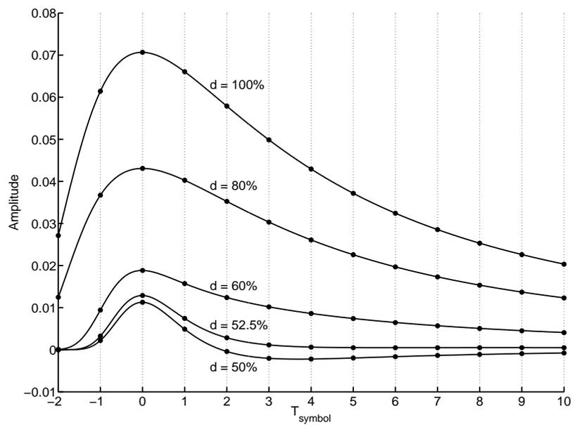
(b) Pulse response of PWM pre-emphasis at  $T_{symbol} = 25ps$ Figure 2.4: Pulse response after 40m of Belden 1694A coaxial cable at  $T_{symbol} = 25ps$
