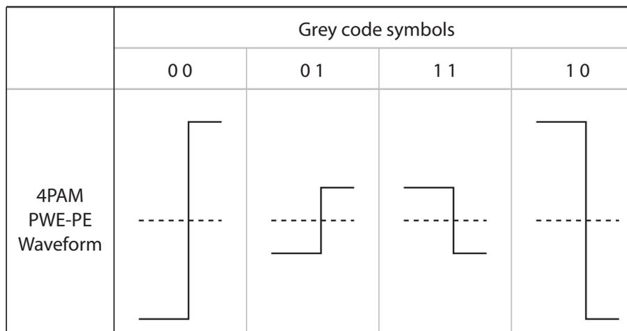
Figure 2.7: Output waveform of 4PAM transmitter with PWM-PE
