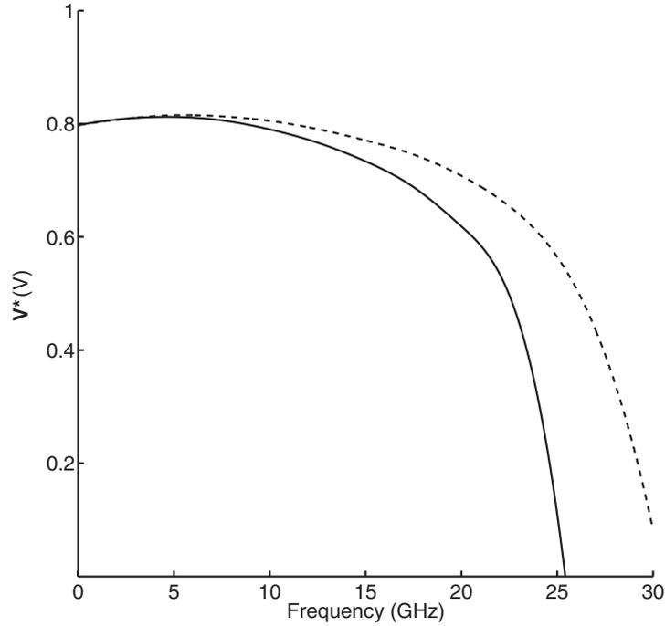
Figure 3.13:  $V^*$  as a function of frequency;  $k = 1.5$ (solid);  $k = 1.2$ (dashed)
