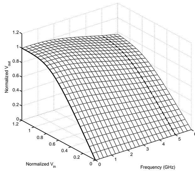
(b) Design III:  $W = 27\mu m$ ,  $\Delta V_{MAX} = 635mV$
