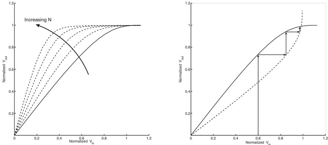
(a) VTCs of a cascade of full-switching CML buffers; solid line - one stage VTC; dash line - cascaded stage 2 to 5
