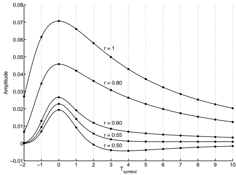
(a) Pulse response of FIR pre-emphasis at  $T_{symbol} = 25ps$
