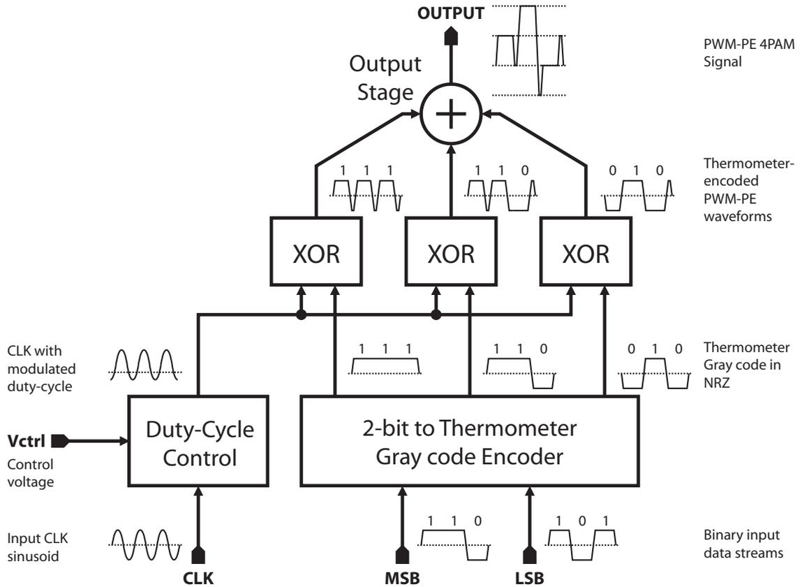
Figure 4.1: Functional block diagram of transmitter system architecture
