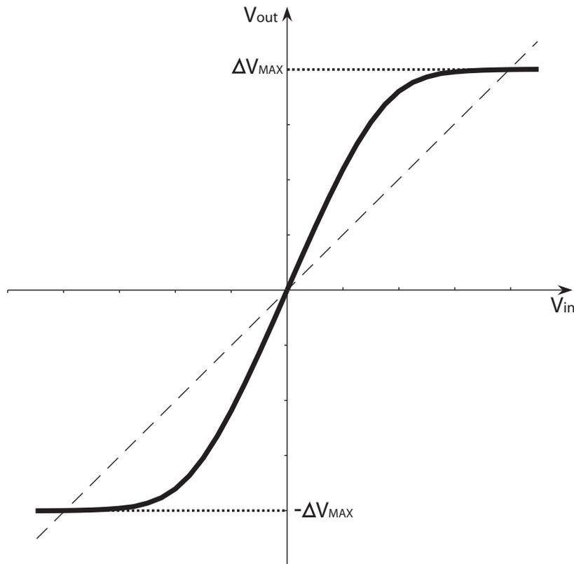
Figure 2.10: VTC of a CML circuit operating in full-switching region
