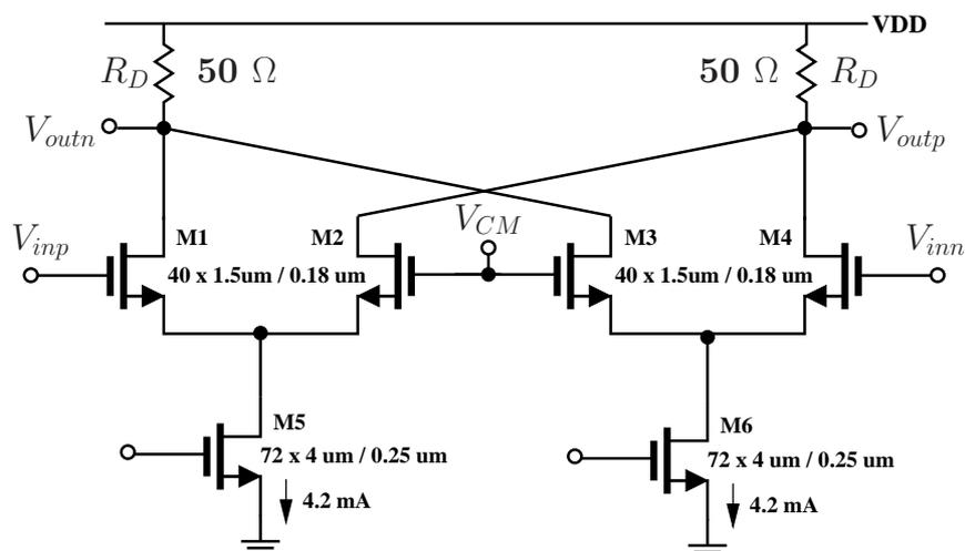
Figure 3.18: Output buffer: Schematic.
