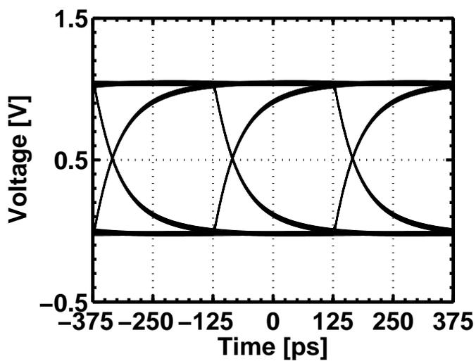
Figure 2.7: Behavioral simulation eye diagram of the equalized SML detector at 4 Gbps.
