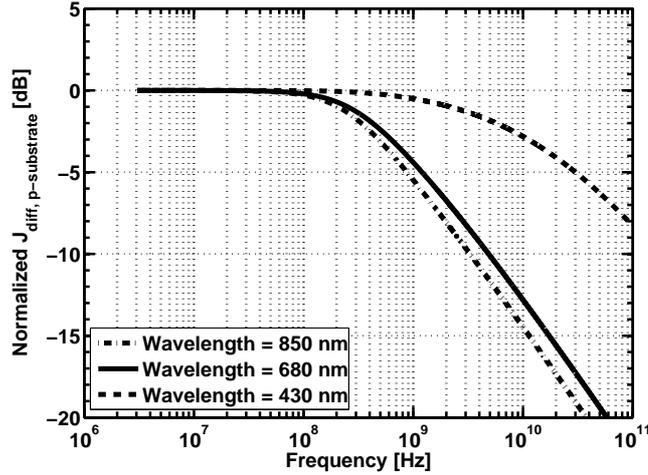
Figure 2.2: Normalized  $J_{diff, p-substrate}$  for different wavelengths.
