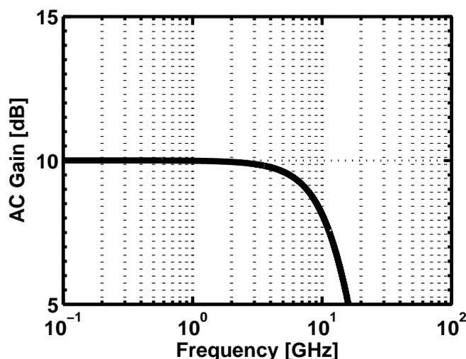
Figure 3.9: Subtractor: Frequency response.
