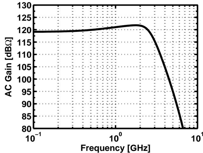
Figure 3.20: Complete optical receiver: Frequency response.
