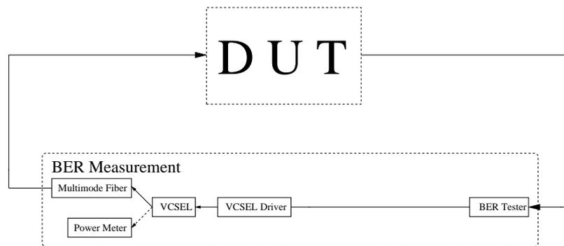
Figure 4.9: BER measurement setup.
