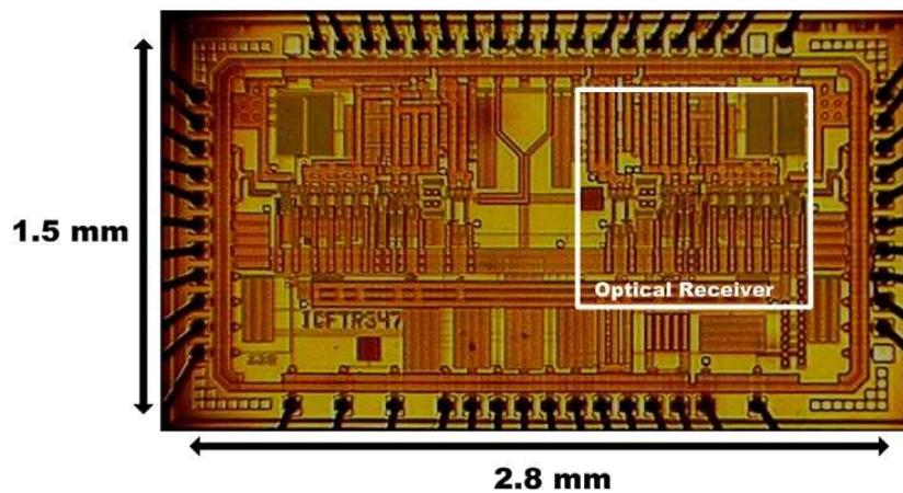
Figure 4.1: Die photo of the chip with the optical receiver highlighted.
