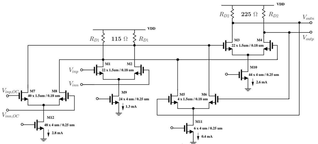
Figure 3.16: LA: Input stage schematic.
