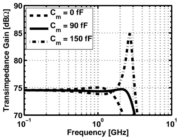
Figure 3.4: TIA: Frequency response with different values of  $C_m$ .
