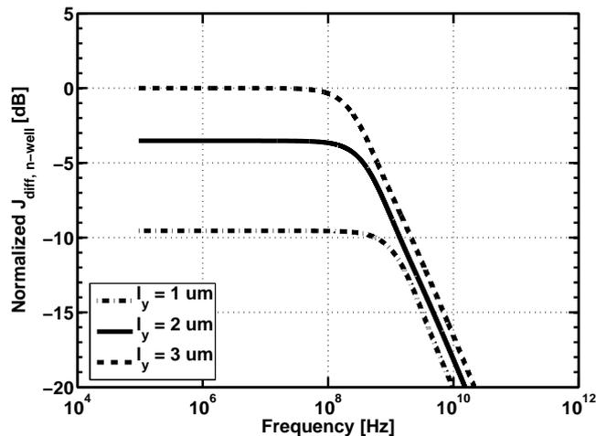
Figure 2.3: Normalized  $J_{diff, n-well}$  for different  $l_y$ .
