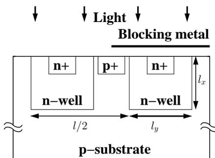
Figure 2.1: Simplified cross section of the SML detector.
