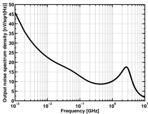
Figure 3.5: TIA: Output noise spectrum density.
