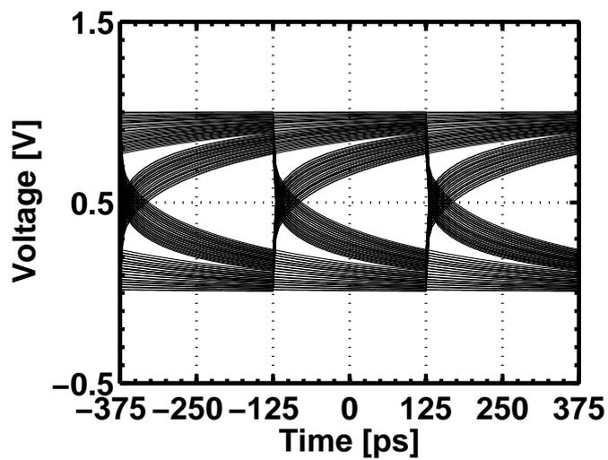
Figure 2.5: Behavioral simulation eye diagram of the SML detector at 4 Gbps.
