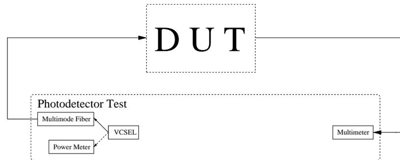
Figure 4.6: Photodetector responsivity test setup.
