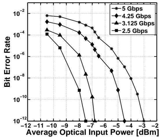
Figure 4.14: Measured BER as a function of average optical input power at different data rates under high speed setting.
