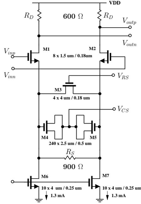
Figure 3.11: Equalizer: Schematic.
