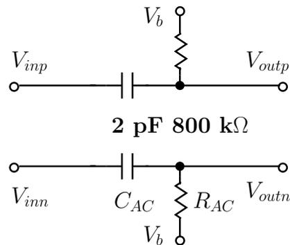
Figure 3.8: AC coupling: Schematic.
