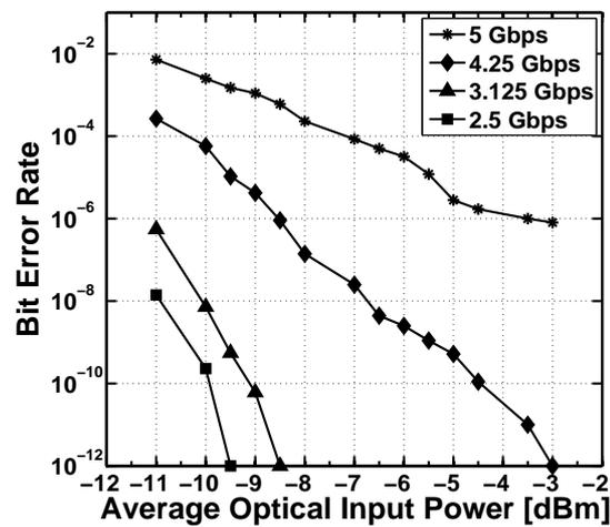
Figure 4.12: Measured BER as a function of average optical input power at different data rates under low power setting.
