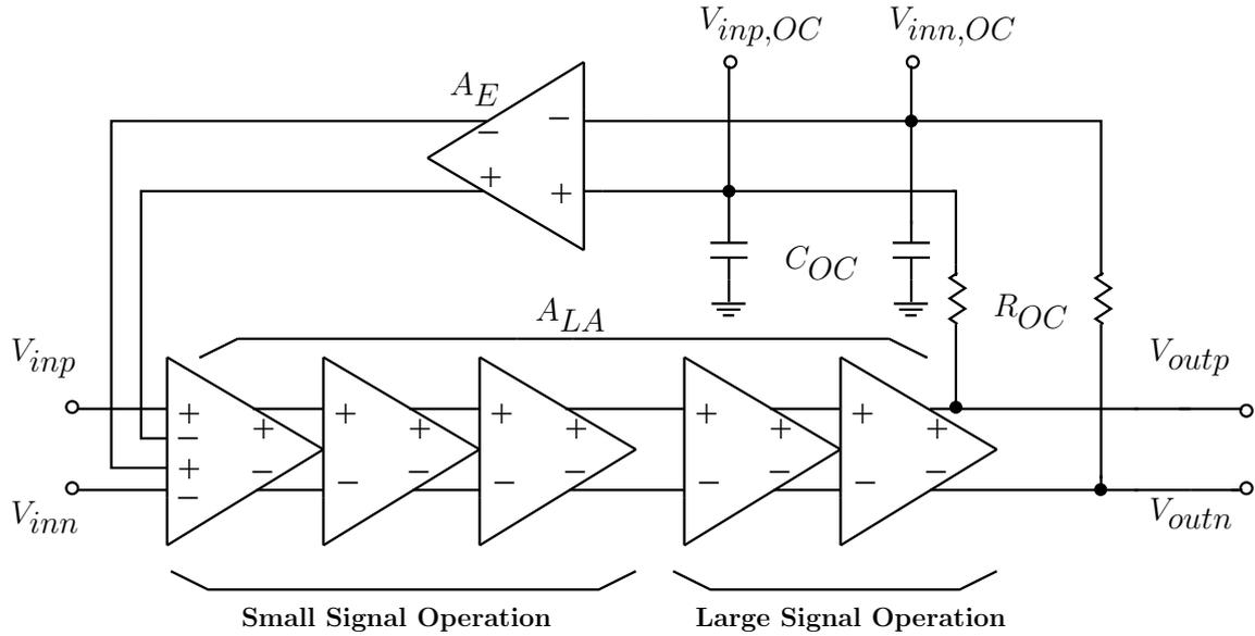
Figure 3.14: LA: Block diagram.
