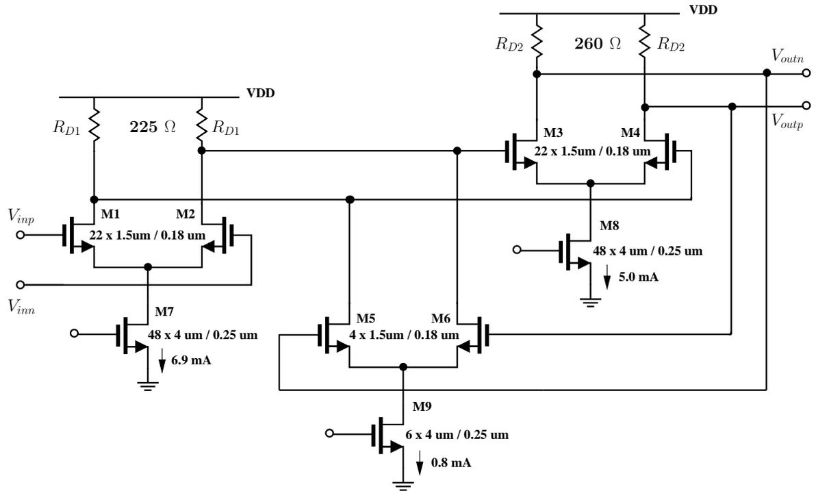
Figure 3.7: Subtractor: Schematic.
