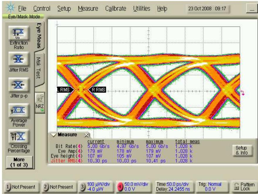
Figure 4.5: Measured eye diagram at 5 Gbps using  $2^{31} - 1$  PRBS pattern with an input swing of  $8 \text{ mV}_{pp}$ .
