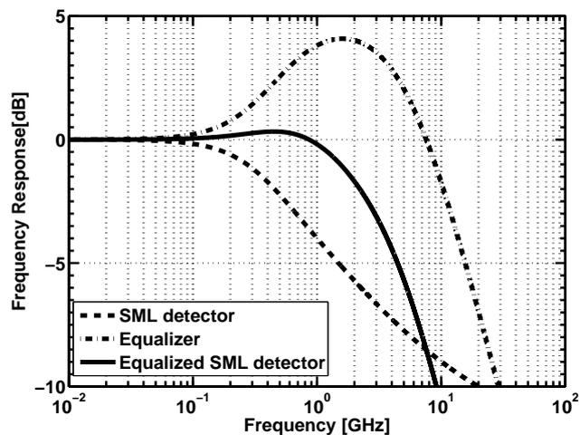
Figure 2.6: Frequency response of the SML detector, the equalizer, and the equalized SML detector.
