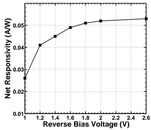
Figure 4.7: Net responsivity of the photodetector at different reverse bias voltages.
