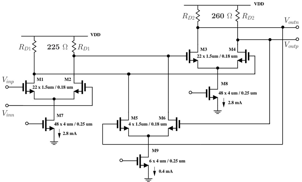
Figure 3.15: LA: Gain cell schematic.
