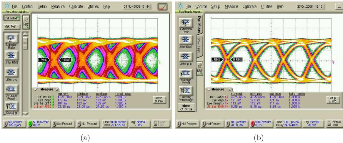
Figure 4.11: Measured eye diagrams for at 4.25 Gbps for a  $2^{31} - 1$  PRBS pattern with an average optical input power of -3 dBm with (a) equalization off and with (b) equalization on.
