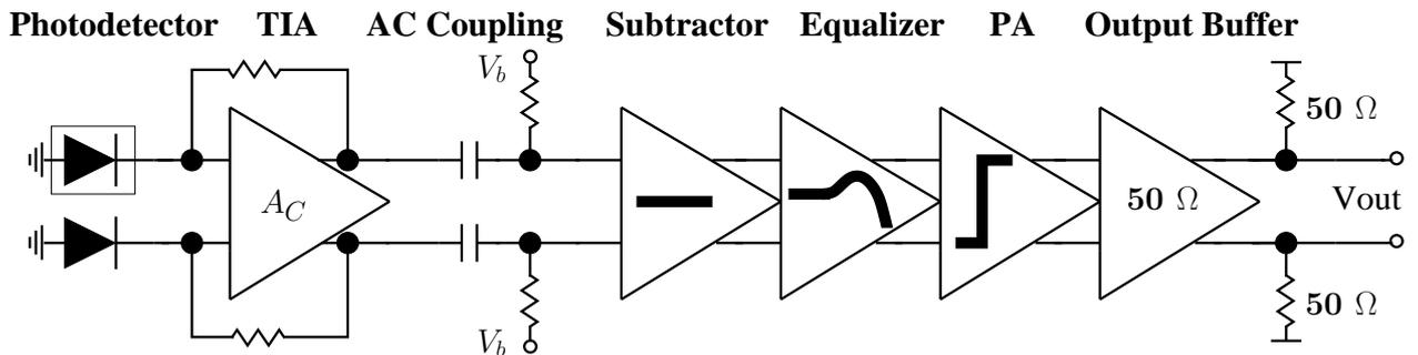
Figure 3.1: Optical receiver block diagram.
