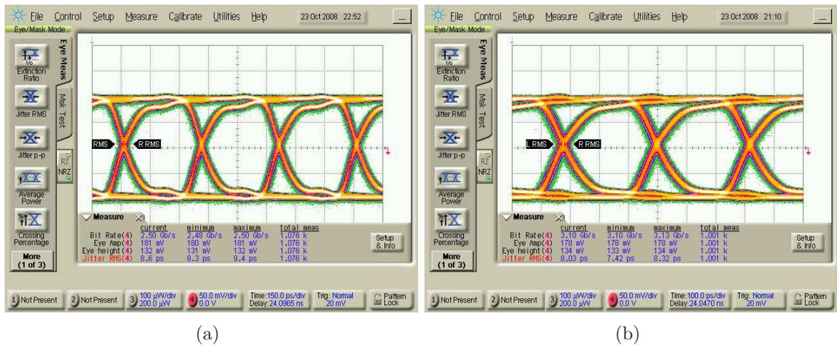
Figure 4.10: Measured eye diagrams for a  $2^{31} - 1$  PRBS pattern with an average optical input power of -3 dBm at (a) 2.5 Gbps and (b) 3.125 Gbps.
