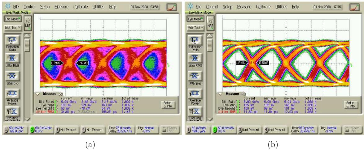
Figure 4.13: Measured eye diagrams for at 5 Gbps for a  $2^{31} - 1$  PRBS pattern with an average optical input power of -3 dBm with (a) equalization off and with (b) equalization on.
