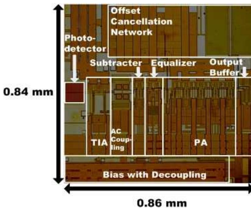
Figure 4.2: Die photo of the optical receiver.
