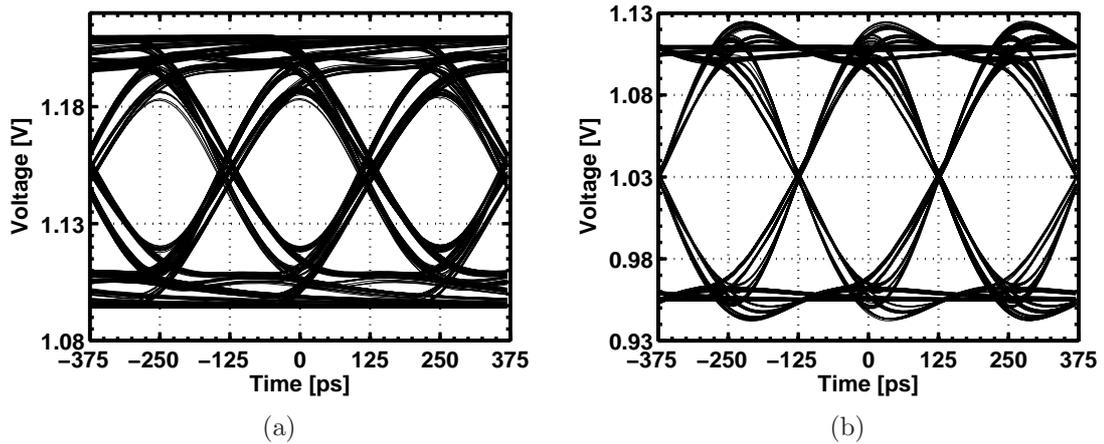
Figure 3.13: Equalizer: Eye diagram at 4 Gbps (a) before and (b) after the equalizer with  $V_{CS} = 1.2$  V and  $V_{RS} = 0.8$  V.
