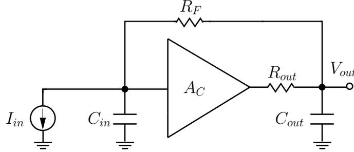
Figure 3.2: Shunt-shunt feedback TIA.
