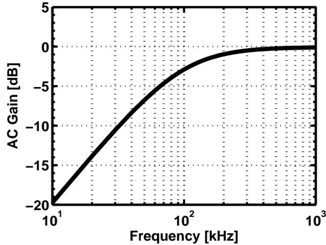
Figure 3.10: AC coupling: Frequency response.
