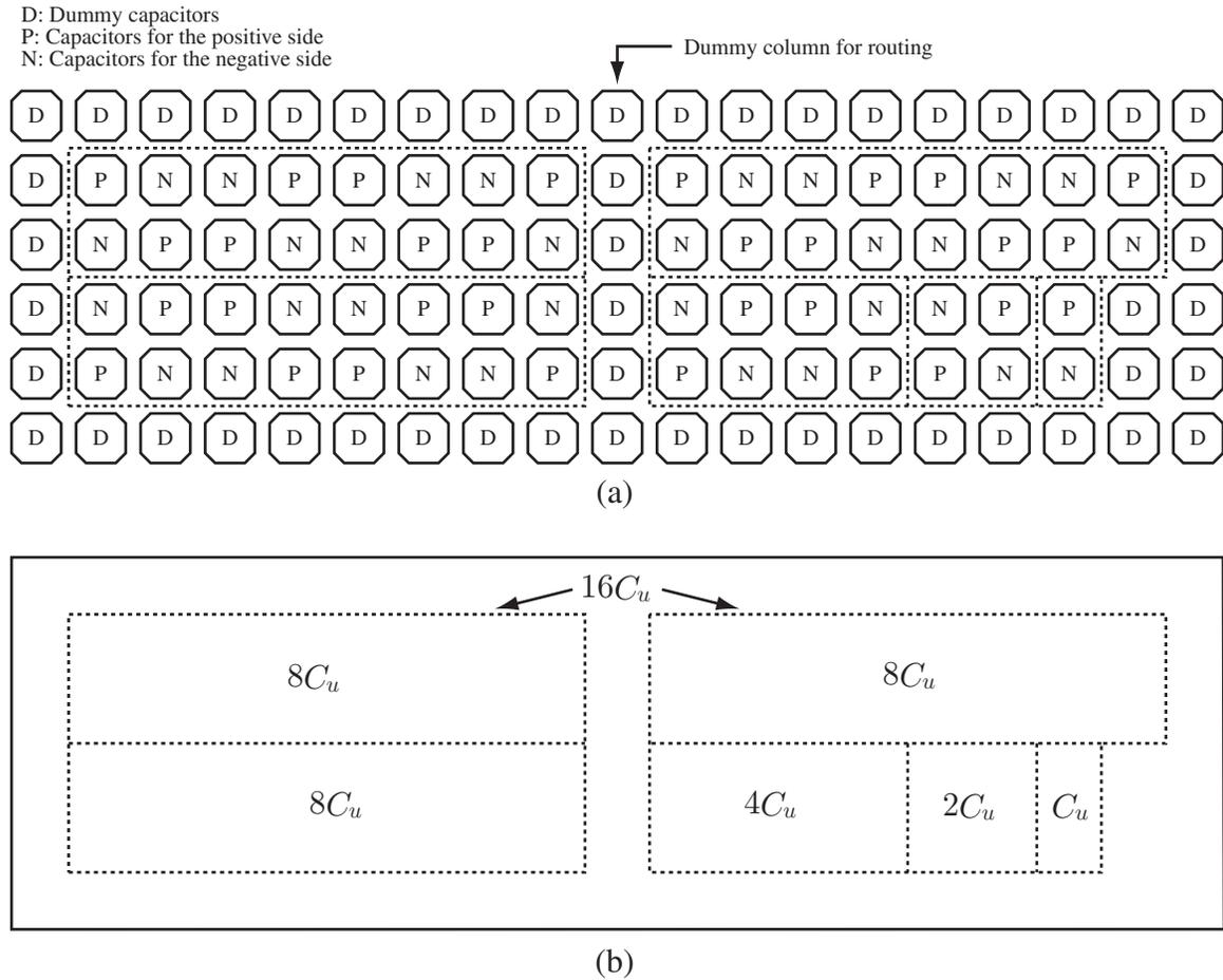
Figure 4.27: (a) 5-bit Binary-weighted capacitor array (b) Capacitor array floorplan.
