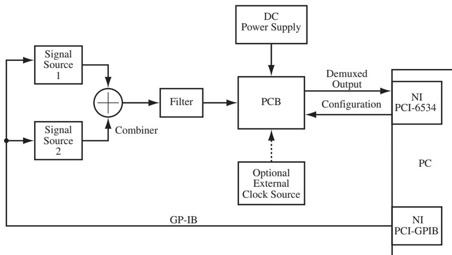
Figure 5.3: Planned test setup.
