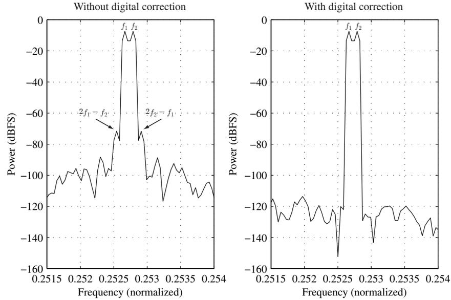
Figure 3.15: Modulator output spectra without and with digital correction.
