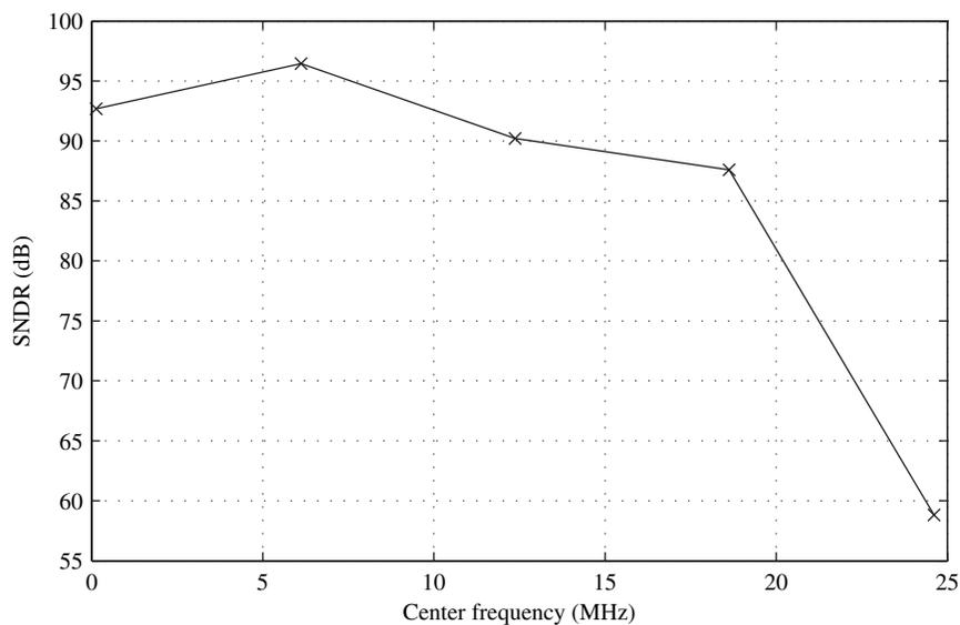
Figure 4.23: SNDR obtained from circuit simulations.
