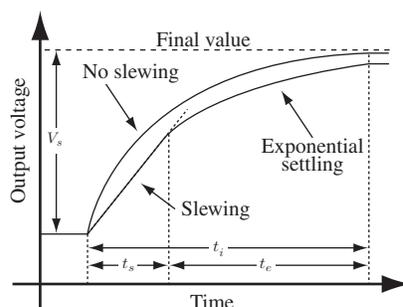
Figure 3.19: Effects of slewing and a non-zero time constant.
