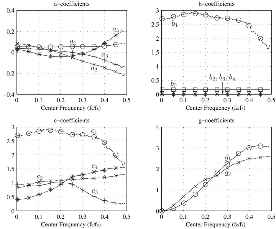
Figure 3.6: Modulator coefficients after dynamic range scaling.
