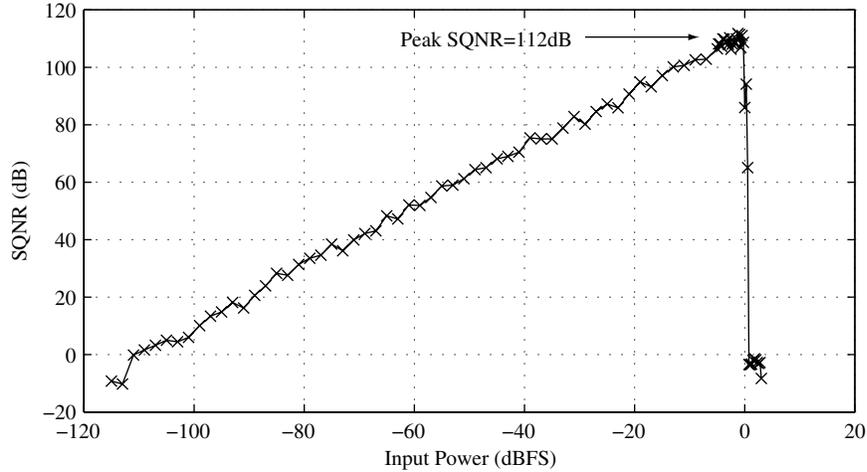
Figure 3.1: SQNR versus input level of the second-order modulator with a 4-bit quantizer.
