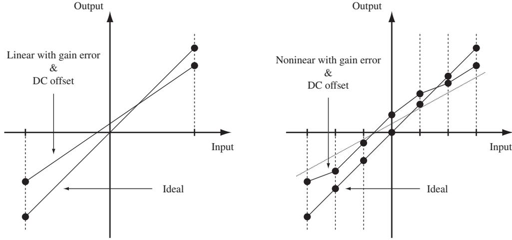
Figure 2.12: Comparison of non-ideal single-bit and multi-bit DACs.
