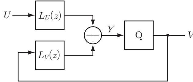
Figure 2.10: General model of a delta-sigma modulator.
