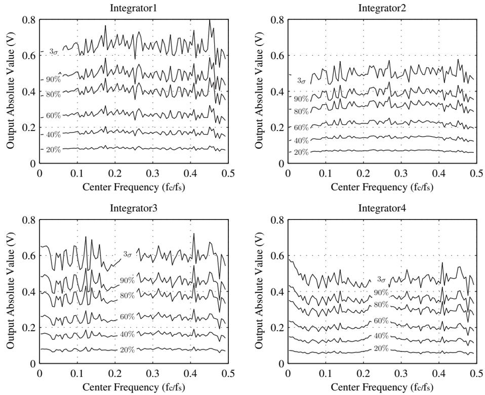
Figure 3.12: Integrator output after coefficient quantization.
