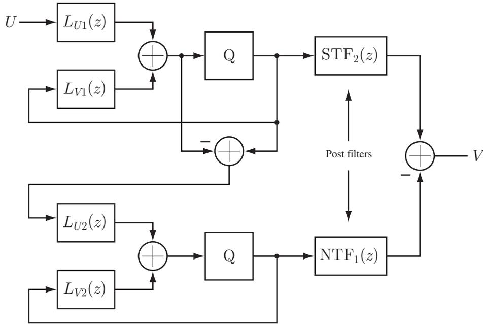
Figure 2.11: Cascaded-modulator structure.
