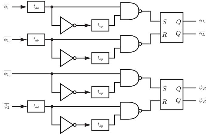
Figure 4.18: Clock generator for ADC.
