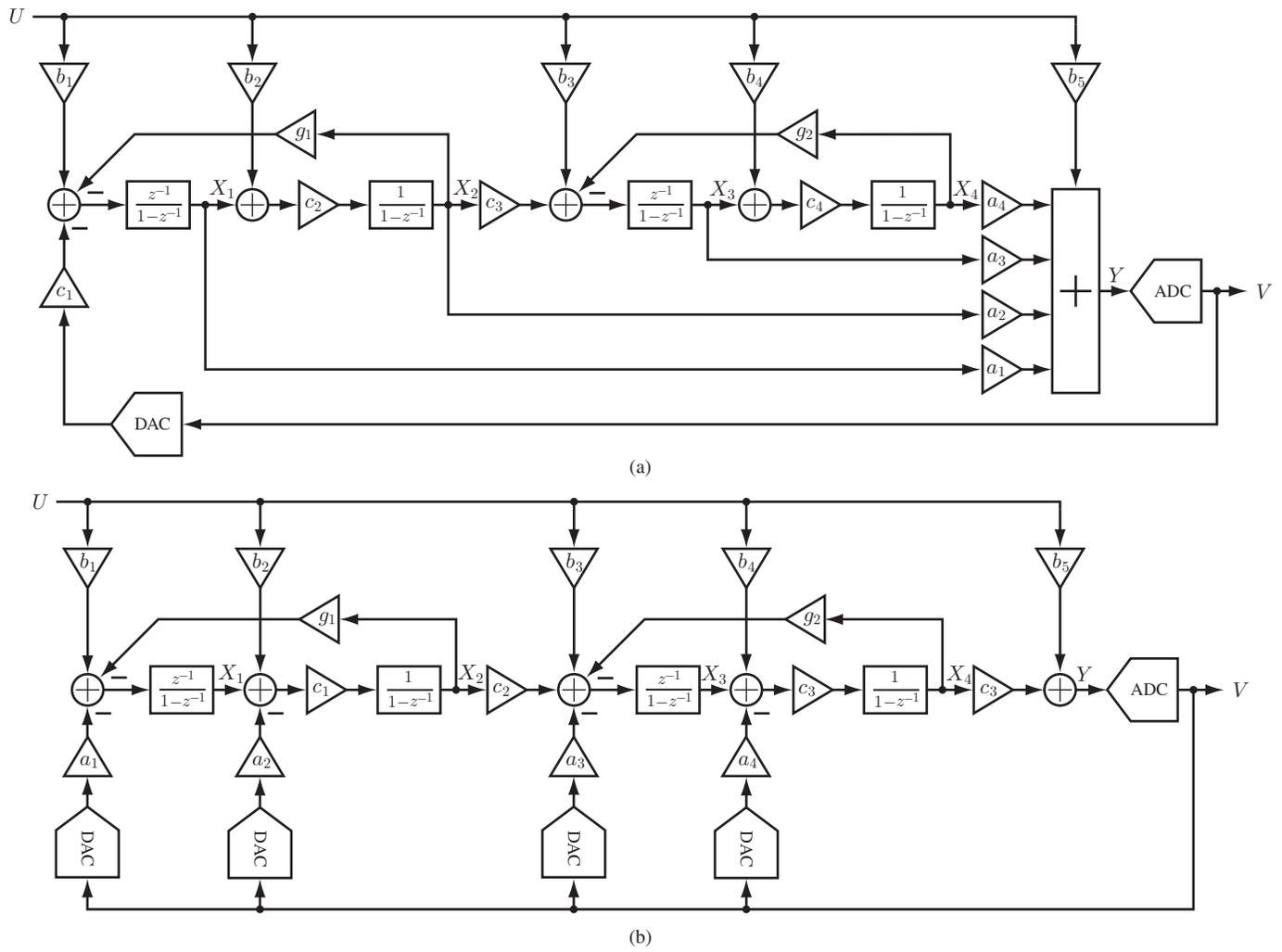
Figure 3.2: (a)Fourth-order CRFF Structure (b)Fourth-order CRFB structure.
