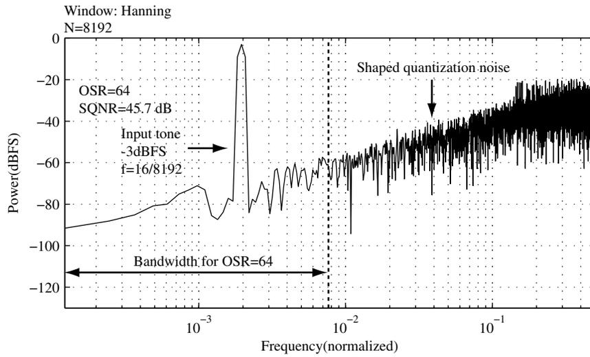
Figure 2.6: Output spectrum of the first-order delta-sigma modulator with a single-sinusoid input.
