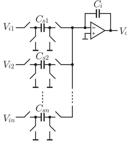
Figure 3.21: An integrator with multiple input SC branches.
