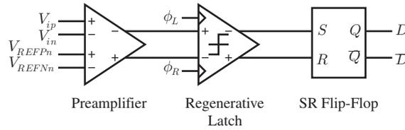
Figure 4.11: Block diagram of the comparator.
