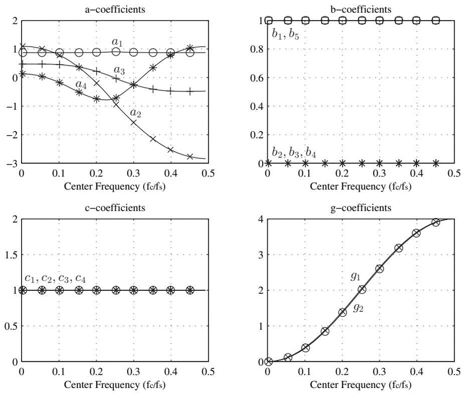
Figure 3.4: Modulator coefficients before dynamic range scaling.
