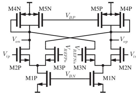
Figure 4.12: Preamplifier of the comparator.
