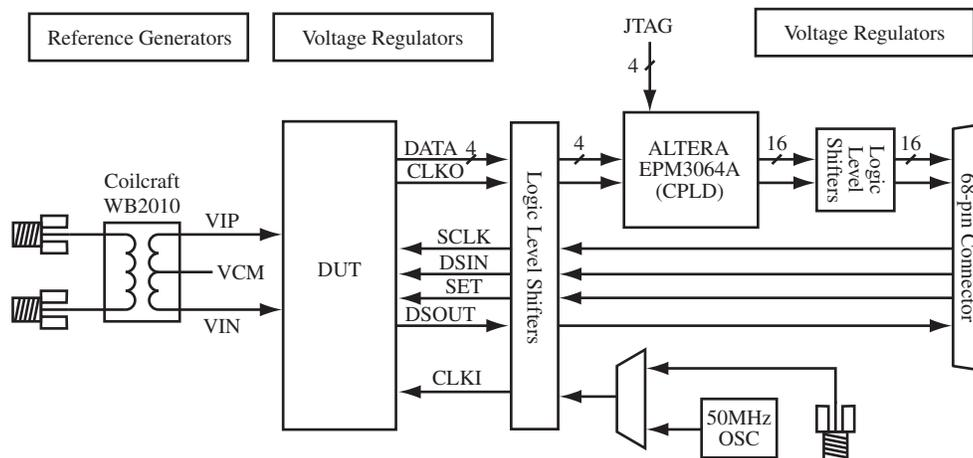
Figure 5.2: PCB block diagram.
