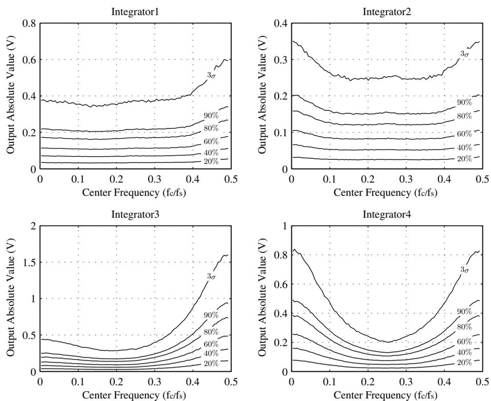
Figure 3.5: Integrator output swing for different center frequencies before dynamic range scaling.
