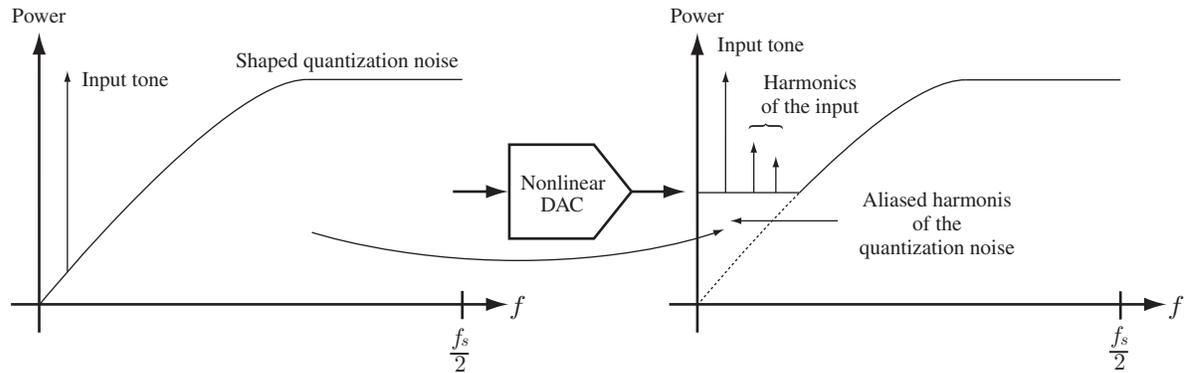
Figure 2.14: The effect of a nonlinear DAC.
