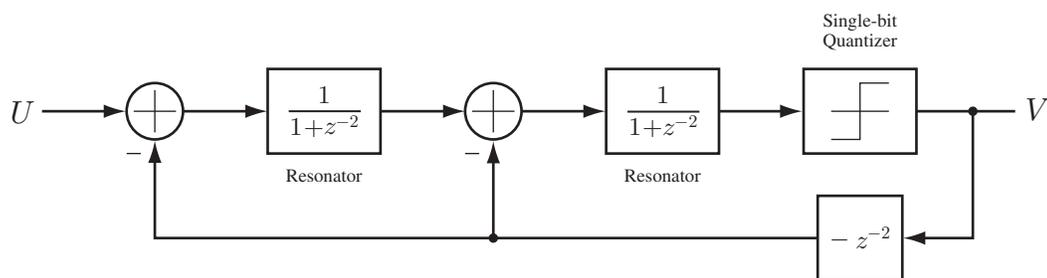
Figure 2.18: Fourth-order Bandpass Delta-Sigma Modulator.
