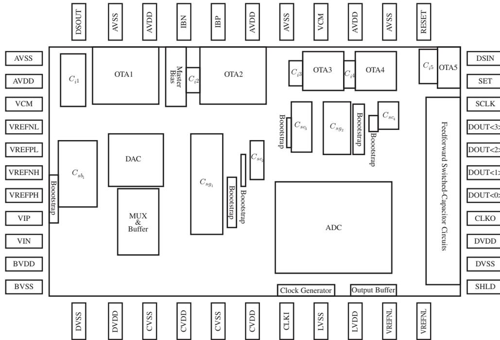
Figure 4.25: Modulator floor plan.
