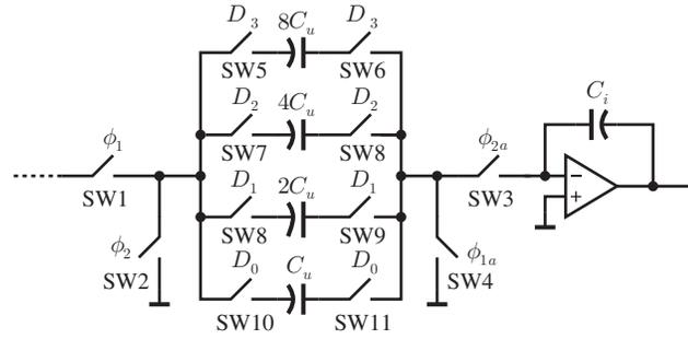
Figure 4.7: A possible implementation of a switched-capacitor integrator [1].
