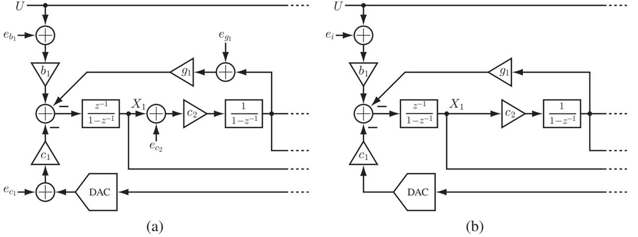
Figure 3.17: Noise sources of the first resonator and its input-referred thermal noise equivalent.
