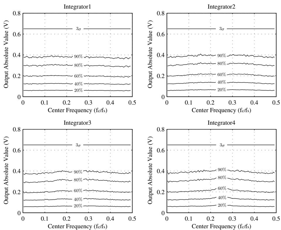
Figure 3.7: Integrator output after dynamic range scaling.
