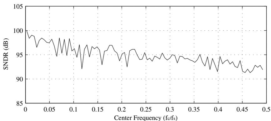
Figure 3.18: SNDR from a simulation with coefficient quantization and thermal noise sources.
