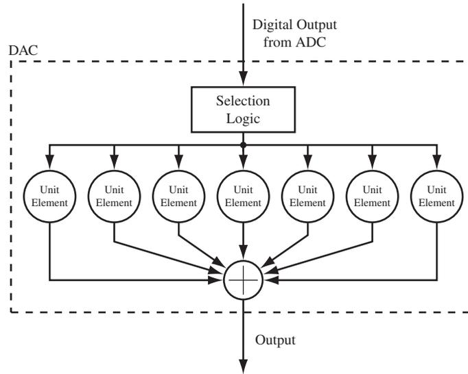
Figure 2.15: An 8-level DAC with unit elements.
