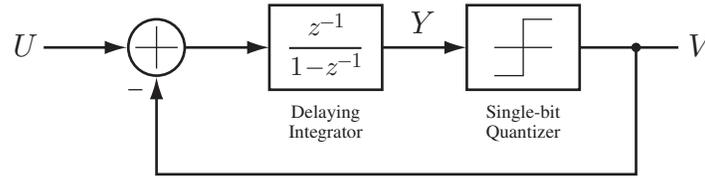
Figure 2.2: Equivalent model with a quantizer.
