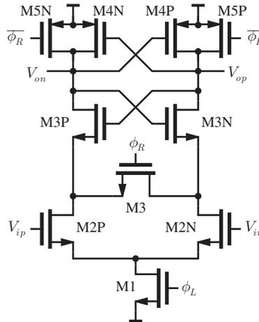
Figure 4.13: Latch of the comparator.
