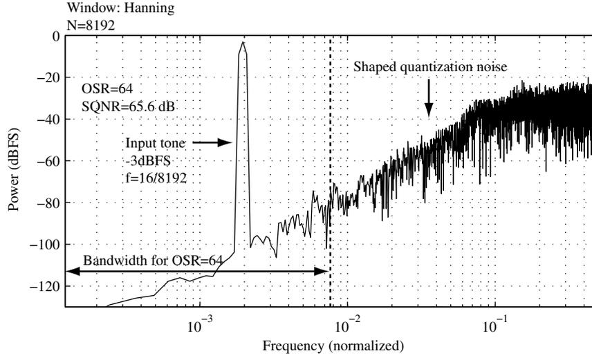
Figure 2.9: Output spectrum of the second-order delta-sigma modulator with a single-sinusoid input.
