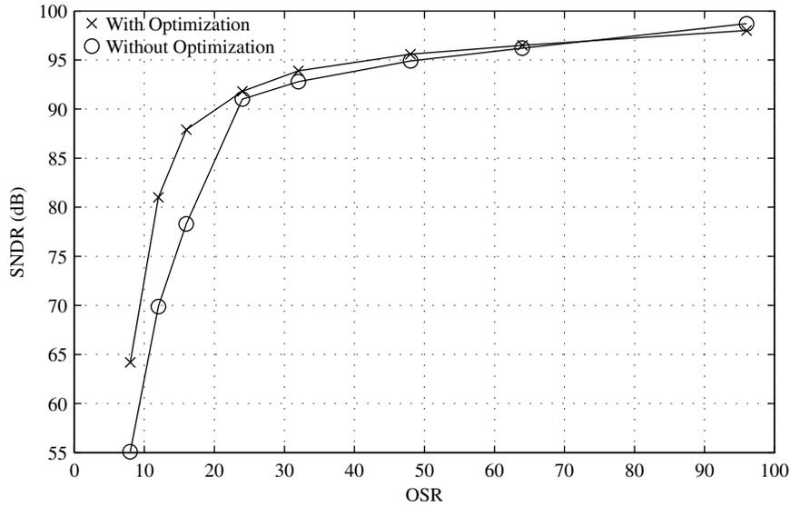
Figure 3.23: SNDR obtained with and without NTF zero optimization for the lowpass configuration.
