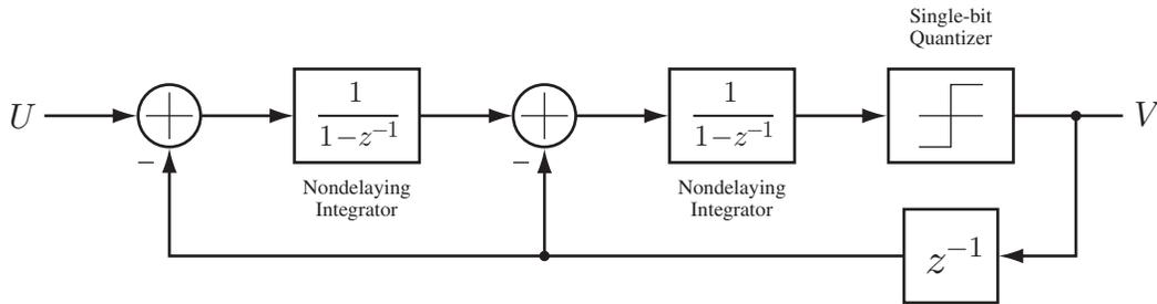
Figure 2.7: Second-order delta-sigma modulator.
