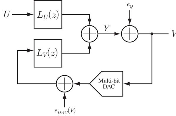
Figure 2.13: Multi-bit delta-sigma modulator with a nonlinear DAC.
