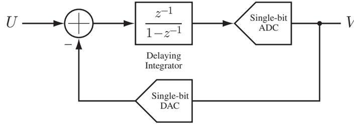
Figure 2.1: First-order delta-sigma modulator.
