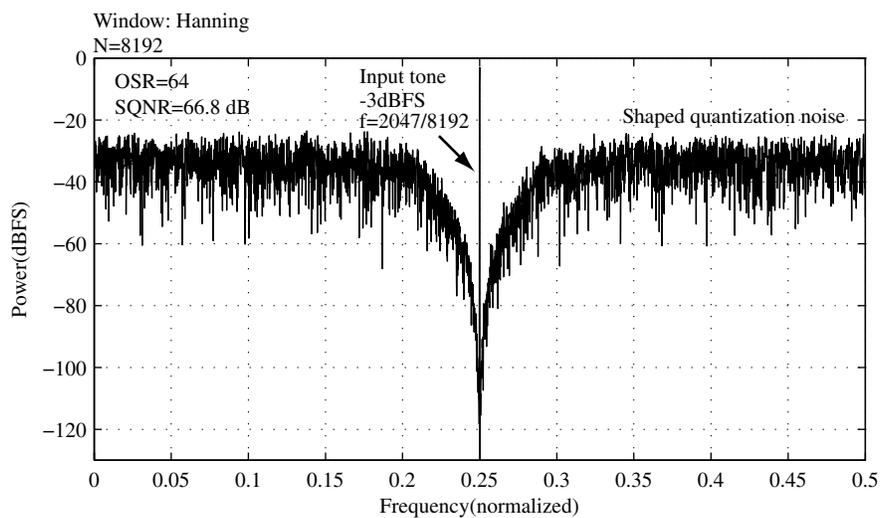
Figure 2.19: Output spectrum of the fourth-order delta-sigma modulator.
