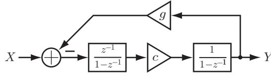
Figure 3.9: Discrete-time resonator.
