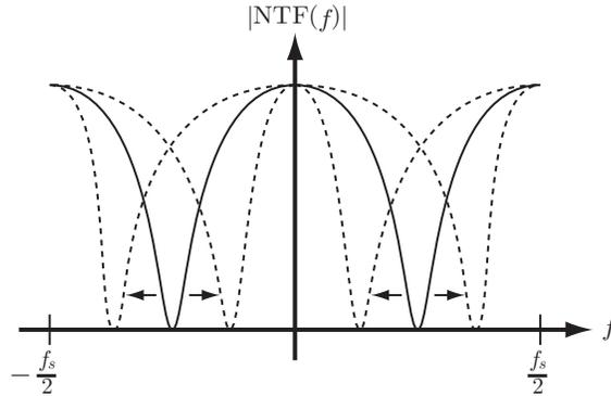
Figure 2.20: NTF of a Tunable Bandpass Delta-Sigma Modulator.
