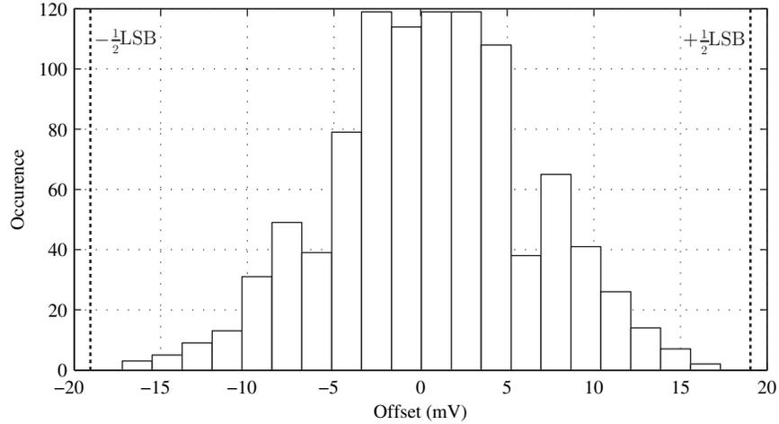
Figure 4.14: Histogram of the comparator input offset voltage for 1000 Monte-Carlo simulation runs.
