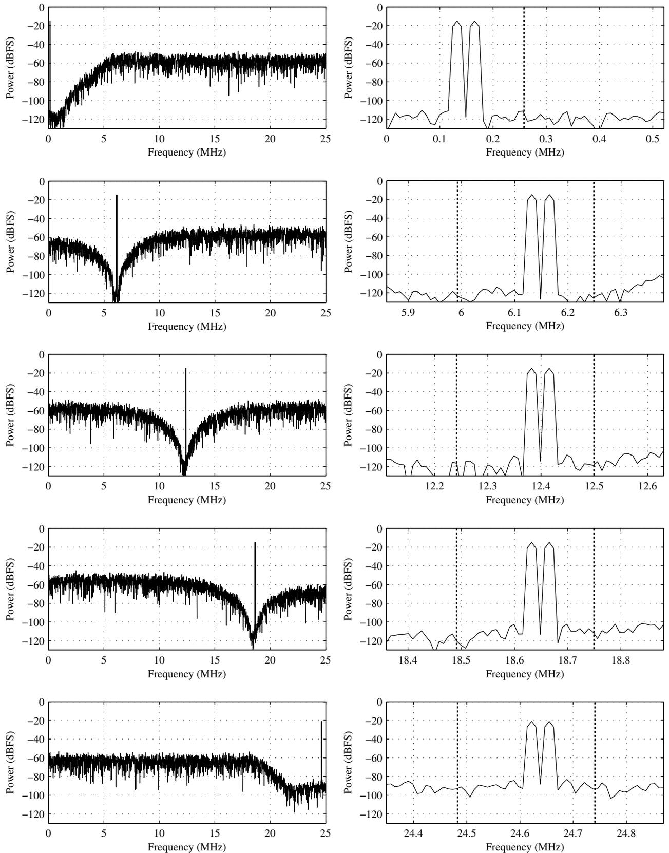
Figure 4.22: Modulator output spectra obtained from circuit simulations (6144-point DFT with Hann windowing).
