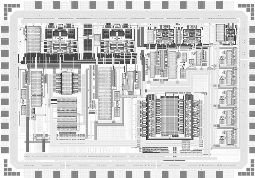
Figure 4.26: Modulator layout.
