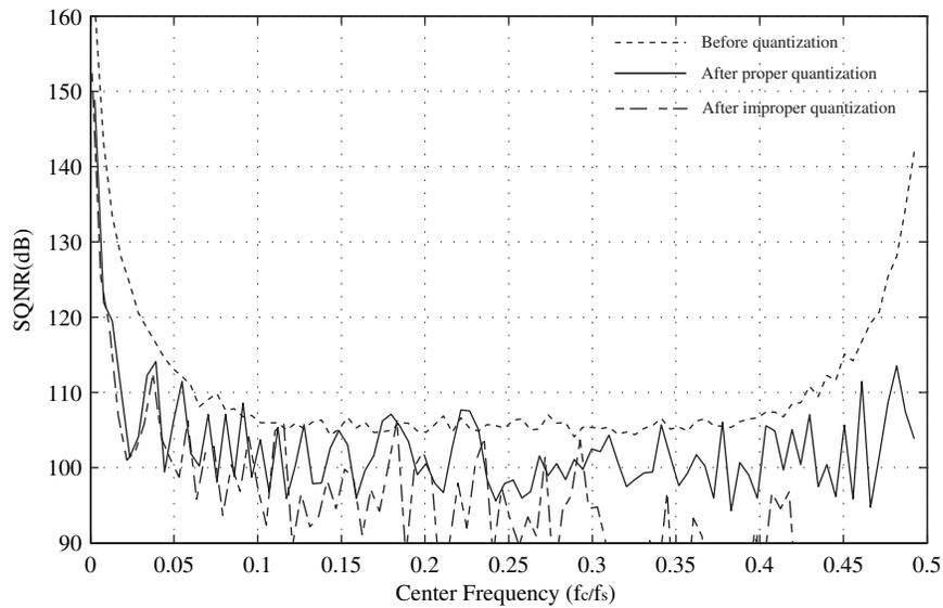
Figure 3.13: SQNR after modulator coefficient quantization.
