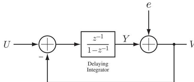
Figure 2.3: Linearized model of first-order delta-sigma modulator.
