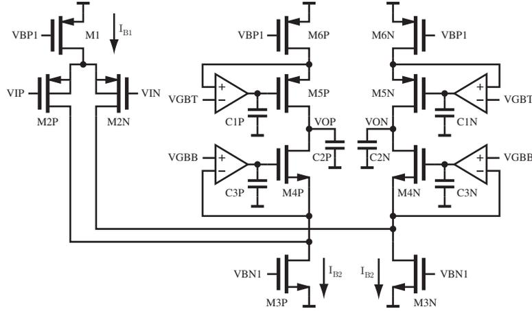
Figure 4.3: Schematic of the OTA.
