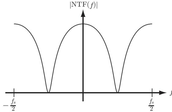
Figure 2.17: NTF of a bandpass delta-sigma modulator.
