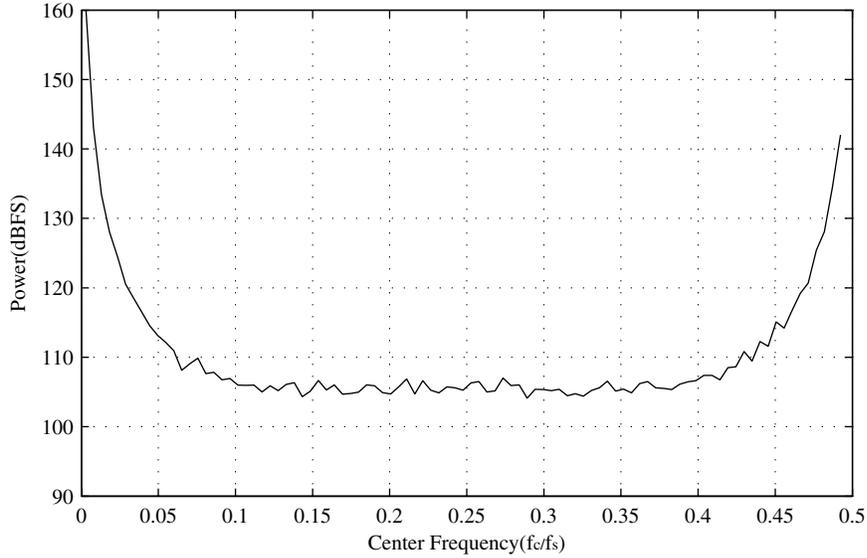
Figure 3.3: SQNR for different center frequencies for the tunable modulator at an OSR of 96 with two-tone input.
