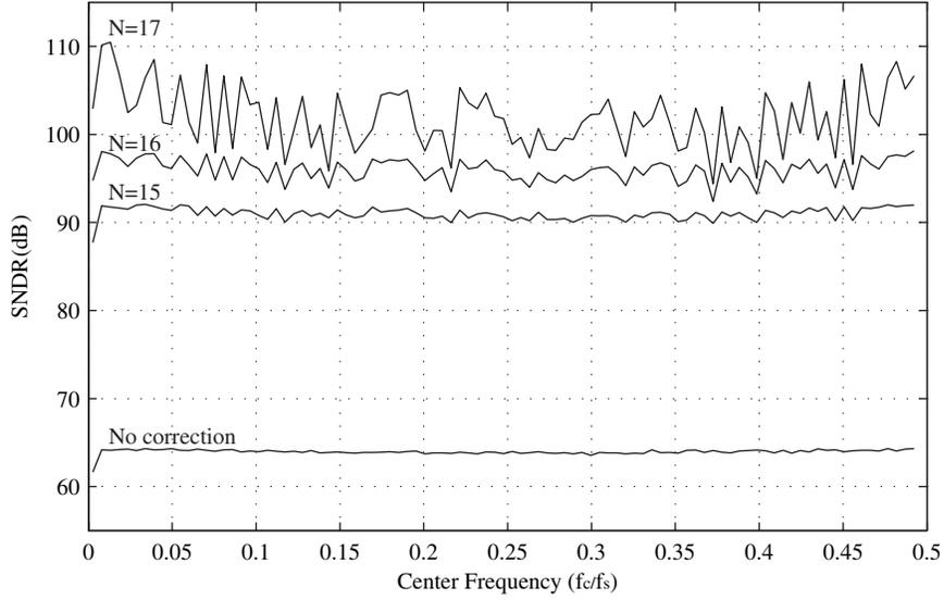
Figure 3.16: Comparison of SNDR without/with digital correction.
