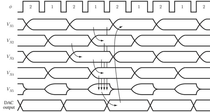
Figure 4.2: Timing Diagram of the Modulator.
