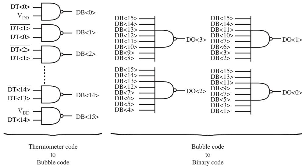
Figure 4.21: Thermometer to binary converter.
