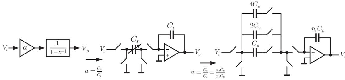
Figure 3.8: Conceptual implementation of a programmable coefficient.
