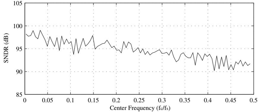
Figure 3.22: SNDR with thermal noise and circuit non-idealities.
