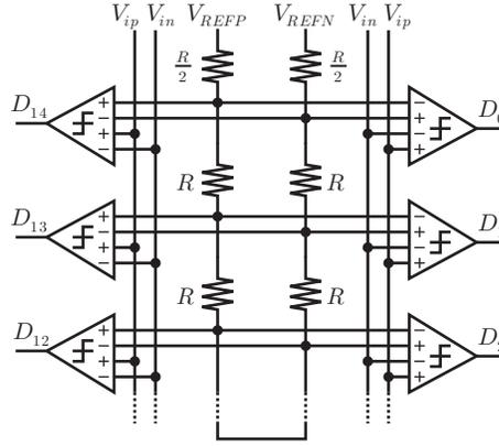
Figure 4.10: Flash ADC (clock signals omitted).
