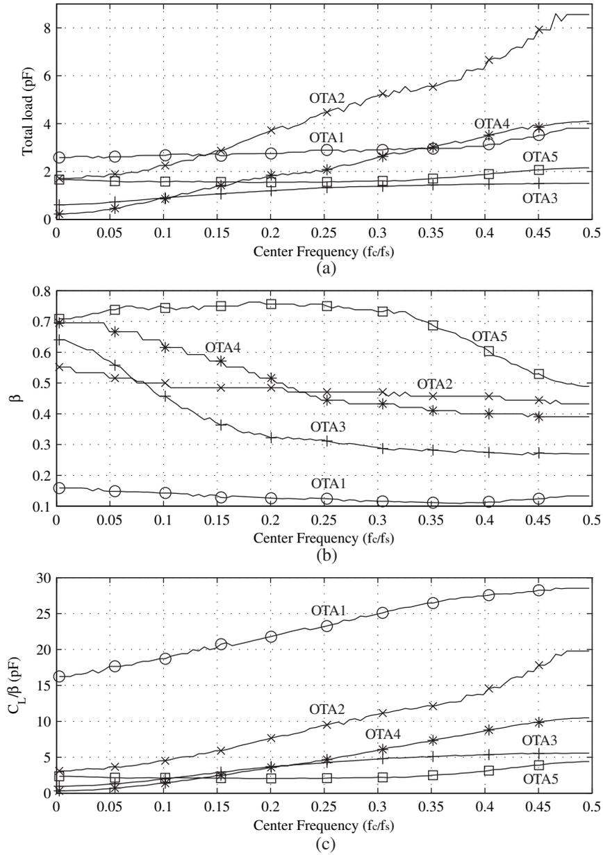
Figure 3.20: (a) Load capacitances ( $C_L$ ), (b) feedback coefficients of OTAs ( $\beta$ ), and (c)  $\frac{C_L}{\beta}$ .
