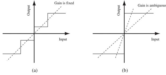
Figure 2.4: Transfer curves of (a) multi-bit quantizer and (b) single-bit quantizer.
