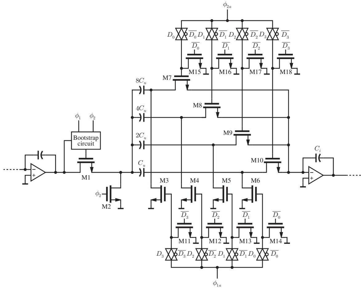
Figure 4.8: A more suitable programmable switched-capacitor integrator.
