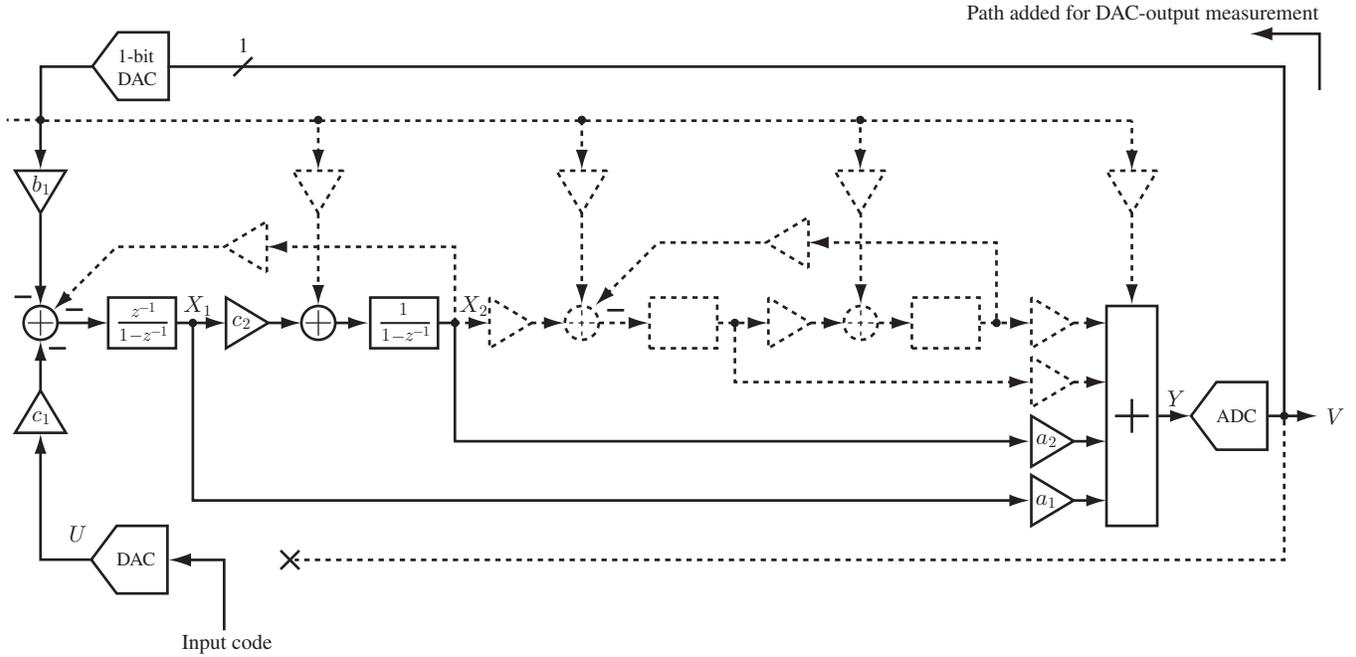
Figure 3.14: Modulator configuration to measure the DAC nonlinearity for digital correction.
