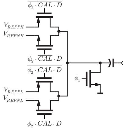
Figure 4.16: Schematic of a unit DAC.
