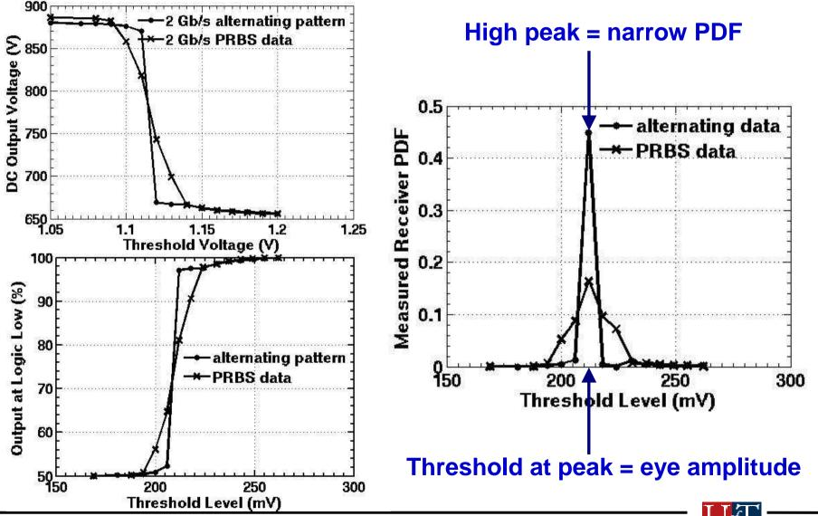
Gain and Equalization Adaptation to Optimize the Vertical Eye Opening in a Wireline RX
