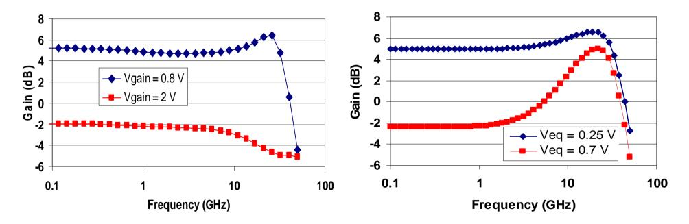
Gain and Equalization Adaptation to Optimize the Vertical Eye Opening in a Wireline RX
