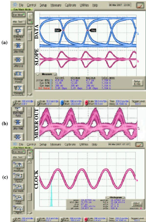
Fig. 11. Waveforms at different points of the TR loop. (a) Data (top eye) and slope (bottom eye) outputs of passive filter at 2-Gb/s. (Vertical scale (top eye)=100mV/div; Vertical scale (bottom eye)=50mV/div; Horizontal scale=200ps/div) (b) Mixer output corresponding to a 2-Gb/s random data sequence (Vertical scale= 50mV/div; Horizontal scale=200ps/div). (c) Recovered 2-GHz clock (Vertical scale= 100mV/div; Horizontal scale=200ps/div).
