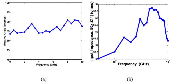
Fig. 8. Network analyzer measurements. (a) Relative angle between the data and slope paths. (b) Input impedance of the passive filter.
