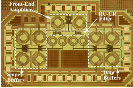
Fig. 6. Die Photo of Passive Filter
