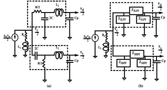
Fig. 3. Small signal model of passive filter. (a) Small signal half-circuit. (b) Small signal half-circuit with RCL-CRL sections replaced by equivalent  $\Delta$  sections.
