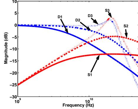
Fig. 4. Data and slope path frequency responses. D1 and S1 respectively denote the data and slope path transfer functions without inductors  $L_1, L_2$ ; D2 and S2 respectively denote the data and slope path transfer functions with inductor  $L_1$  only and D3 and S3 respectively denote the data and slope path transfer functions without both inductors  $L_1, L_2$ . For these simulations,  $g_m = 20\text{mA/V}$ ,  $C_p = 110\text{fF}$  and all other parameters were taken from the table in Fig. 2.
