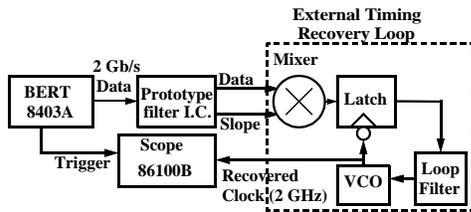
Fig. 10. Test set up for external TR loop using the passive filter.
