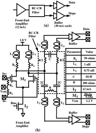
Fig. 2. Passive Filter. (a) Block diagram. (b) Schematic.
