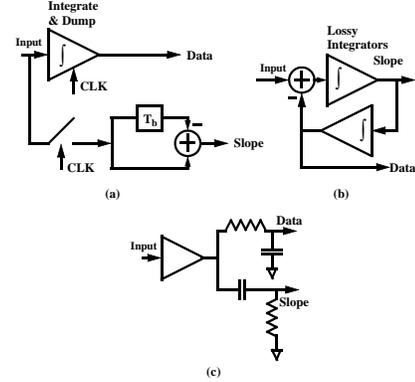
Fig. 1. Slope detection techniques. (a) Integrate and Dump [7]. (b) Active Filter [5]. (c) Passive filter comprised of RC-CR section [This work].
