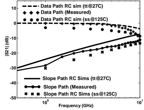
Fig. 7. Measured and simulated  $S_{21}$  in the data and slope paths.
