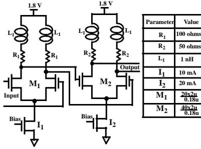
Fig. 5. Schematic of two-stage buffer.
