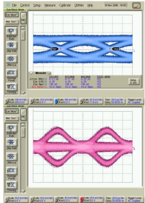
Fig. 9. Data (top eye) and slope (bottom eye) outputs of passive filter at 10-Gb/s (Vertical scale (top eye)=100mV/div; Vertical scale (bottom eye)=25mV/div; Horizontal scale=20ps/div).
