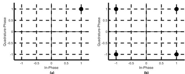
Fig. 11: Constellation diagram of the received QPSK signal (a) in the presence of the CW blocker (b) after the blocker is cancelled.
