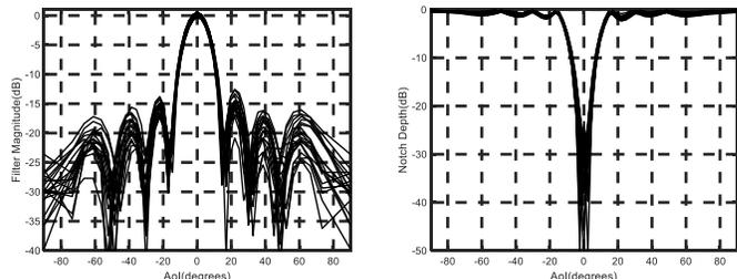
Fig. 8: Blocker extraction and notch filter for 5 percent mismatch in the gains of the amplifiers in the blocker cancellation filter.
