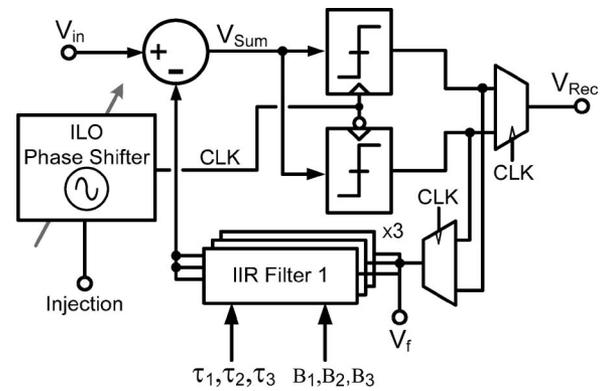
Fig. 8. Fabricated DFE/ILO block diagram.
