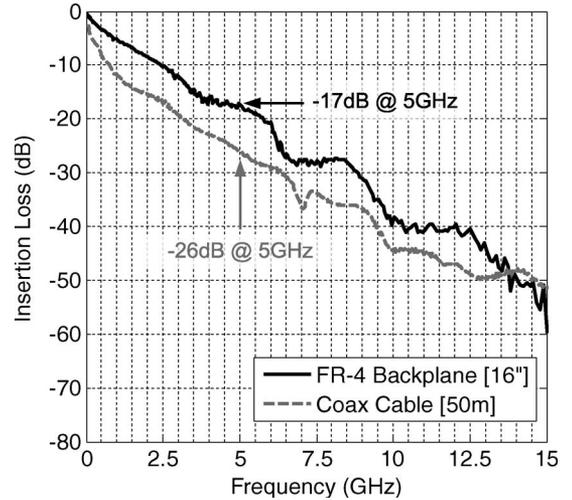
Fig. 4. Measured channel insertion loss.
