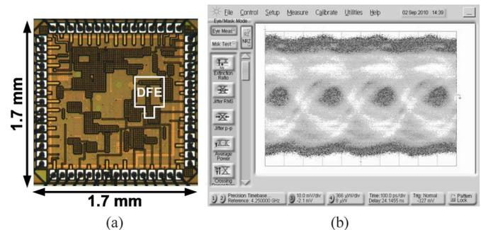
Fig. 10. Chip die photo and input eye diagram. (a) Chip die photo. (b) Measured input eye diagram.
