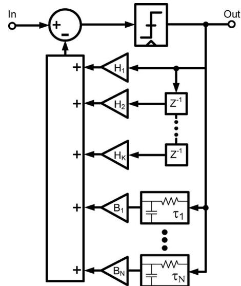
Fig. 1. Generic DFE architecture consisting of  $K$  discrete-time taps and  $N$  continuous-time IIR filters.
