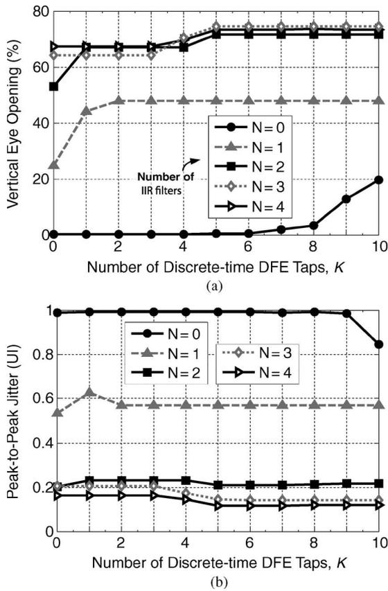
Fig. 7. Simulated DFE architectures at 10 Gb/s (coax cable). (a) Coax cable (50 m) simulated vertical eye opening. (b) Coax cable (50 m) simulated peak-to-peak jitter.
