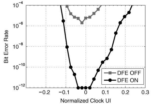
Fig. 12. Measured 3.7 Gb/s Bathtub Curve.
