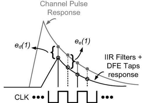
Fig. 3. Channel and DFE feedback pulse response.
