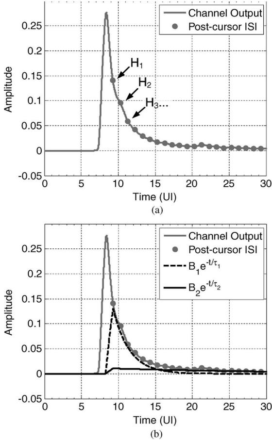
Fig. 2. Pulse response for DFEs employing different number of discrete-time taps and/or IIR filters. (a) Conventional discrete-tap DFE,  $K = 10$ ,  $N = 0$ . (b) 2-IIR filter DFE,  $K = 0$ ,  $N = 2$ .
