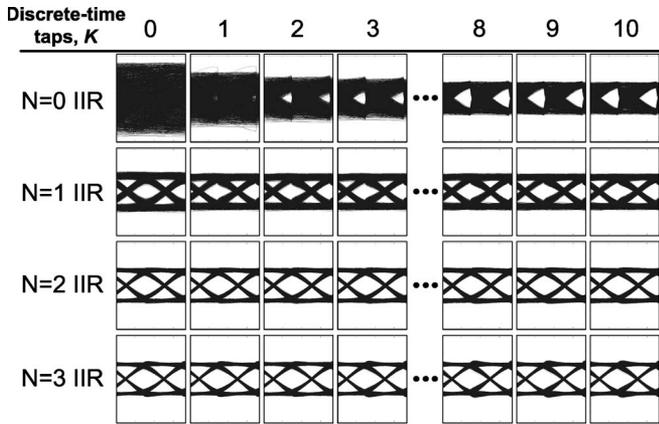
Fig. 5. Simulated eye diagrams for various DFE Architectures.
