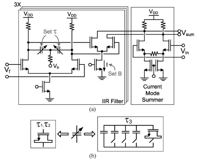
Fig. 9. DFE IIR filter and varactor implementation. (a) IIR filter and current mode summer circuit implementation. (b) Two different varactor implementations.
