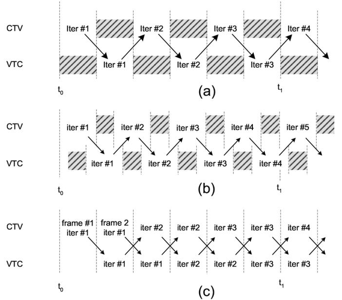
Fig. 4. Timing diagram for the message-passing algorithm. (a) Conventional. (b) Overlapped message passing [17]. (c) Block interlacing.
