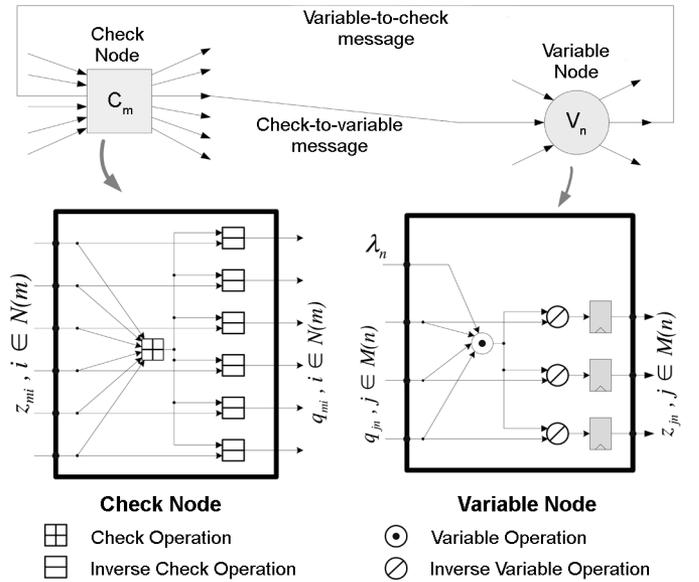
Fig. 1. Conventional fully parallel message-passing LDPC decoder with generic functions for check and variable nodes.
