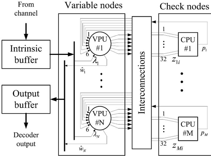
Fig. 5. Top level block diagram for the fully parallel (2048, 1723) LDPC decoder with half broadcasting. ( $N = 2048$ ,  $M = 384$ ).
