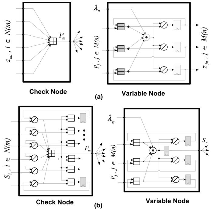
Fig. 2. (a) Half-broadcast architecture. The check node  $c_m$  broadcasts a single message,  $P_m$ , to all neighboring variable nodes. (b) Full-broadcast architecture. The check node  $c_m$  broadcasts  $P_m$  to the neighboring variable nodes. The variable node  $v_n$  broadcasts  $S_n$ .
