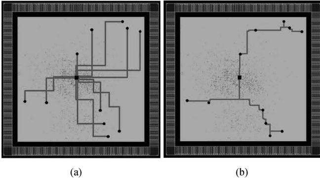
Fig. 3. Routed nets for one check node output highlighted in a fully parallel LDPC decoder layout: (a) without broadcasting and (b) with broadcasting.
