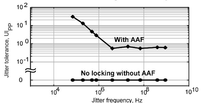
Fig. 1. Simulated Jitter Tolerance of the CDR in [5] with/without AAF
