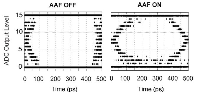
Fig. 8. Digital eye-diagrams with AAF OFF/ON.
