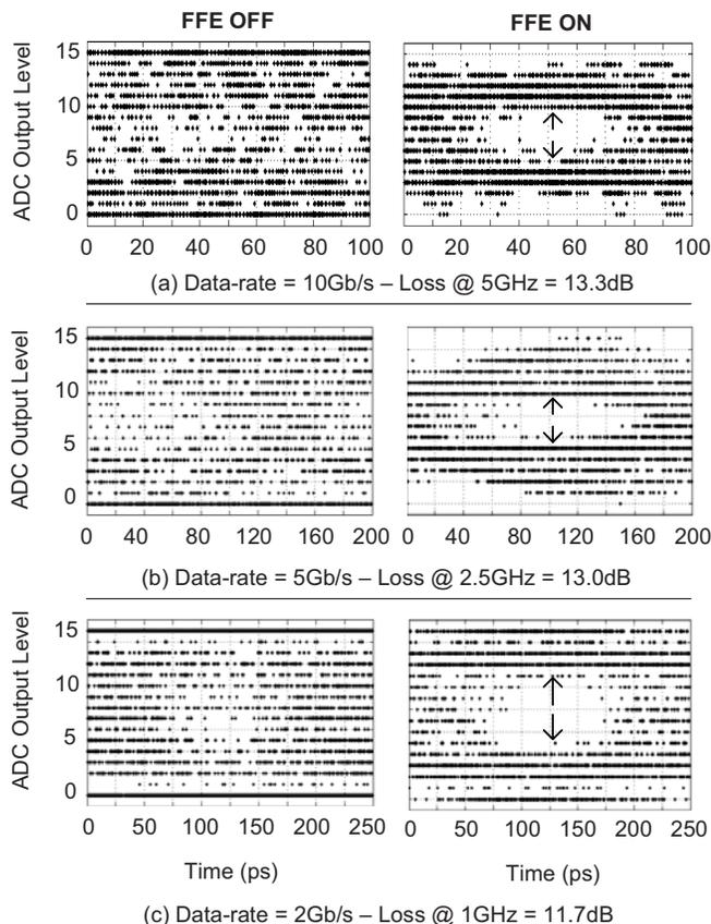
Fig. 9. Digital eye-diagrams with FFE OFF/ON.
