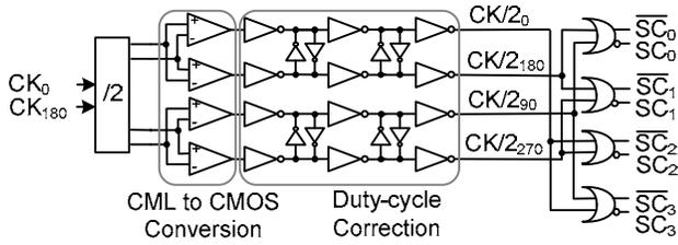
Fig. 5. The clock generation circuitry.
