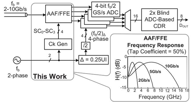
Fig. 2. Proposed analog front-end for a 2x blind ADC-Based RX.
