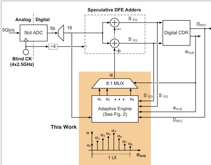
Figure 25.1.1: Adaptive DFE for 2x blind ADC-based receiver.
