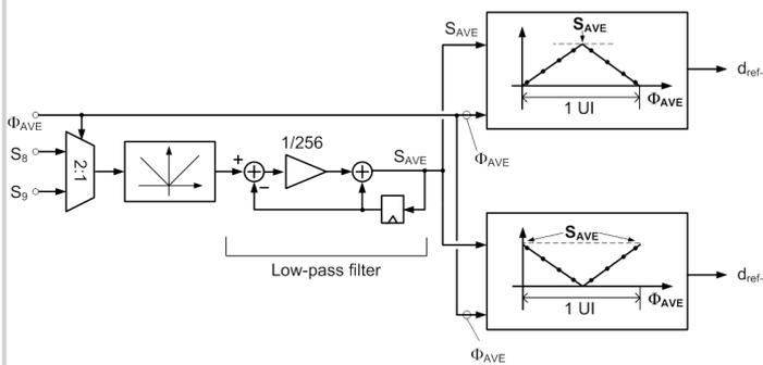
Figure 25.1.3: Desired waveform generator: desired levels produced based on average phase.
