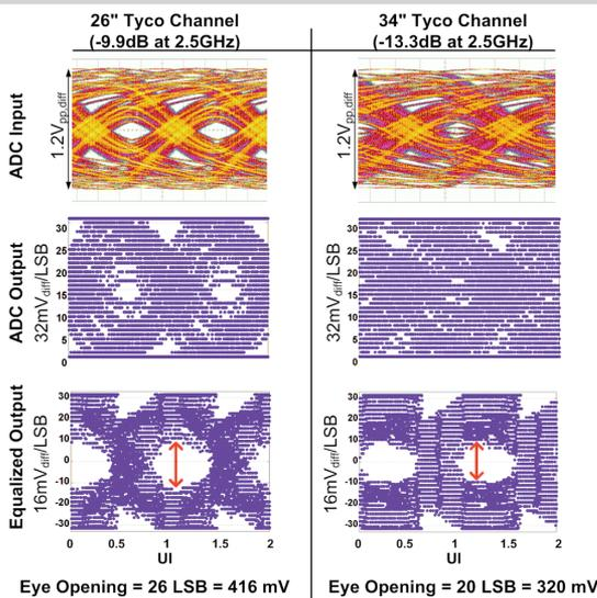
Figure 25.1.5: Measured eye diagrams for a 26" and 34" Tyco channels.
