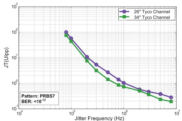
Figure 25.1.6: Measured jitter tolerance for 26" and 34" Tyco channels.
