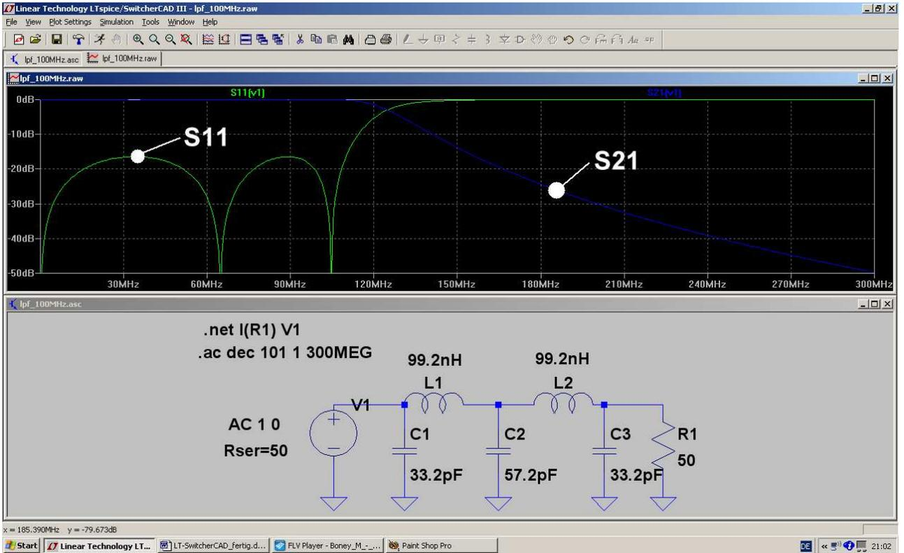
For a separate presentation of the two S-parameters right click on the diagram and choose
