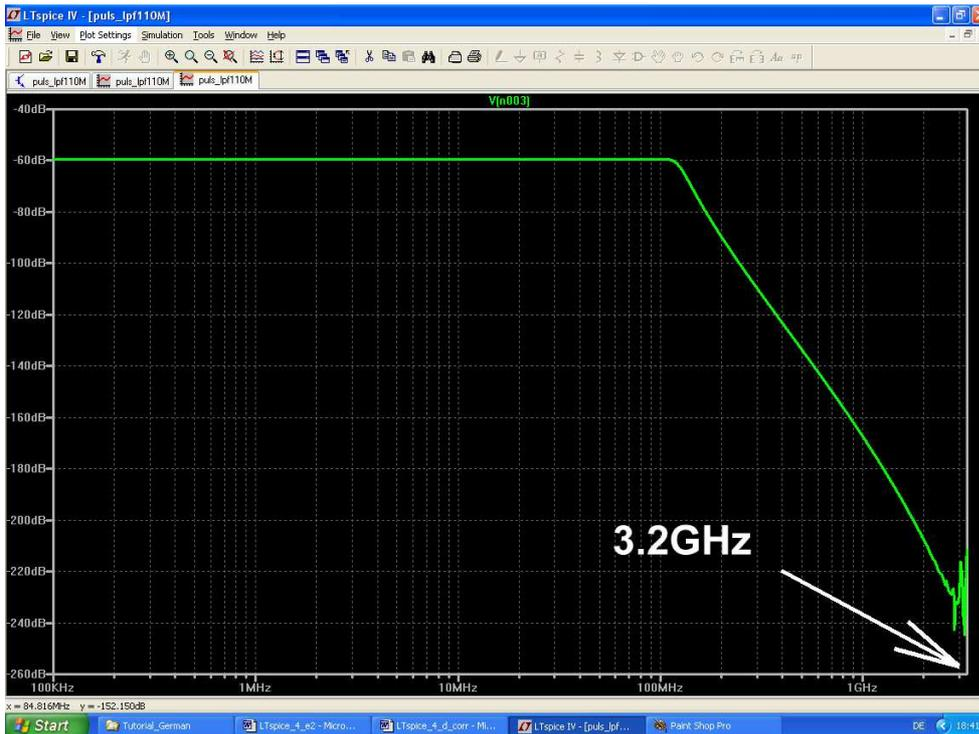
Reducing the number of samples for the FFT will also reduce the simulation accuracy AND the the maximum frequency presented in the diagram from 52.5GHz to 3.2GHz
