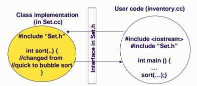
Bottom Line: Code is spread out over several .cc and .h files Changes to implementation are transparent to user Only the file that changes needs to be recompiled
