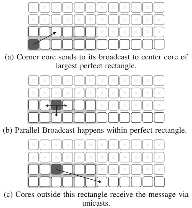
Fig. 12. Optimized Parallel Broadcast with 18 active cores. The maximum perfect rectangle is shown in light grey. Cores not participating in the broadcast are marked with a “x”.
