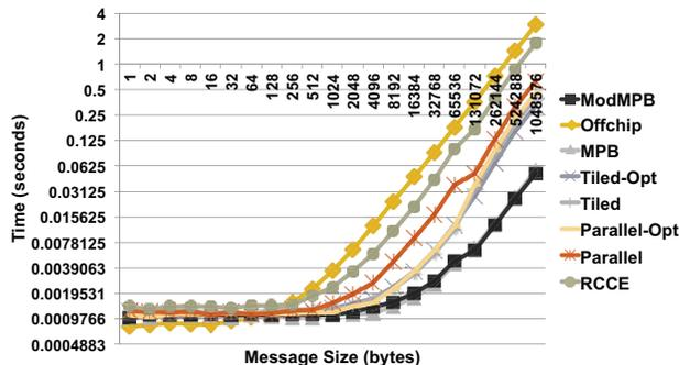
Fig. 9. Microbenchmark results: Broadcast latency when varying message size from 1B to 1MB.
