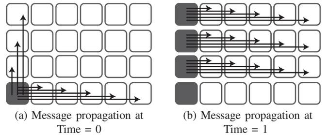
Fig. 7. ModMPB Broadcast Propagation.
