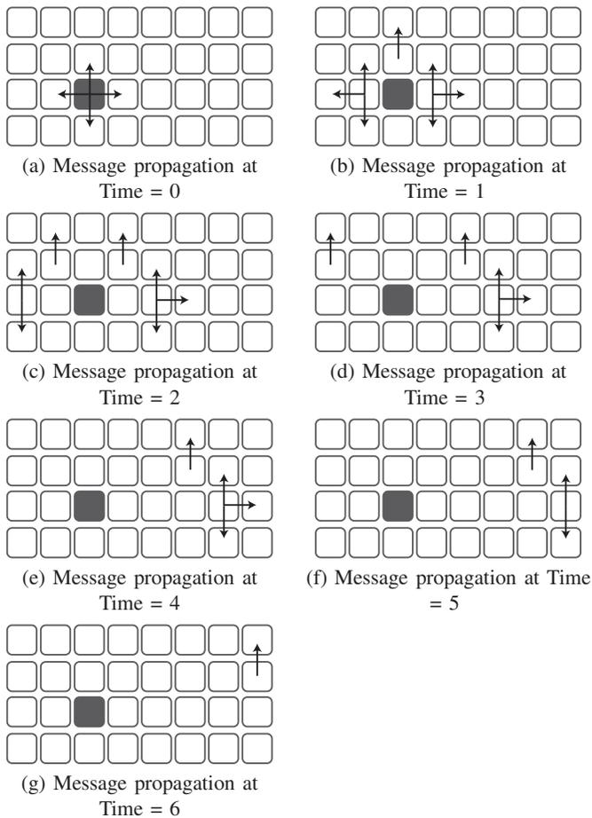
Fig. 2. Parallel Broadcast Propagation. The broadcast source node is shown in grey. The number of cores shown is simply for illustration purposes.
