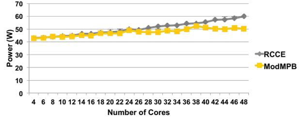
Fig. 17. Power consumption for RCCE and ModMPB broadcasts.
